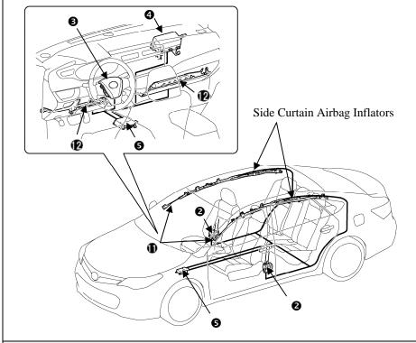
Standard Frontal Airbags, Seat Belt Pretensioners, Knee Airbags, Side Curtain Airbags
