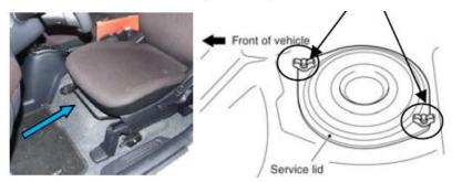
② Pull up the lever of the Service Plug and then remove the Service Plug by pulling upward on the lever.
