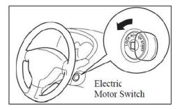
② If it is impossible to turn off the Electric Motor Switch, use needle-nose pliers to remove the Power control unit fuse from the fuse box under the hood. It is the No.7 15A fuse shown in below figure. If you cannot locate this fuse, remove all fuses and relays in the fuse box.
