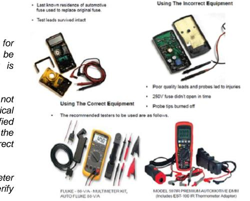
Note The tester is to be checked as per the manufacturers instructions BEFORE and AFTER each measurement taken.
