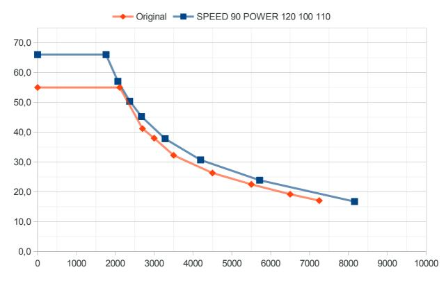
The original power map of the Twizy cuts back torque in the rpm range up to ~61 kph. It contains a nonlinearity, but one that does not look natural: if you take a look at 2700 and 3000 rpm, these do not fit into the overall curve, even if considering efficiency nonlinearity. Also, the mechanical power at the original turning point of 2115 rpm is 12.2 kW instead of the 13 kW. 13 kW will only be available from 5500 rpm upwards.
