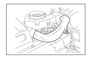
(3) Remove the clip and No. 2 HV battery intake duct with the No. 3 HV battery intake duct.
