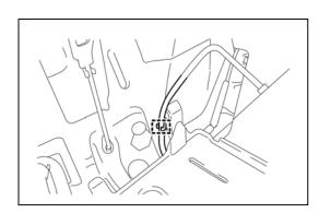
(3) Disconnect the battery pack wire connector and clamp
