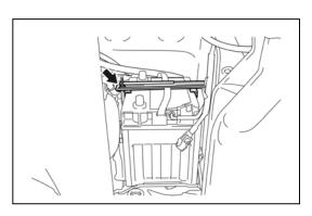
(3) Disconnect the battery ventilation hose and remove the battery
