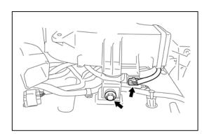
(6) Remove the battery cooling blower assembly as shown in the illustration
