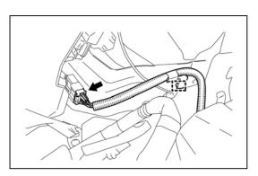
(4) Remove the grommet and hybrid battery hose assembly
