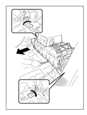
(8) Using a tire lever to hold up the HV battery, insert a wooden block or equivalent as shown in the illustration
