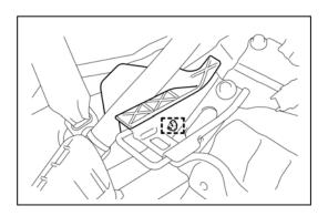
(2) Remove the 2 bolts and child restraint seat anchor bracket sub-assembly RH.
