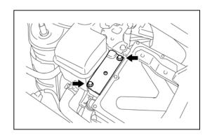
8. Check the voltage at the terminals in the inspection point in the power control unit.
