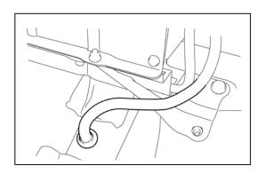
(5) Remove the 4 bolts from the HV battery
