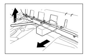
(9) Pull the HV battery together with the cardboard toward the rear of the vehicle
