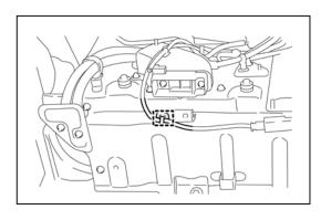
(11) Using a suitable adaptor such as a rope, remove the HV battery while tilting the HV battery
