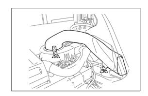
(2) Remove the clip and No. 4 HV battery intake duct.
