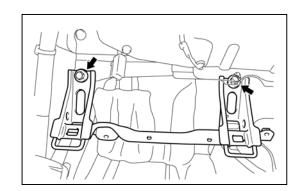
29. Remove the HV battery
