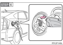
Insert the charging cable into the charging inlet.
