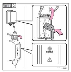
Insert the charging cable into the outlet of the external power source.
