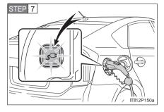
Confirm that the charging indicator is illuminated. (When the charging timer function is in use, the light will turn off several seconds after illuminating.)
