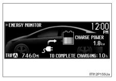
If the "POWER" switch is turned to ON mode during charging, the current charging status and the amount of time needed until charging is complete will be displayed on the energy monitor.
