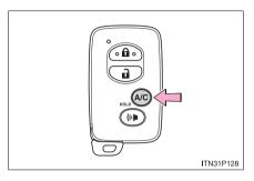
Press and hold the A/C to operate the Remote Air Conditioning System.
