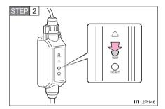
Press the test button on the CCID (Charging Circuit Interrupting Device).
