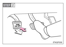
Release the parking brake and your foot from the brake pedal gradually, and then start the vehicle by depressing the accelerator pedal gently.
