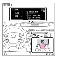
Stop the vehicle and press the charging timer switch.
