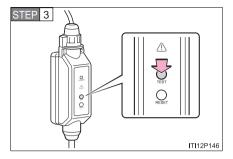
Press the test button on the CCID (Charging Circuit Interrupting Device) to check that the electrical leakage detection function operates properly.
