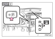
Shift the shift position to P. Check that the shift position indicator on the instrument cluster is in P, and release the brake pedal gently after applying the parking brake.
