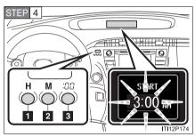
Adjust the set time using the time adjustment button.
