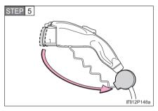
Remove the charging connector cap.
