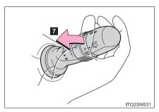
Washer/wiper dual operation Wipers operate automatically.
