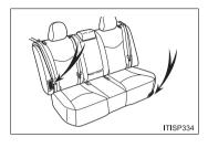
There are air intake vents on the side of the rear right seatback and on the front corner of the left rear seat cushion for the purpose of cooling the hybrid battery (traction battery). If the vents become blocked, the hybrid battery (traction battery) may overheat, leading to a reduction in hybrid battery (traction battery) output.
