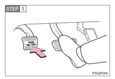
Stop the vehicle completely by depressing the brake pedal and then apply the parking brake.
