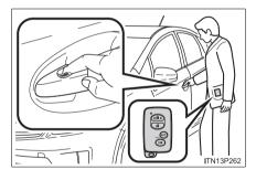
Touch the lock sensor (the indentation on the upper part of the door handle) to lock the doors.
