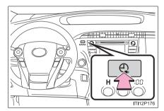
If the charging timer switch is pressed while the charging timer indicator is illuminated or flashing, the charging timer function will be canceled. Charging will commence immediately if the charging cable is connected to the vehicle.
