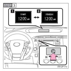
Press the charging timer switch to select a setting mode.
