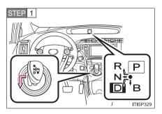
When the "READY" indicator comes on, shift the shift position to D or R and release it with the brake pedal depressed. The D or R position is selected and the lever returns to its home position. Confirm which position is selected with the shift position indicator in the instrument cluster.
