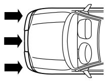
near-frontal collisions, not rollover, side-impact, or rear-impacts unless the collision causes sufficient longitudinal deceleration.
