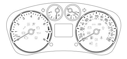
**Speedometer:** Indicates the current vehicle speed.
