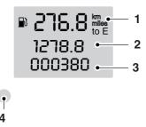
Distance to empty: Registers the approximate distance the vehicle can travel before refueling is necessary.
