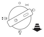
Pull the headlamp control towards you until the second detent is felt to turn the rear fog lamp on. The rear fog lamp indicator light  $0 \neq$  will illuminate.
