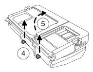
When raising the seatback(s), make sure the lever is locked and you hear the seat latch into place.
