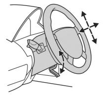
**WARNING:** Never adjust the steering wheel when the vehicle is moving.
