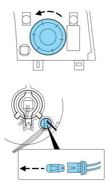
3. Remove the bulb and the bulb socket.
