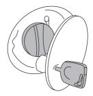
If the check fuel cap light  $\mathbf{k}^{\bullet}$  comes on, the fuel filler cap may not be properly installed. The light can come on after several driving events after you've refueled your vehicle.
