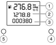
1. **Distance to empty / clock:** Registers the approximate distance the vehicle can travel before refueling is necessary. Clock shows the current set time.
