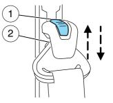
To adjust the belt upward, slide the adjuster up. You do not need to push the button to slide the adjuster upwards. Pull down on the height adjuster to make sure it is locked in place.
