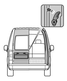
**Note:** The dual rear doors should be closed before driving your vehicle. Leaving the doors open could cause serious damage to them and their components. The left door must be closed first.
