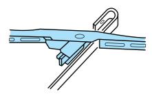
Replace wiper blades at least once per year for optimum performance. Poor wiper quality can be improved by cleaning the wiper blades and the windshield. Refer to *Windows and wiper blades* in the *Cleaning* chapter.
