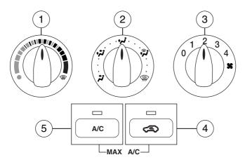
1. **Temperature control:** Controls the temperature of the airflow in the vehicle. For optimum defrosting performance, set the dial to the defrost symbol  $\sqrt{44}$ .
