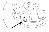
your tires serviced by an authorized dealer. The tire pressure should be checked periodically (at least monthly) using an accurate tire gauge, refer to *Inflating your tires* in this chapter.
