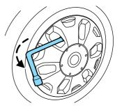
3. Loosen each wheel lug nut one-half turn counterclockwise but do not remove them until the wheel is raised off the ground.
