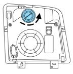
3. Pull the bulb straight out of the socket.
