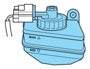
immediately. If the brake fluid level falls below the MIN line, a brake warning lamp will come on.
