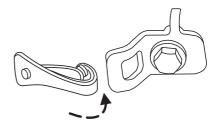
If the tether strap is clipped incorrectly, the child safety seat may not be retained properly in the event of a collision.
