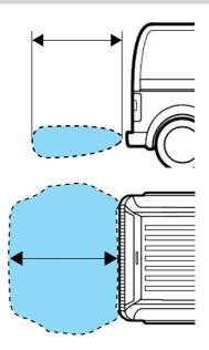
Keep the RSS sensors (located on the rear bumper/fascia) free from snow, ice and large accumulations of dirt (do not clean the sensors with sharp objects). If the sensors are covered, it will affect the accuracy of the RSS.
