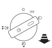
Pull the headlamp control towards you until the first detent is felt to turn the front fog lamps on. The front fog lamp indicator light  $\ddagger$  will illuminate.
