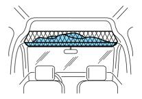
**WARNING:** Do not place heavy or hard objects in the overhead storage, which may fall while driving, and could cause serious injury.
