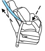
9. Attach the tether strap (if the child seat is equipped). Refer to *Attaching child safety seats with tether straps* later in this chapter.
