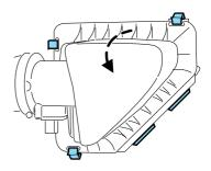
careful not to crimp the filter element edges between the air filter housing and cover. This could cause filter damage and allow unfiltered air to enter the engine if not properly seated.
