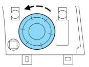
3. Disconnect electrical connector from the bulb.
