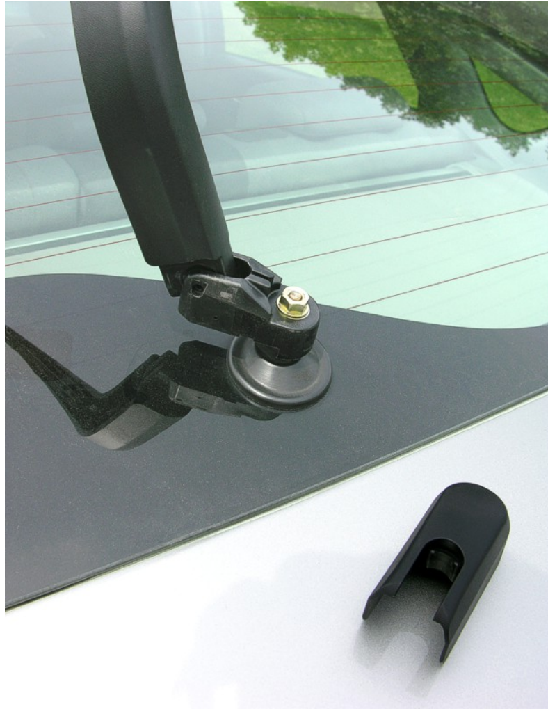
Rear Hatch Wiper (Toyota Part: 85124 - 44140)
