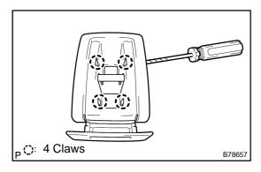
(d) Using a screwdriver, disengage the 4 claws and remove the rear seat back cover.
