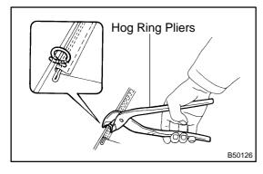
(a) Using hog ring pliers, install the cushion cover to the cushion pad with new hog rings.NOTICE:
