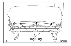
(b) Lift up the seatback cover and remove the 3 hog rings.
