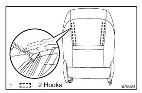
(e) Using a screwdriver, disengage the 2 hooks and remove the seatback cover together with the pad.
