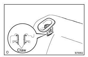
(c) Using a screwdriver, disengage the claws and remove the seatback stop button grommet.
