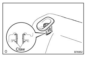
(d) Using a screwdriver, disengage the claws and remove the seatback stop button grommet.
