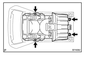
(1) Remove the 4 screws and then the installment panel cup holder.
