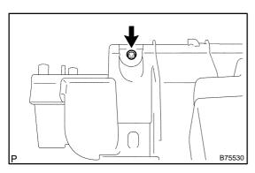
(b) Remove the screw and then the combination meter reflector No.1.
