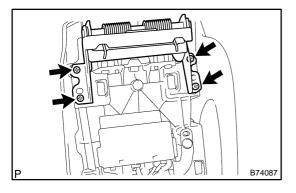
(a) Remove the 4 screws and then the console compartment door sub–assy rear.
