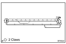
(b) Disengage the 2 claws and then remove the combination meter cover No.1.
