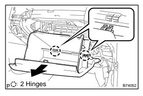
(b) Pull in the direction indicated by the arrow in the illustration and disengage the 2 hinges. Remove the glove compartment door assy.
