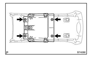
(1) Remove the 4 screws and then the rear console box cup holder.
