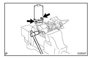
(c) Using SST, turn the steering main shaft 2 or 3 turns at a rate of one turn per second to seat the motor, and temporarily tighten the 2 bolts.
