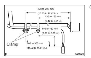
(e) Hold the wire harness for the power steering motor and the torque sensor wire harness with the 2 clamps and vinyl tape as shown in the illustration.
