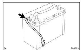
(c) Remove the battery room ventilation hose from the battery.
