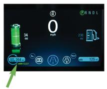
The Total Range indicator displays the total distance that can be driven, based on the combined electric and extended range, before recharging or refueling the vehicle.
