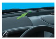
**Note:** Immediately after plugging in, the charging status indicator may be amber for up to five seconds before turning green. The charging system may run fans and pumps when the vehicle is turned off.
