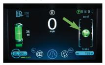
Press the CONFIG button to select the Enhanced Configuration of the instrument cluster to display the efficiency gauge.
