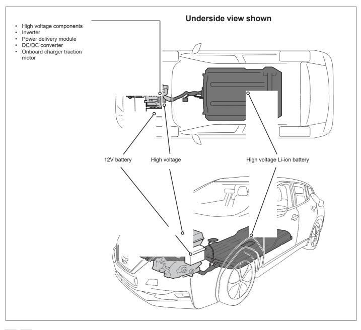
High voltage component or harness (Harness can be cut only after the high voltage system shutdown procedure has been completed.)
