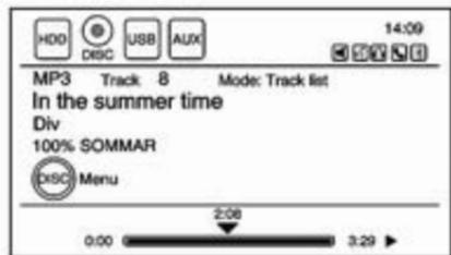
If a disc is already loaded, but currently on a map screen or listening to a different audio source, press the **HDD/DVD/AUX** button to switch to the disc source. A track number appears on the display when each track starts to play.
