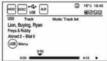
The USB icon displays when the USB device is connected.
