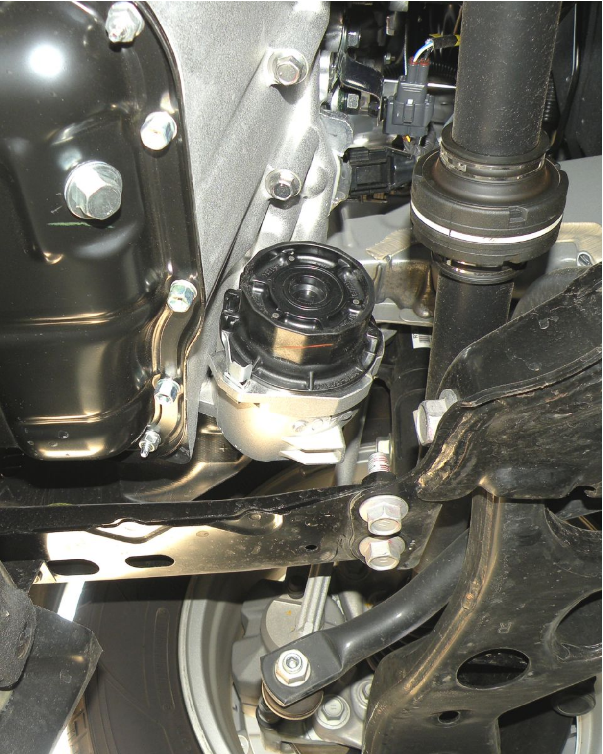
The oil filter-cap is located slightly above and behind the oil pan on passenger side of the Prius. It's the round black object in the center of the photo above.
