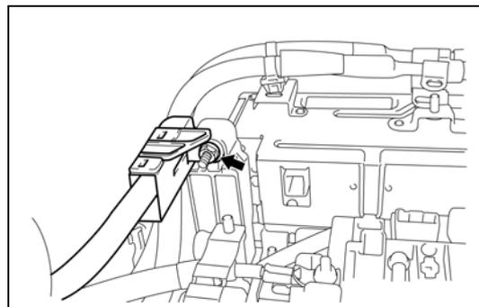
24. Remove the No. 3 hybrid battery exhaust duct.
