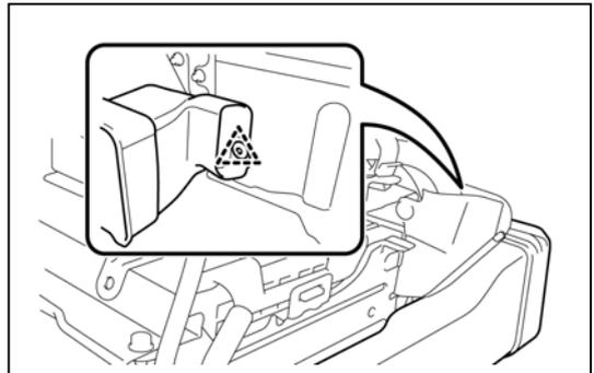
27. Remove the child restraint seat anchor bracket sub-assembly LH
