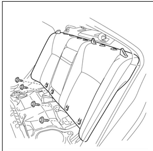
(2) Disengage the 3 hooks and remove the rear seatback assembly.
