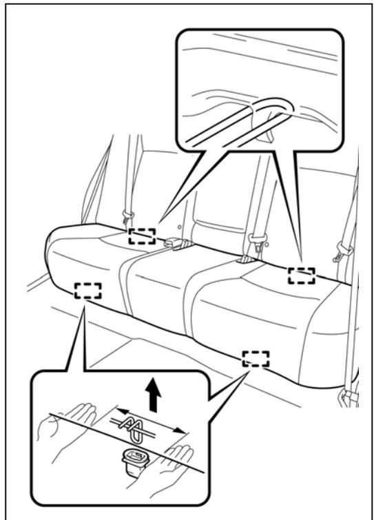
10. Disengage the claw to open the 3 caps of the rear seat shoulder belt guide.
