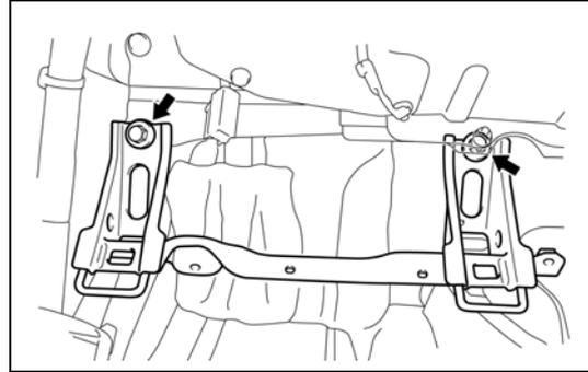
29. Remove the HV battery
