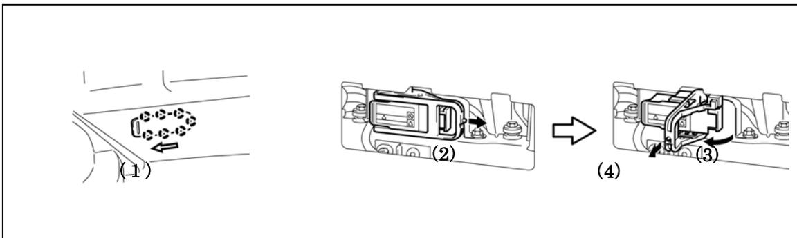
6. Remove the cool air intake duct seal
