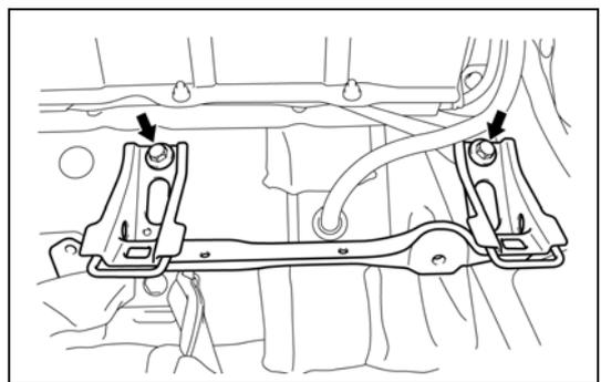
28. Remove the child restraint seat anchor bracket sub-assembly RH
