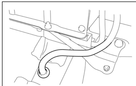
(5) Remove the 4 bolts from the HV battery
