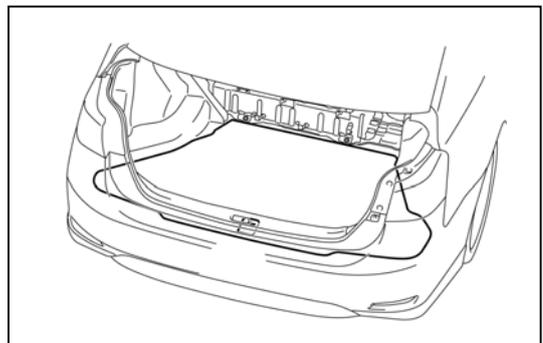
(7) Use a tire lever from the cabin side to lift the HV battery up over the tabs on the body
