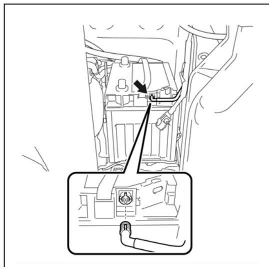
19. Remove the battery cooling blower assembly.
