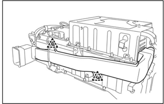
25. Remove the No. 2 hybrid battery exhaust duct
