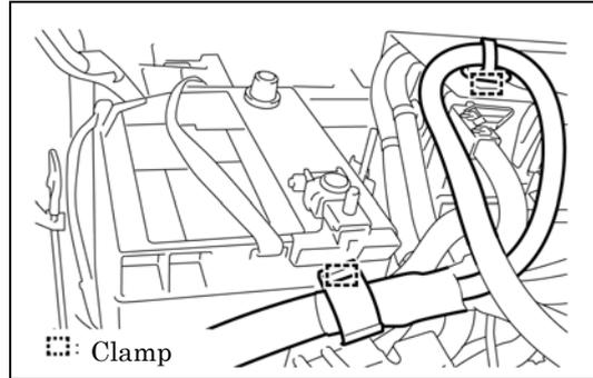
21. Remove the No. 4 hybrid battery shield panel.
