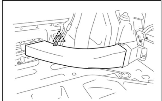
26. Remove the No. 1 hybrid battery exhaust duct.
