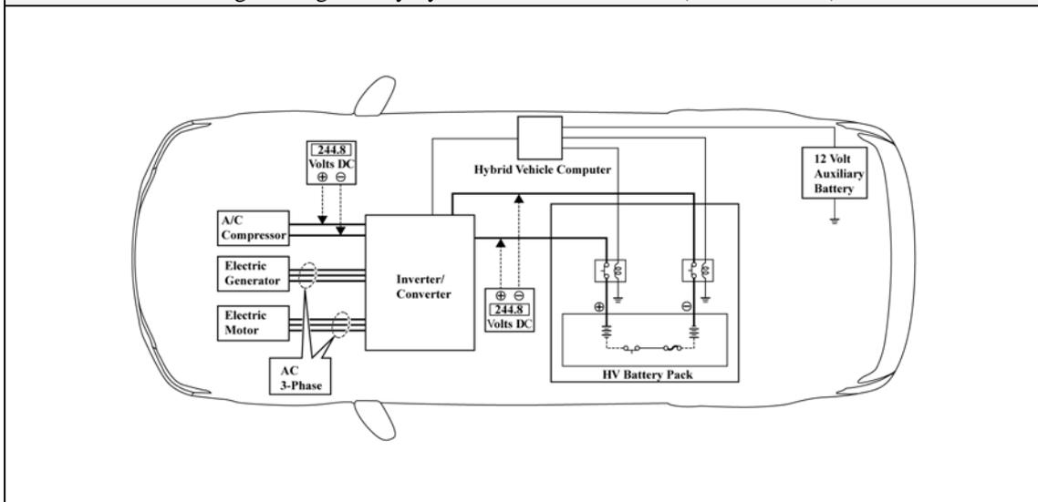
High Voltage Safety System – Vehicle On and Operational (**READY-ON**)
