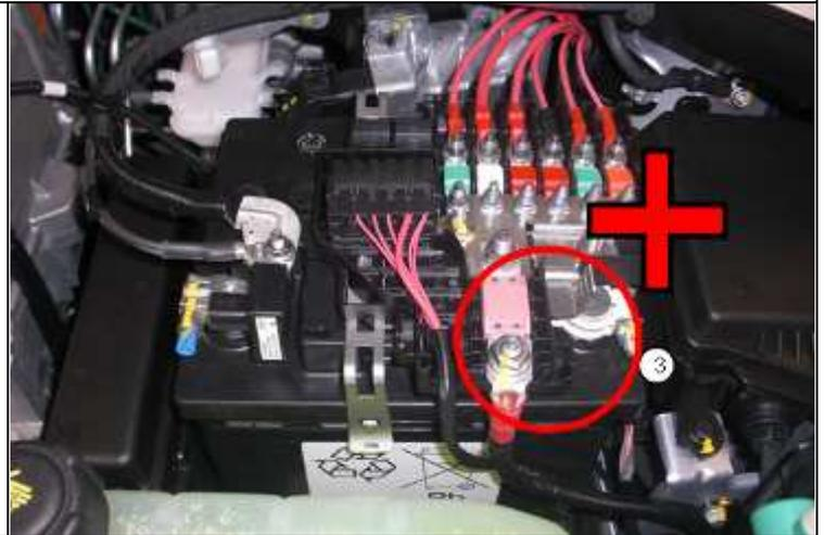
**Nota :** Some electrical features may still be in use. Disconnecting the 12V battery may generate electrical arcs. Be extremely careful during this operation.
