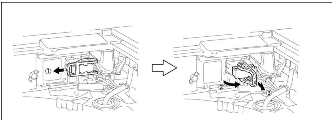
3. Carry the removed service plug grip in your pocket to prevent other staff from accidentally reinstalling it while you are dismantling the vehicle.
