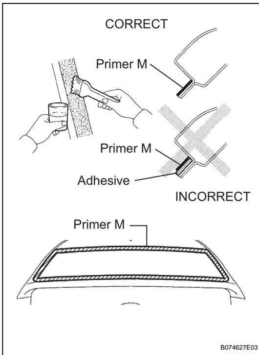
(b) Using a brush or sponge, coat the edge of the glass and the contact surface with Primer G.
