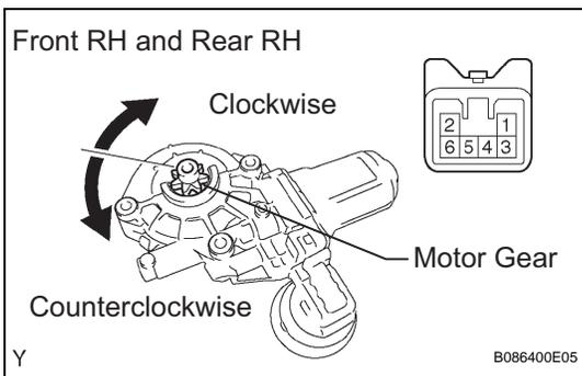
**4. INSPECT POWER WINDOW REGULATOR MOTOR ASSEMBLY (for Front RH and Rear RH)**
