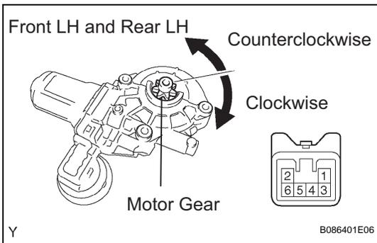
**3. INSPECT POWER WINDOW REGULATOR MOTOR ASSEMBLY (for Front LH and Rear LH)**
