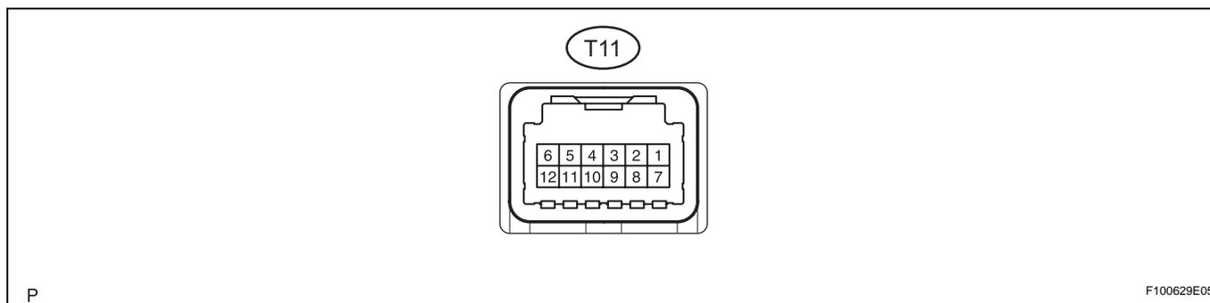
(a) Measure the voltage of the connector.
