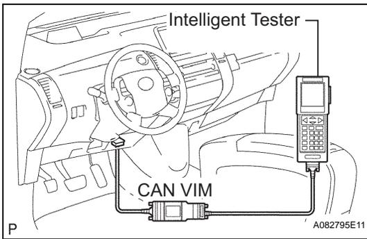
**2. CHECK DTC (USING INTELLIGENT TESTER)**
