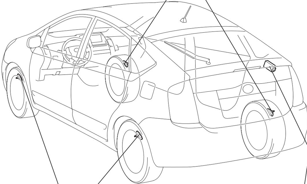
TIRE PRESSURE WARNING VALVE AND TRANSMITTER
