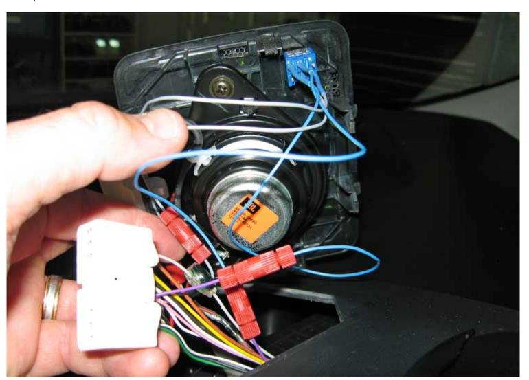
Next I popped a sister switch into the other corner of the speaker grille, and I liked this better. Reverse camera on the left, speed wire interrupt on the right.
