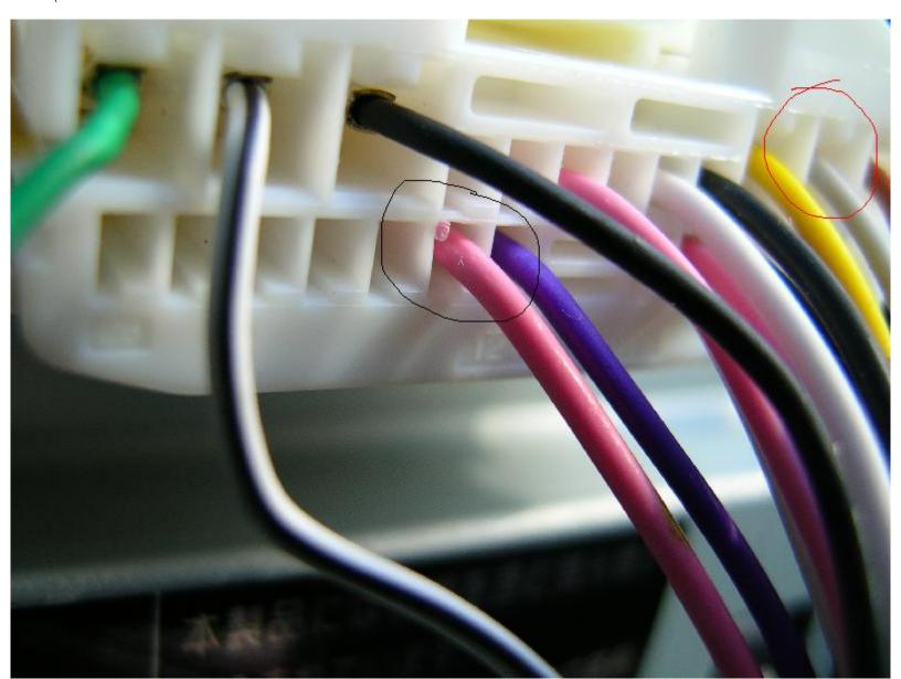
My first attempt was to follow Keydiver's example and use an DPDT on-off-on switch to allow our three situations: All factory connections - speed wire interrupt - reverse video. I wired it all up, and didn't care for it much, though it worked just fine. Here was that attempt where you can see the purple wires attached to the blue wires that go to one pole of the DPDT switch.
