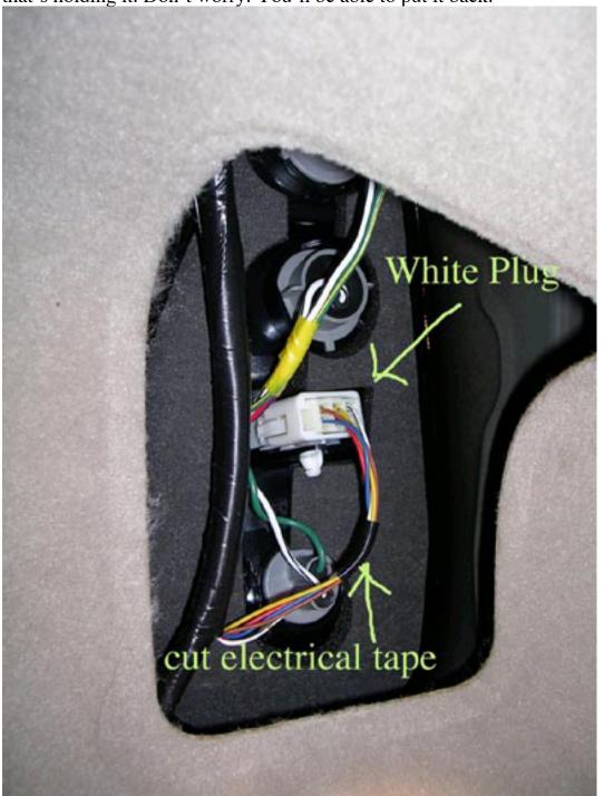
The end of the plug that was facing into the taillight has all of the wires that lead to all of the lights. The end of the plug that was facing out has the wires that come from the car. That's the end you want to work on; the wires that are facing out. There are five wires with electrical tape wrapped around them to keep them together. With the scissors, gently cut the tape along the wires, being careful not to
