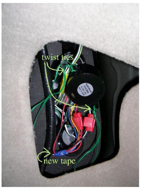
Now turn your car on and put it in reverse. You will year the new buzzer from both the inside and the outside. Replace the access panel.
