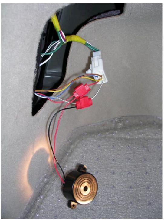
Now take a piece of electrical tape and tape all of the wires together including the buzzer wires. Push the white plug back into place making sure it clips into the black plastic bracket.
