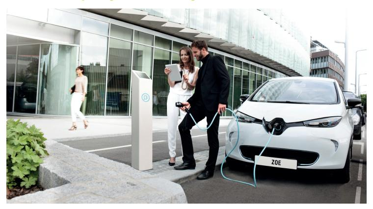
ZOE is the first electric vehicle to be equipped with the Caméléon battery charger. Patented by Renault, this new-generation charger fits beneath the bonnet and is compatible with all power levels up to 43kW. ZOE is consequently able to charge up to 80 percent of the battery's maximum capacity in 30 minutes.
