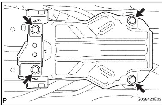
51. REMOVE NO. 1 CONSOLE BOX MOUNTING BRACKET
