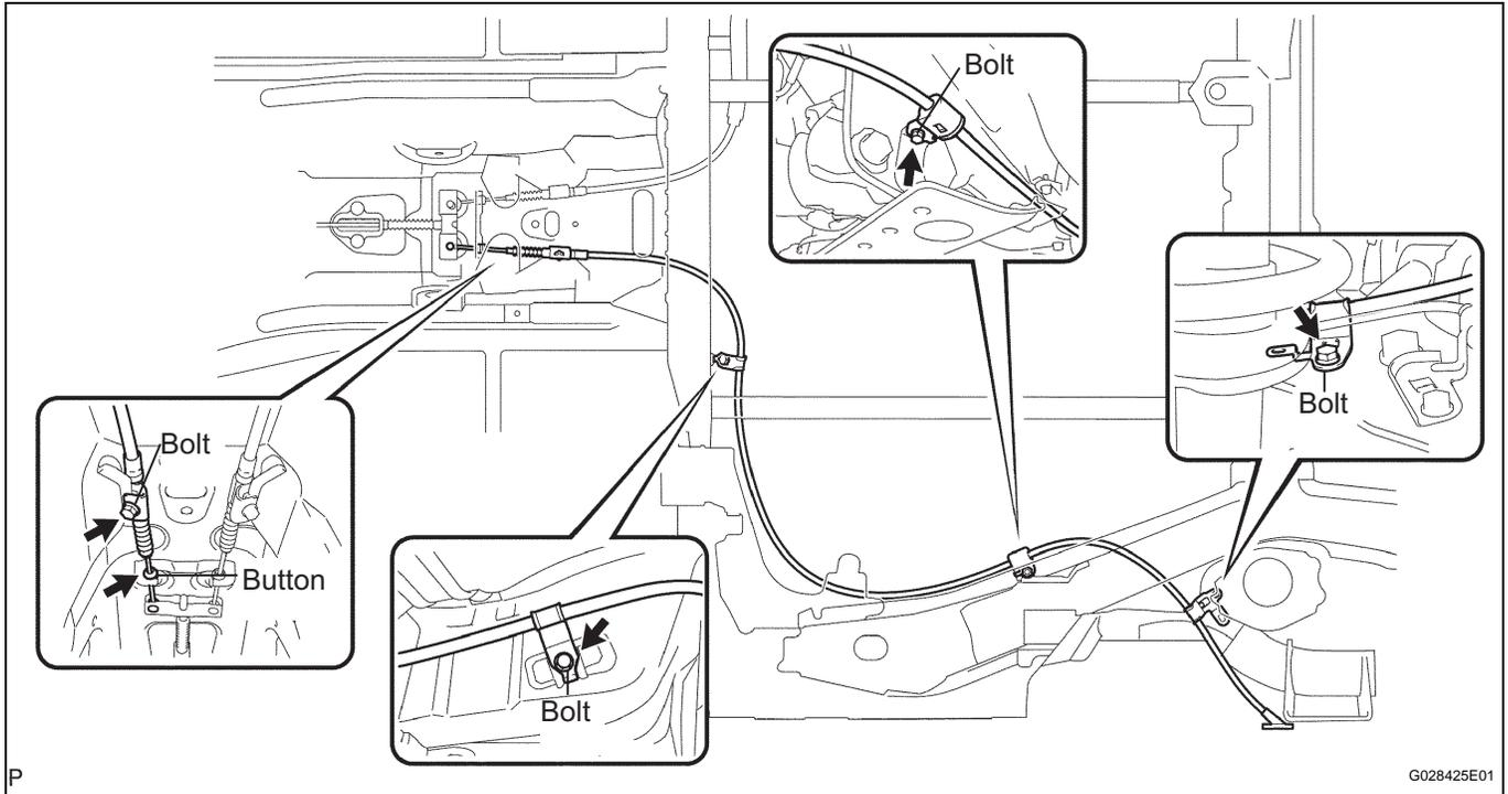
(c) Disconnect the No. 3 parking brake cable from the parking brake equalizer.
