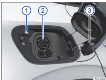
Fig. 147 Behind the charging socket flap at the rear right: charging socket.
