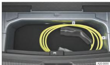
Fig. 151 Under the luggage compartment floor: stowage compartment for the charging cable (schematic diagram).
