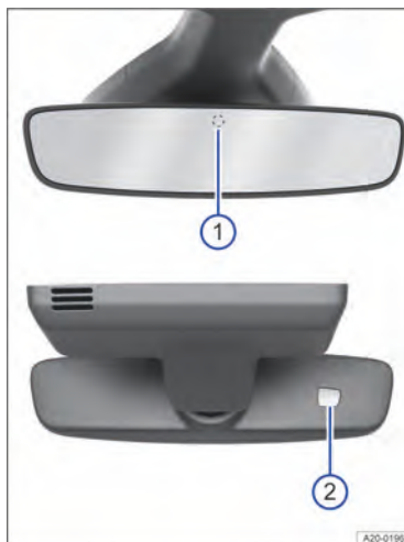
Fig. 94 On the windscreen: automatic anti-dazzle interior mirror.
