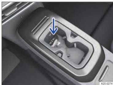
Fig. 99 In the centre console: emergency start function.
