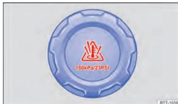
Fig. 180 Under the bonnet: coolant expansion tank cap (illustration).
