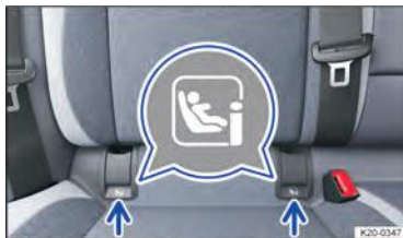
Fig. 44 Markings identifying the i-Size anchor points for child seats on the seats of the rear bench seat.
