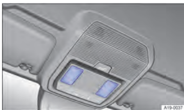
Fig. 90 In the roof console: touch-sensitive reading lights.
