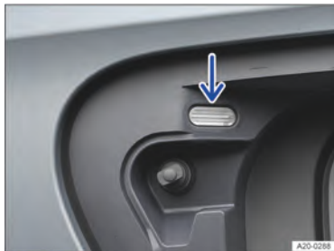
Fig. 148 Behind the charging socket flap: charging process indicator.
