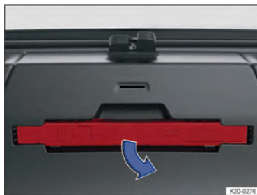
Fig. 50 In the boot lid: holder for the warning triangle.
