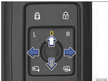
Fig. 95 In the driver door: rotary knob for the exterior mirrors.
