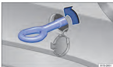
Fig. 172 In the rear bumper on the right: screwing in the towing eye: screwing in the towing eye.
