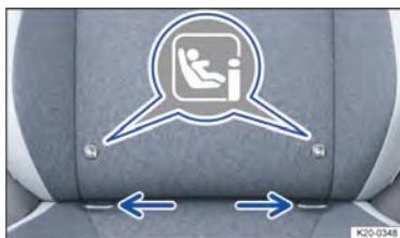
Fig. 45 Markings identifying the i-Size anchor points for child seats on the front passenger seat.
