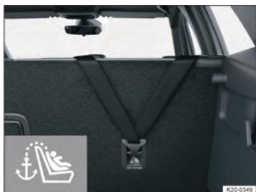
Fig. 47 In the luggage compartment: attached top tether.
