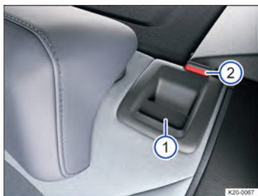
Fig. 77 In the rear seat backrest: release button.
