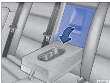
Fig. 134 In the rear seat backrest: opening the load-through hatch.
