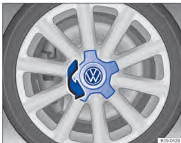
Fig. 188 Removing the centre wheel trim by turning.
