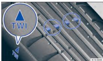
Fig. 185 Tyre tread: tread wear indicators.
