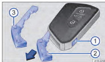
Fig. 54 Vehicle key: releasing the spare key.
