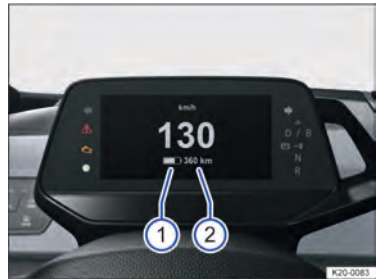
Fig. 11 In the digital instrument cluster: charge level of the high-voltage battery (1) and vehicle range (2).
