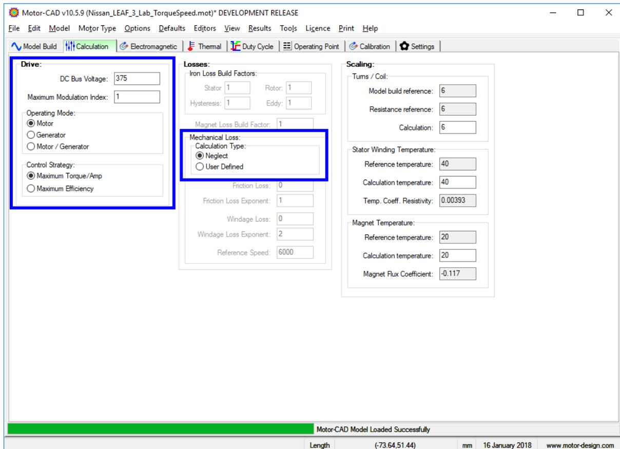
We can now use the **Electromagnetic** tab to calculate the peak torque/speed curve. We set up the options as follows:
