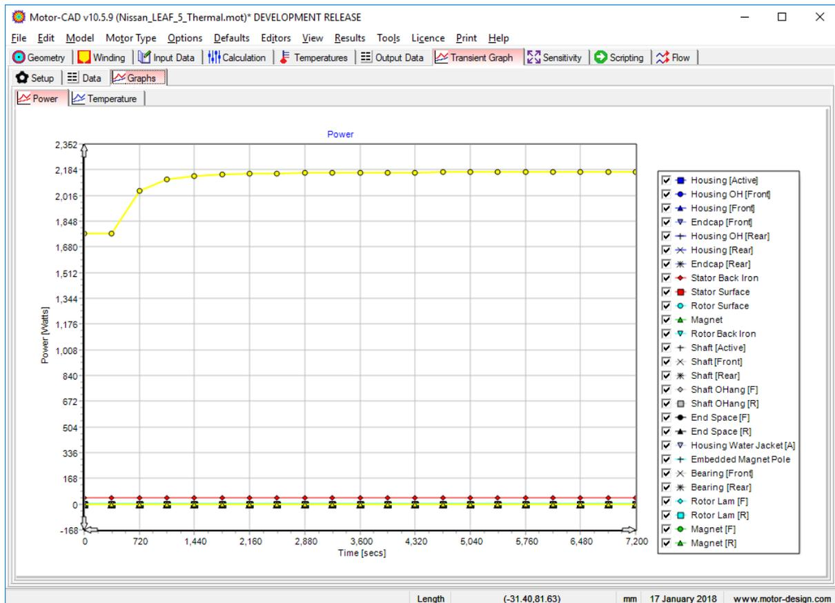
The **Temperatures** -> **Schematic/Radial/Axial** and **Output Data** tabs show the final values at the end of the transient calculation.
