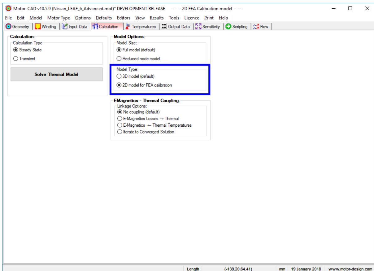
Now solve the model. We notice that the Motor-CAD window caption has been changed to indicate the model is in 2D FEA calibration mode.
