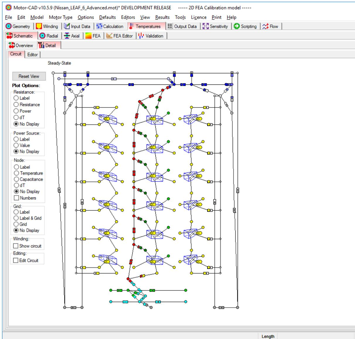
Now we have solved the full thermal circuit using the 2D Fea calibration model we can perform a thermal simulation using thermal FEA. This is solved in the **Temperatures -> FEA** tab. Set the **Area Select** to **Stator** and click **Solve Slot FEA**.
