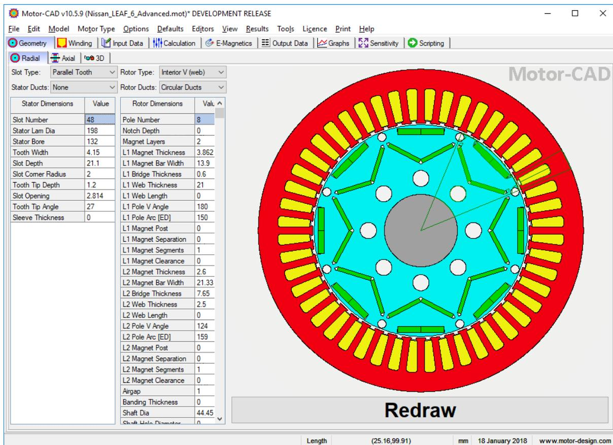
When using imported DXF geometry, it is important that the parameterised Motor-CAD model matches the DXF geometry as closely as possible. This view can be used to modify the model parameters and check how well the geometry matches. The most important parameters are:
