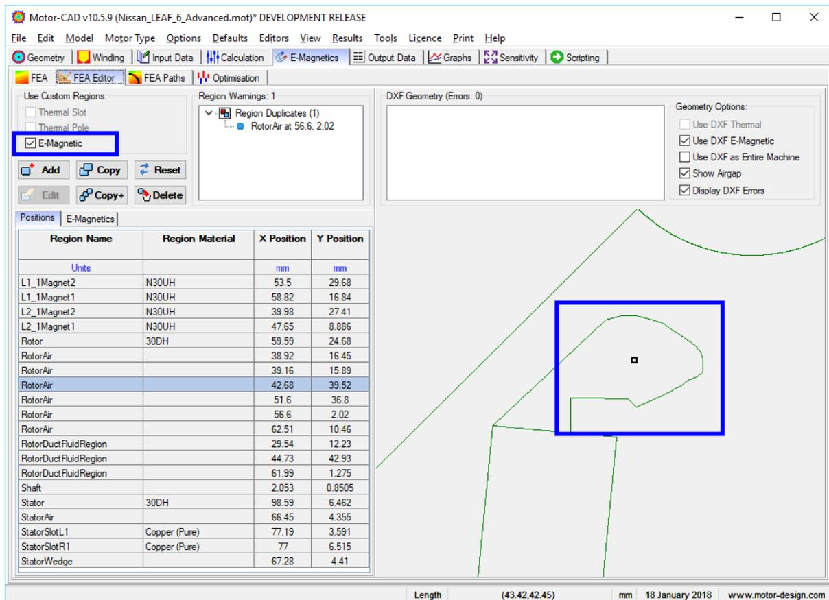
Now that the region has been moved to the correct position, the first warning has disappeared. We repeat the process for the second warning, which refers to the air region at the end of another magnet, so that there are no remaining warnings. We now visually check all regions to make sure they are correct.
