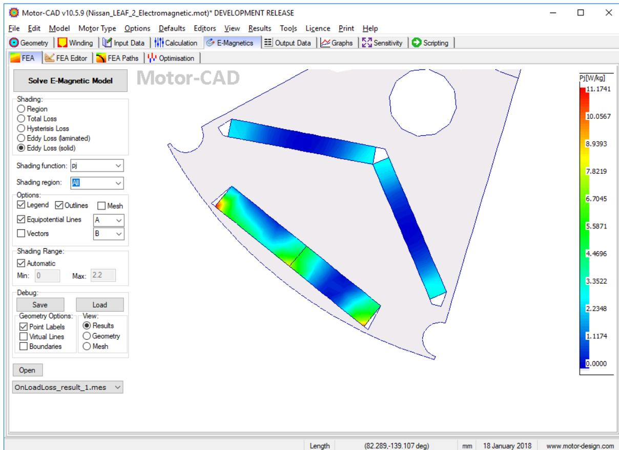
Note that previously calculated flux plots can also be loaded into the FEA viewer using the **Open** button.
