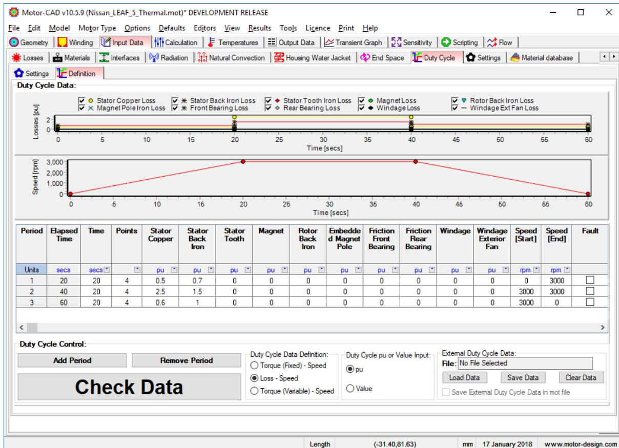
However, when designing a machine it is more usual to define the duty cycle with a torque/speed profile over time. From this an electromagnetic model is used to find the power losses over time, and then this defines the thermal duty cycle. Here the Lab module is a valuable tool since we can very quickly calculate losses over a duty cycle and export the values to the thermal model.
