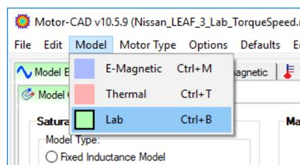
As this is the first time we have viewed the Lab context a single static FEA calculation will be performed to characterise the fixed inductance performance of the machine at a single rotor position. The results can be seen in the **Fixed Inductance Model** section of the interface.
