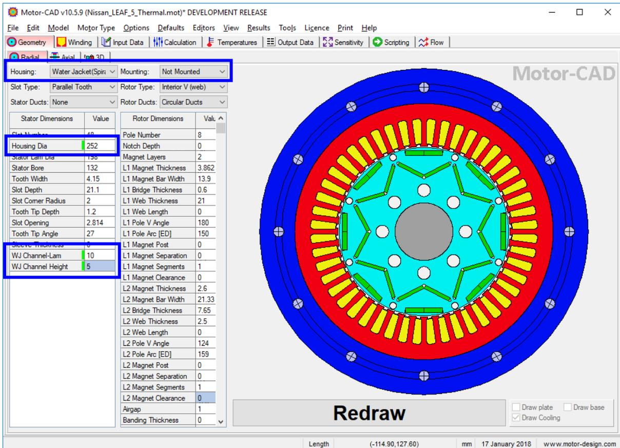
The screenshot shows the Motor-CAD v10.5.9 interface. The 'Radial' tab is active in the 'Geometry' section. The configuration panel on the left shows the following settings:
