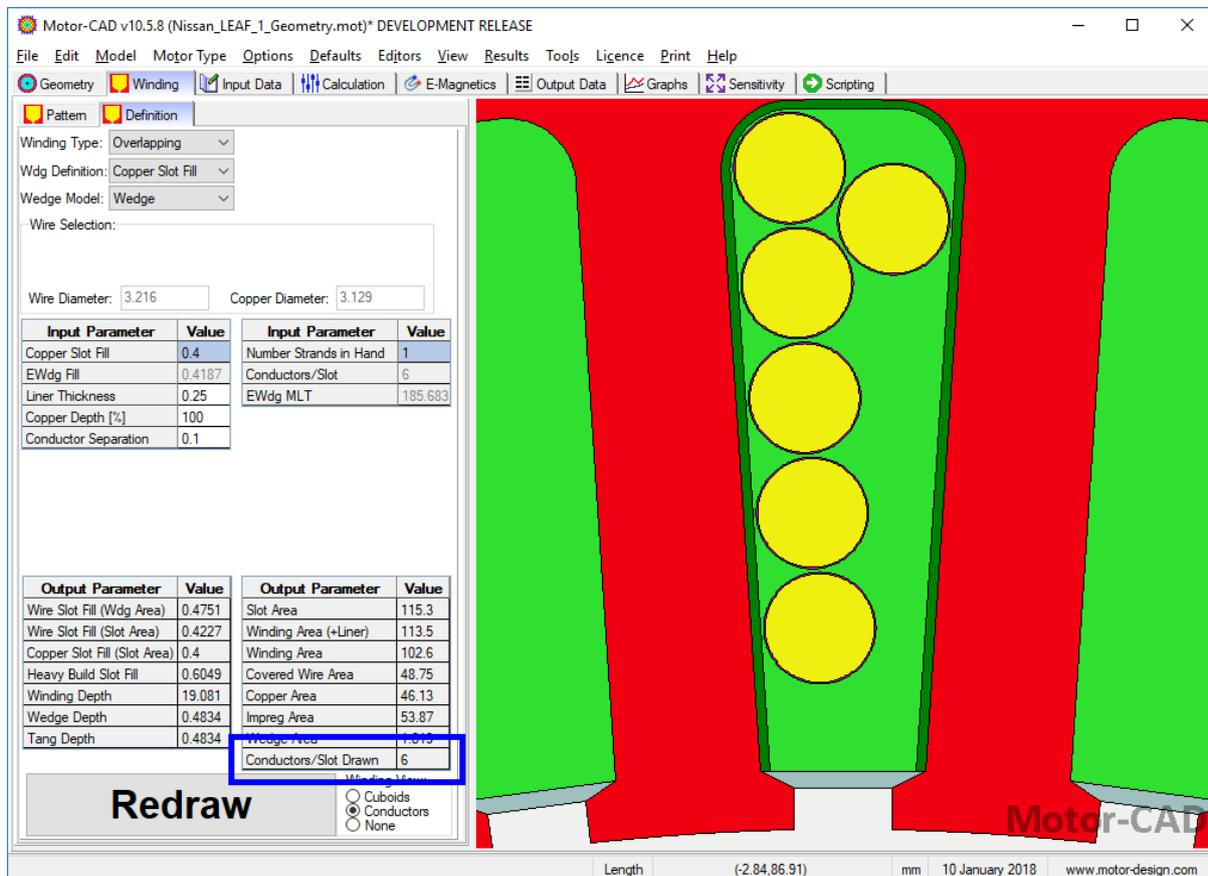
Now define the conductors with the following settings. Note that we have an overlapping winding since this design uses a distributed winding pattern.
