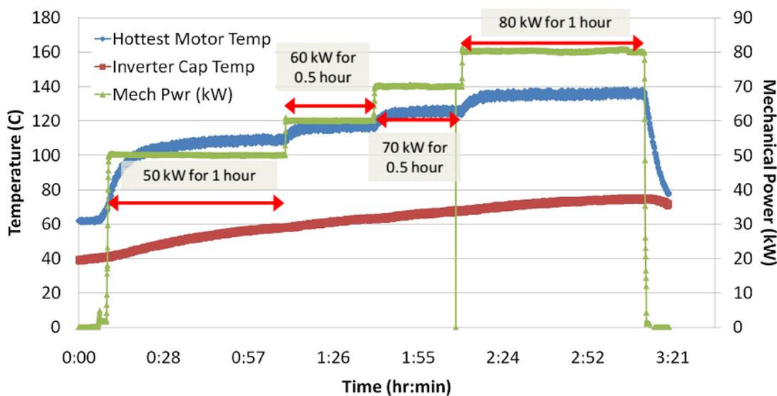
To simulate this test in Motor-CAD, we generate a text file containing the time, torque and speed values for the test. The values must be in SI units (seconds, Nm, rpm) and the file must contain only the numerical values.
