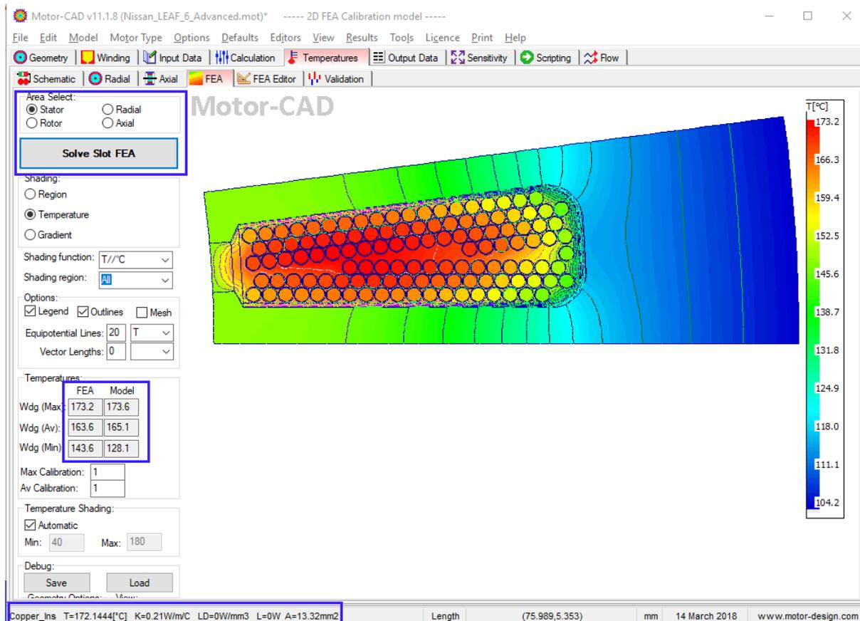
The results usually are well matched between the FEA results and the analytic model. In this example, the difference in the average temperatures is less than 2°C.
