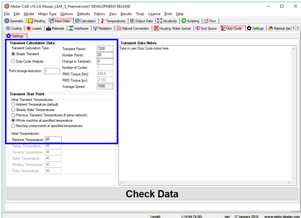
We then go to the **Calculation** tab, set the **Calculation Type** to **Transient** and then **Solve** the model.
