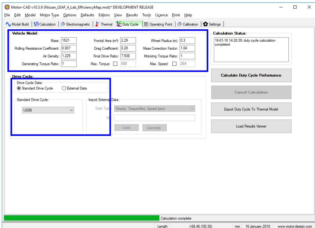
Click **Calculate Duty Cycle Performance** to run the calculation. This should complete within about 2 minutes and by default the viewer shows the torque profile over the cycle.
