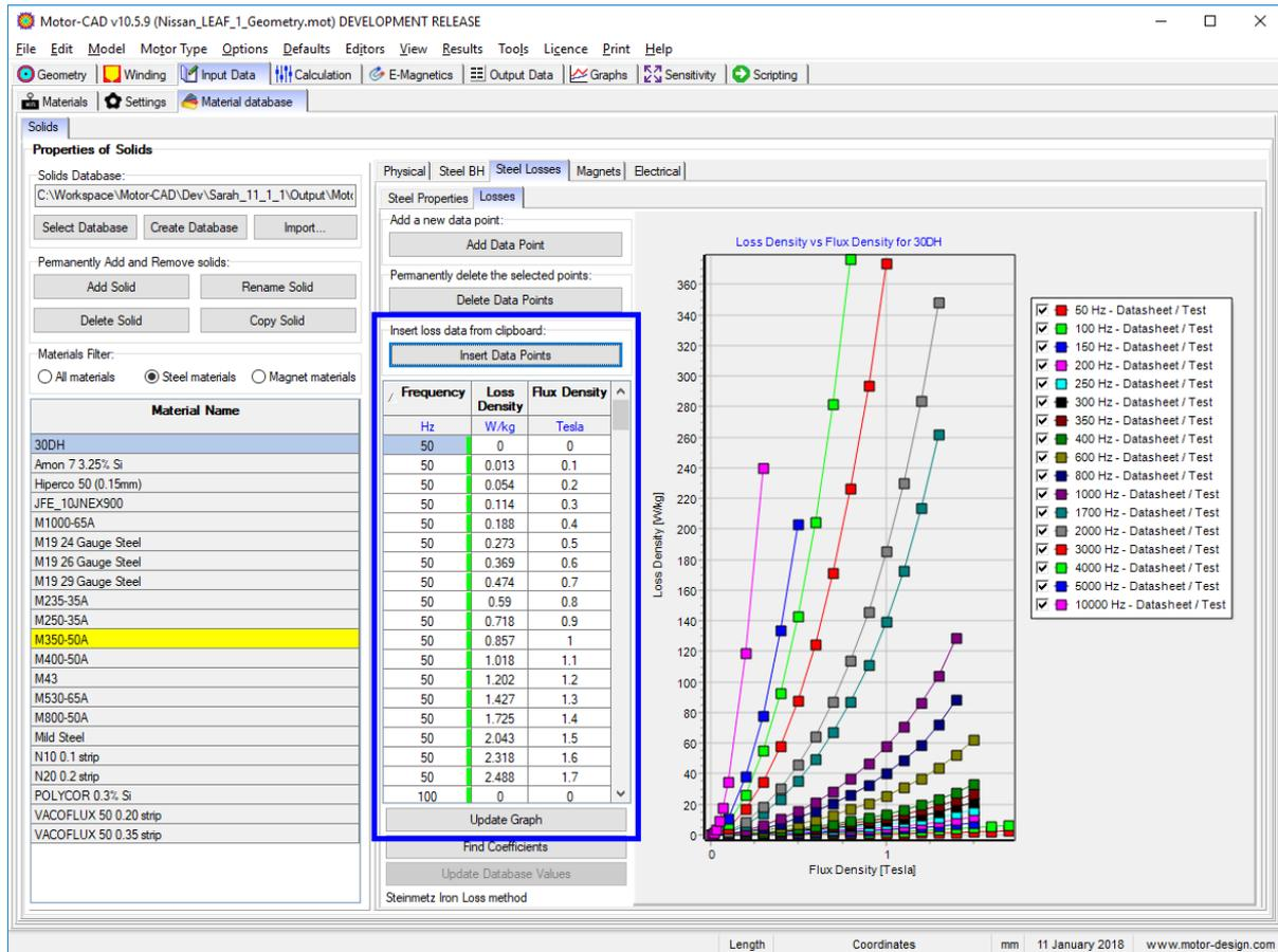
We will now calculate the loss coefficients from the experimental data using Motor-CAD. Click on the **Find Coefficients** button. This uses an iterative curve fitting method to find the iron loss coefficients that best fit the data. This may take several minutes; the progress of the curve fitting is shown in the status bar at the bottom of the Motor-CAD window.
