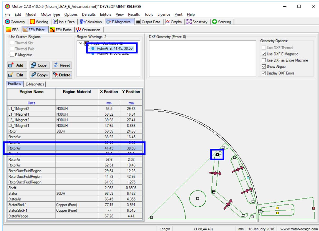
The screenshot shows the Motor-CAD v10.5.9 interface. In the 'Region Warnings' panel, a warning for 'RotorAir at 41.45, 38.59' is highlighted with a blue box. Below this, a table lists various regions with their materials and positions. The 'RotorAir' row at 41.45, 38.59 is also highlighted with a blue box. The main drawing area shows a cross-section of a motor with a blue box around the problematic region marker.
