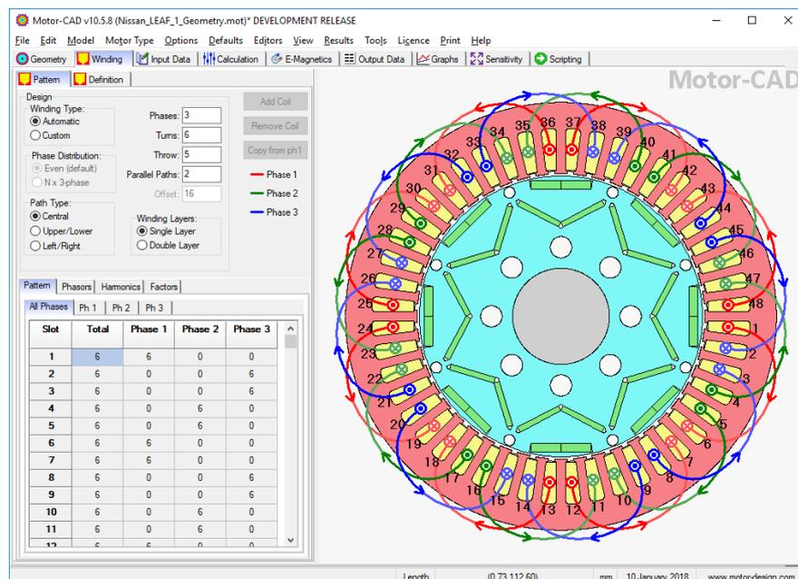
By selecting the **Phasors** tab, we can check that the phasors are 120° apart with equal lengths.
