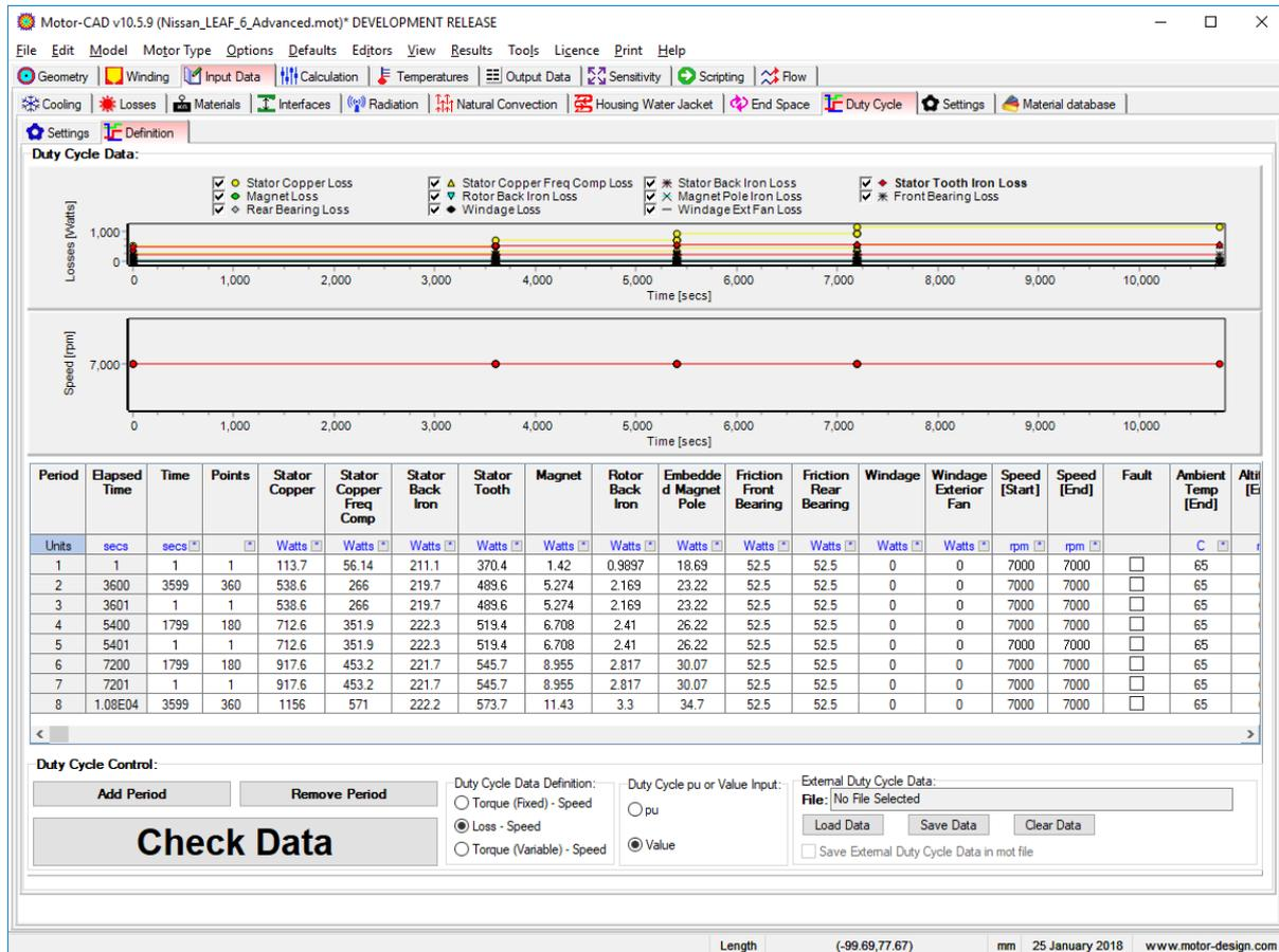
Under **Input Data -> Duty Cycle -> Settings**, we reset the **Number of Cycles** back to 1, since the cycle is only run once for the test.
