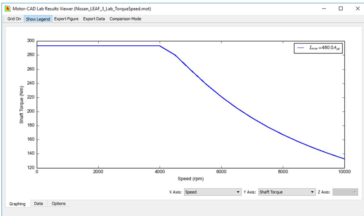
By default the viewer shows the torque vs speed graph, other values can be plotted by changing the **X Axis** or **Y Axis** dropdown, e.g. shaft power vs speed. The raw data can be viewed and exported under the **Data** tab, and the plot can be customised further under the **Options** tab. Exact values at any point can be found by clicking on the graph at the point of interest.
