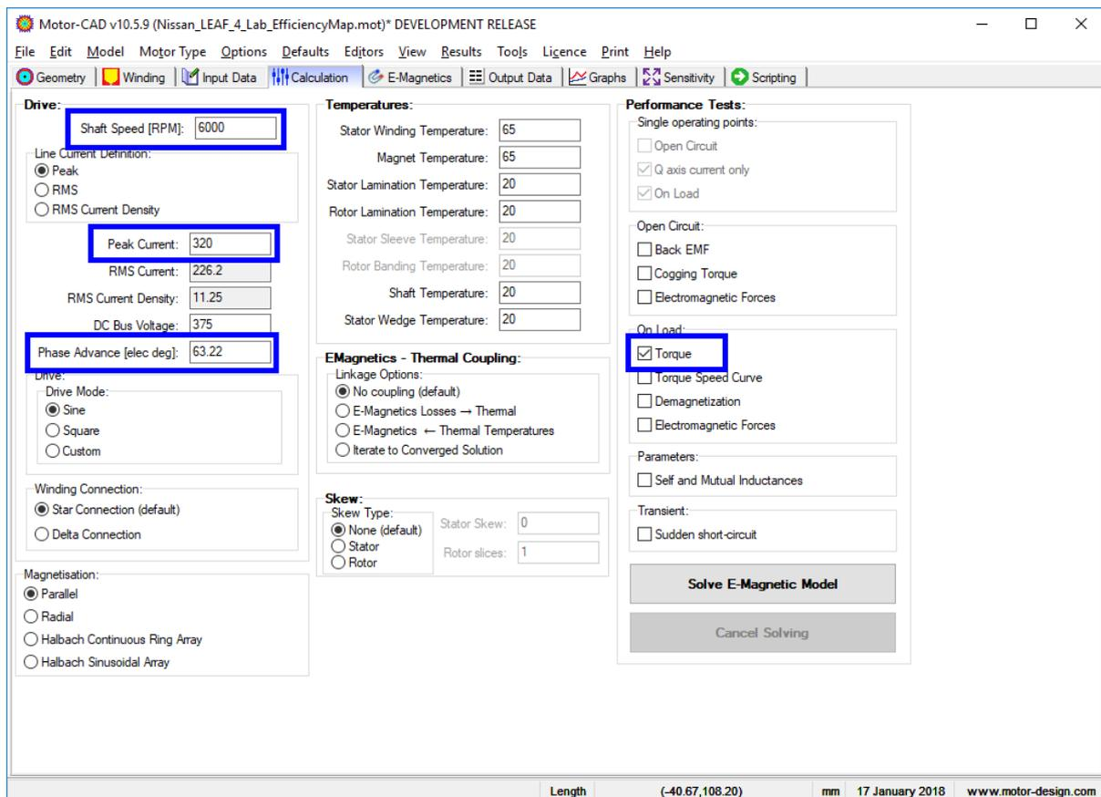
Under **Output Data -> E-Magnetics**, we see that the shaft torque and efficiency found from the transient FEA solution are within 1.5% of the values calculated from the Lab model. We can view other detailed results for this operating point, for example flux plots, torque waveforms, harmonic analysis, loss distribution, etc.
