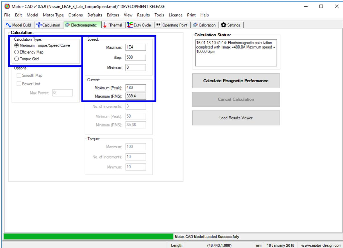
Click **Calculate Emagnetic Performance**, and the calculation should complete in a few seconds. The results are automatically shown in a new window. Previously calculated results can also be loaded at a later point with the **Load Results Viewer** button.
