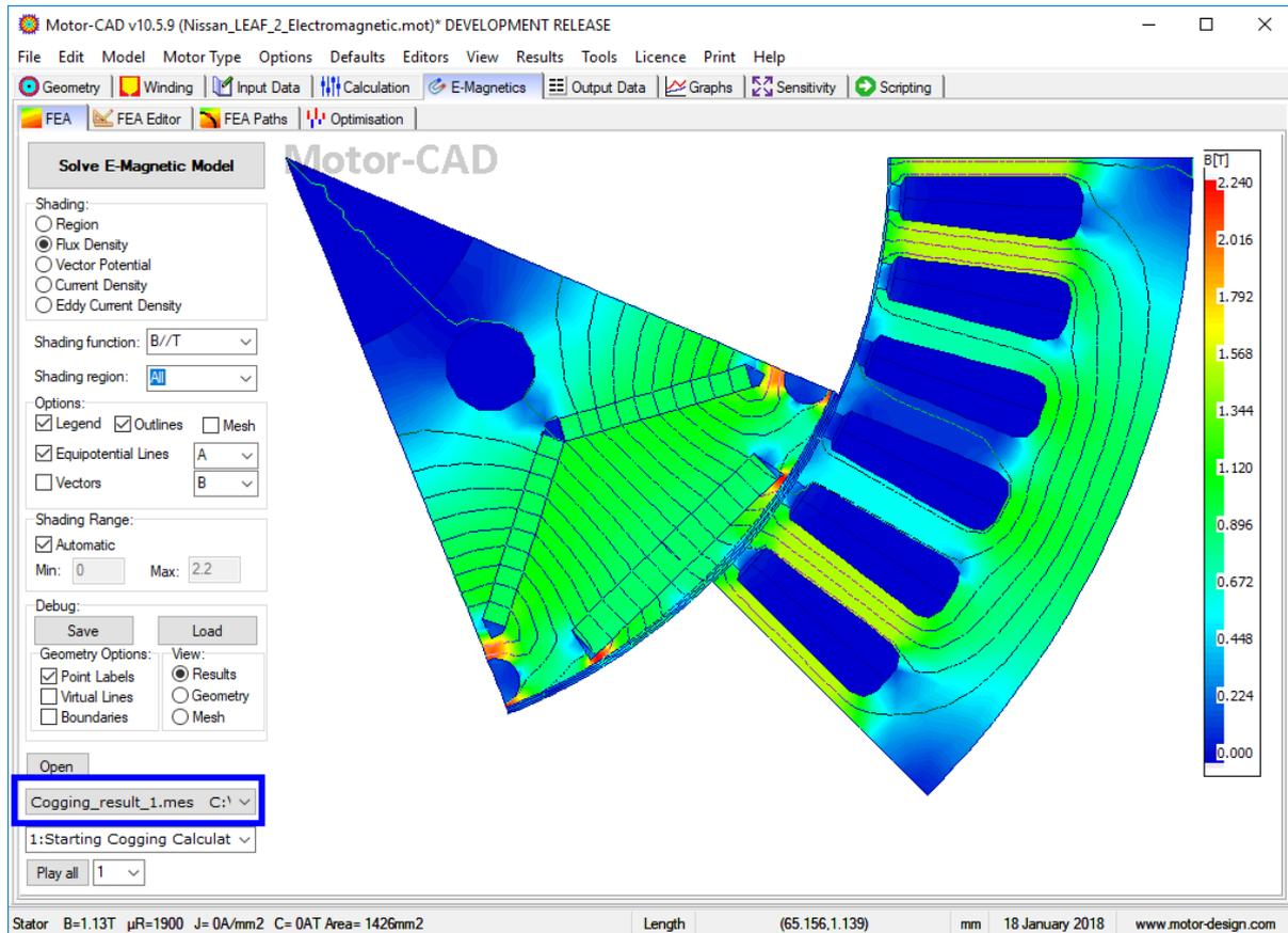
A separate results file is generated for each calculation, including the single operating points that are always simulated regardless of the performance tests selected by the users. The results for each calculation can be viewed by selecting the results file from the dropdown list in the left hand pane as highlighted above.
