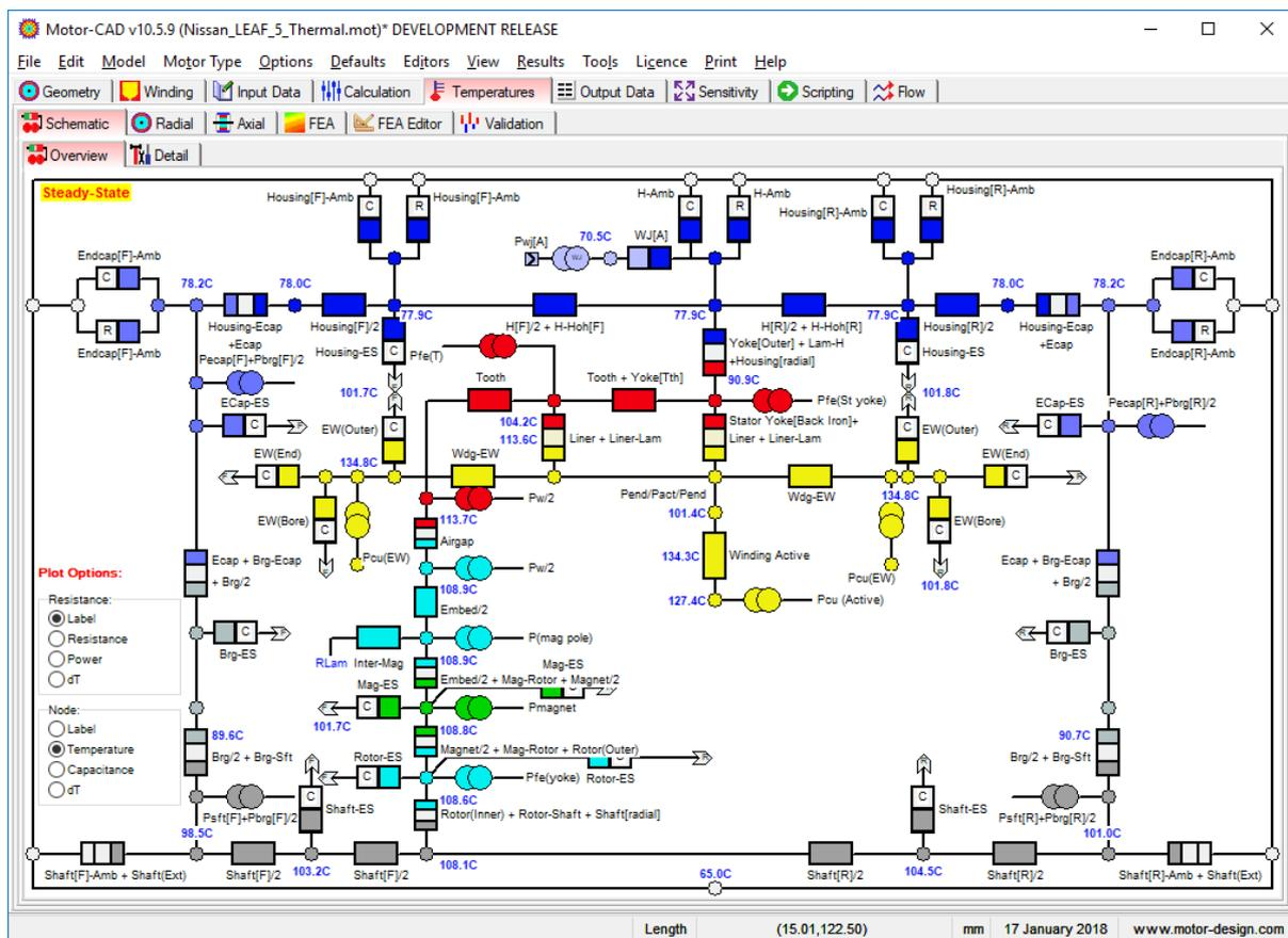
The complete thermal network can be viewed under **Temperatures -> Schematic -> Detail -> Circuit**. This is similar to the schematic view shown above but provides more detail on the complete thermal circuit, including all connections between the components.
