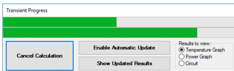
When solving is completed, the results are plotted against time in the **Transient Graph** tab. By default the temperature and power values are plotted for common nodes of interest. Using the **Setup** tab, the graphs can be customised to display the results for any nodes. The chart titles, axis limits and series options can also be changed. The **Data** tab provides the raw data for viewing or exporting, and the **Graphs** tab displays the plots.
