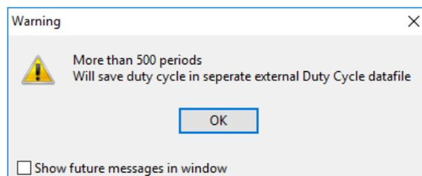
For duty cycles with fewer than 500 periods, Motor-CAD will save the duty cycle data in the .mot file. Otherwise, the data is automatically saved to a separate external file to prevent the size of the .mot file from growing too large. Here a location must be selected for saving the external file.
