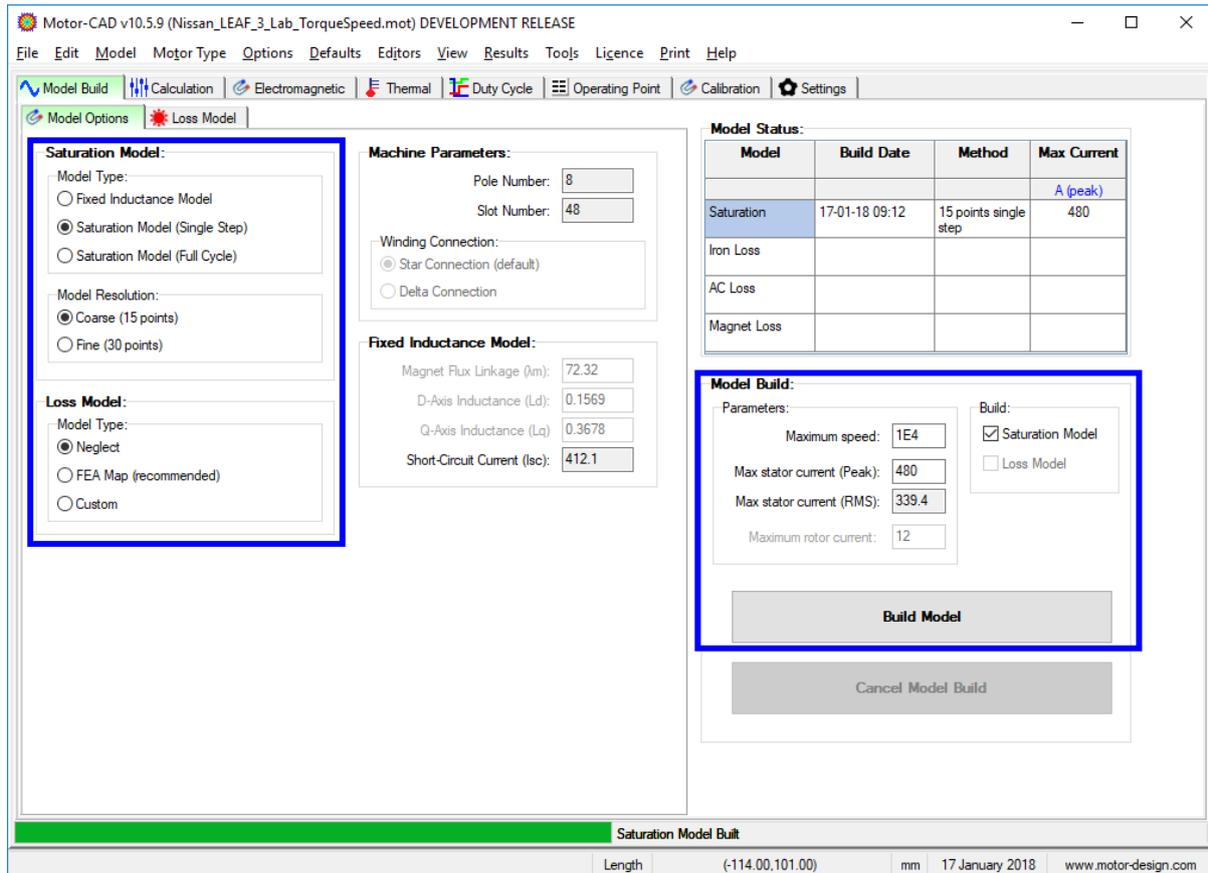
Note that if any changes are made to the settings in the **Model Build** tab (e.g. loss model type is changed), the model must be rebuilt. If any changes are made to the machine geometry, winding or materials in the E-Magnetic or Thermal context, the Lab model also must be rebuilt to reflect the changes. This will not be done automatically.
