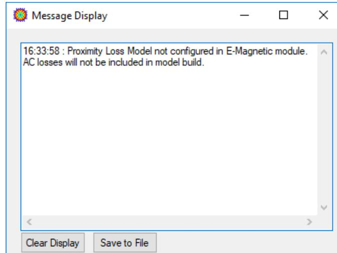
This is just informing us that the proximity losses (AC losses) will not be included in the Lab model since they have not been configured in the E-Magnetic model. This is fine for now – later on, in the **Advanced E-Magnetic Modelling** section, we will add proximity losses to our E-Magnetic model and then return to Lab to include them in the Lab model.
