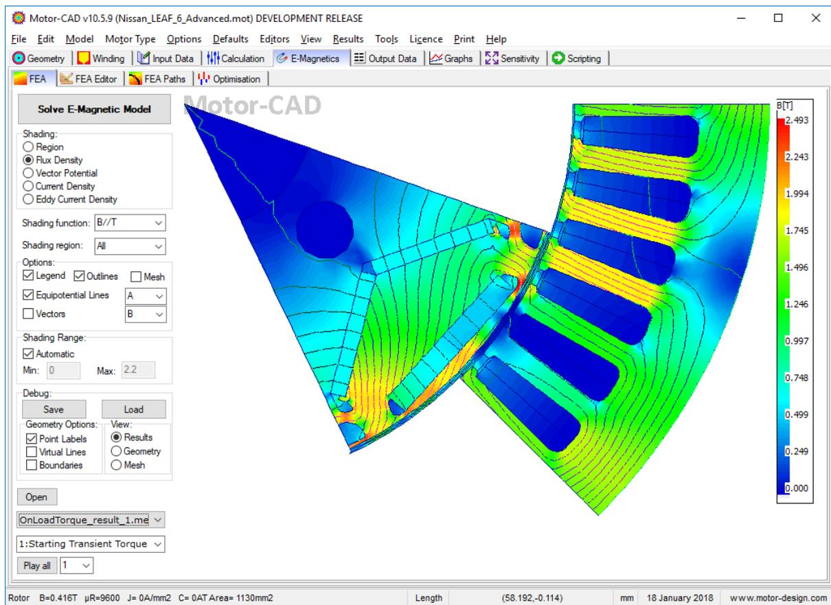
We can check the impact of the geometry customisation on the machine performance in the **Graphs**.
