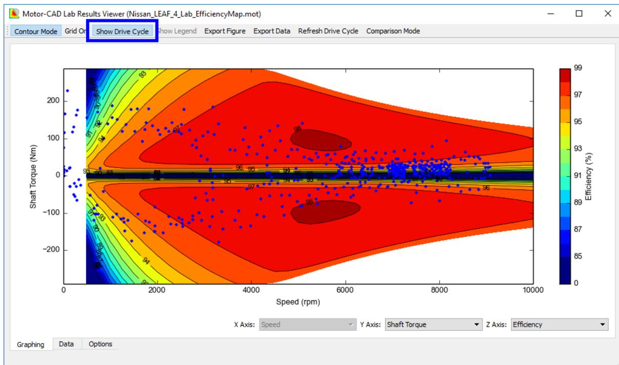
The duty cycle loss values can be exported to the Thermal module in order to calculate the thermal performance over the cycle. We will come back to this step later, after we have configured the thermal model.
