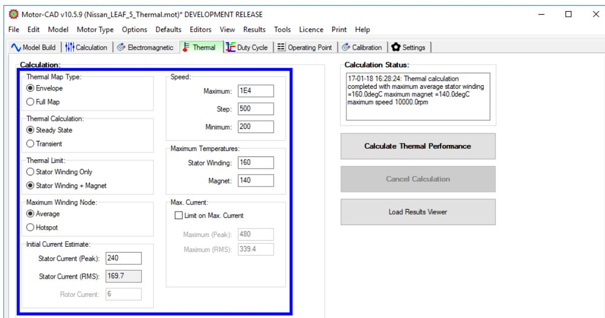
Click **Calculate Thermal Performance** to run the calculation. Note that, since the electromagnetic and thermal calculations must be iterated to find the optimum working point at maximum temperature, this calculation can take some time. The calculation can also be sensitive to the **Initial Current Estimate** so it is advised to ensure that a sensible value is used; typically  $\frac{1}{2}$  of the model build current is appropriate.
