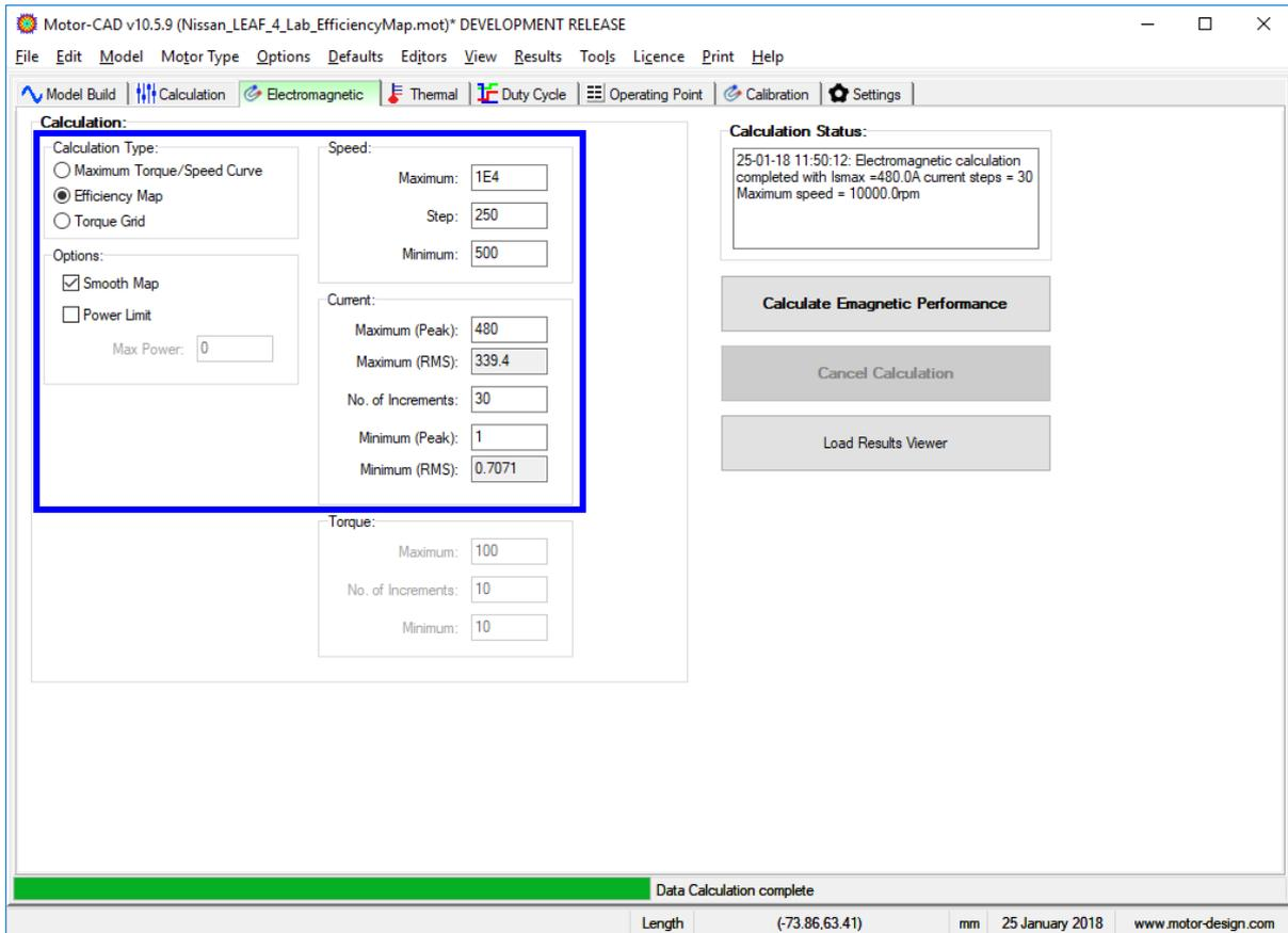
Click **Calculate Emagnetic Performance** to run the calculation. Again, the efficiency map is shown automatically. Other values can be plotted by selecting from the **Y Axis** and **Z Axis** dropdown, and the appearance of the plot (e.g. min/max values, number of contour lines) can be customised in the **Options** tab.
