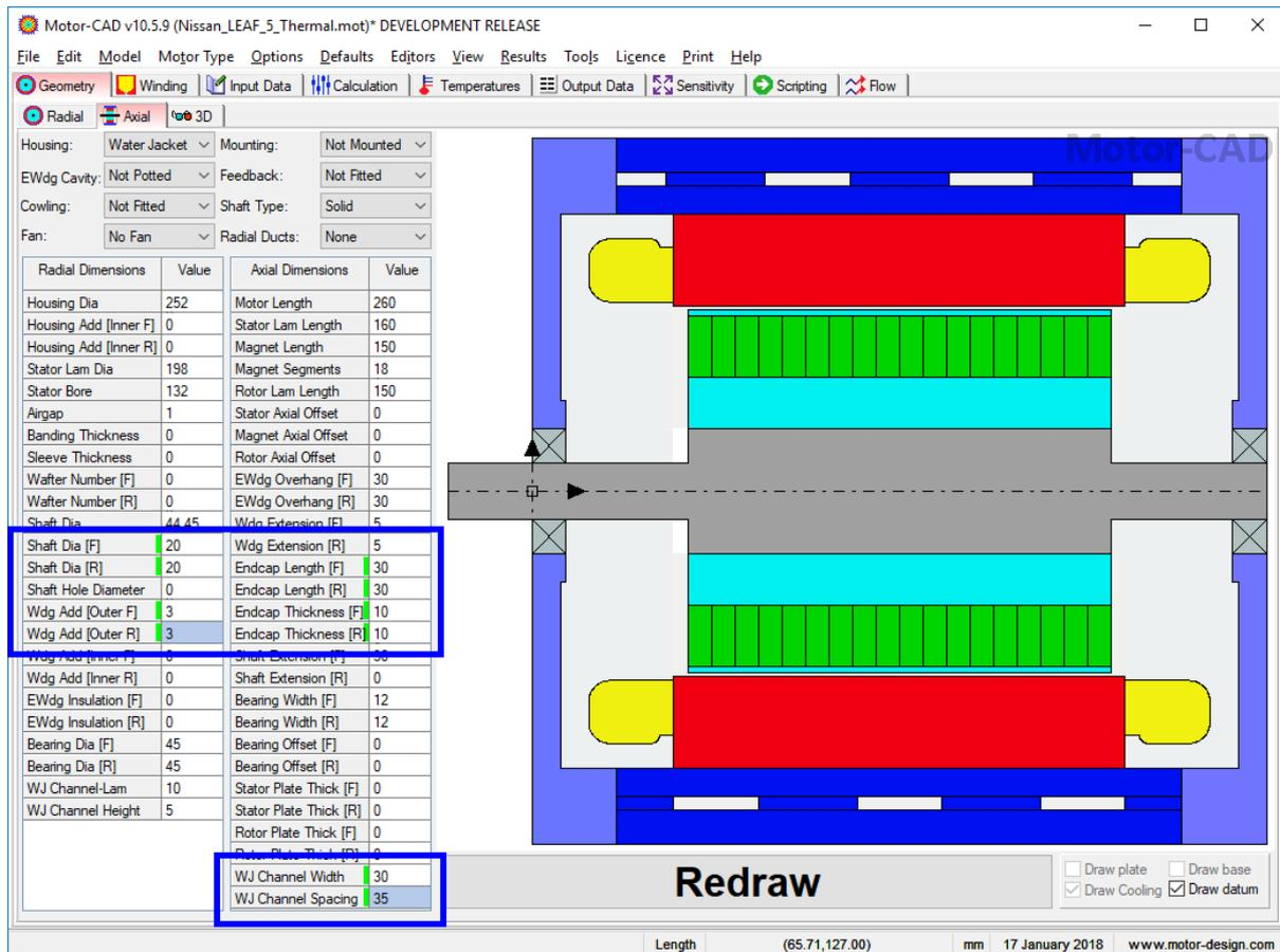
Motor-CAD v10.5.9 (Nissan\_LEAF\_5\_Thermal.mot)\* DEVELOPMENT RELEASE
