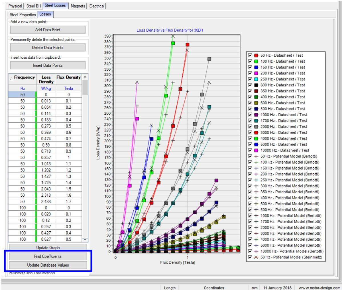
The coefficients calculated can be seen in the **Steel Properties** tab.
