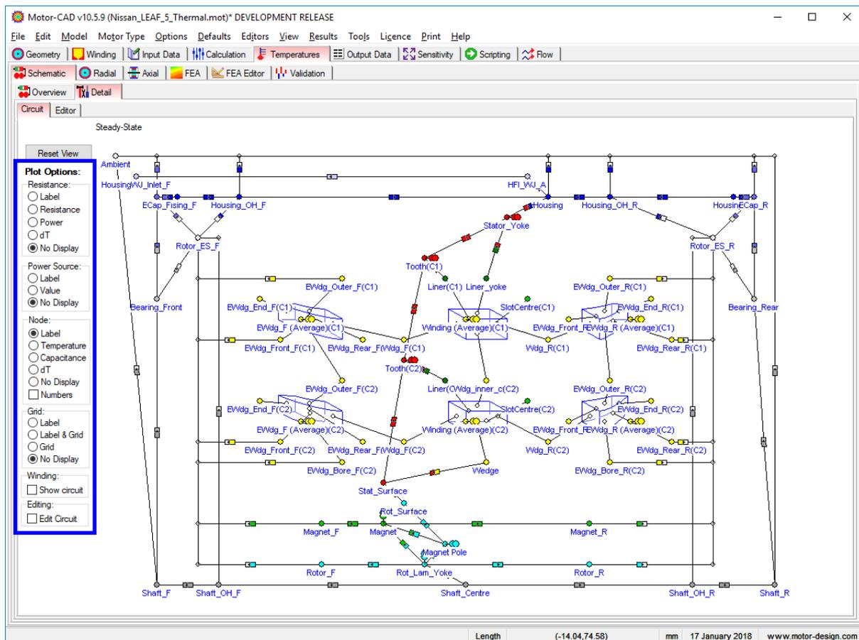
Here we can also understand the cuboidal model used for the stator windings, shown in yellow in the centre of the circuit. We have two rows of winding nodes, C1 (cuboid 1) and C2 (cuboid 2), with the front end winding nodes on the left and rear end winding nodes on the right.
