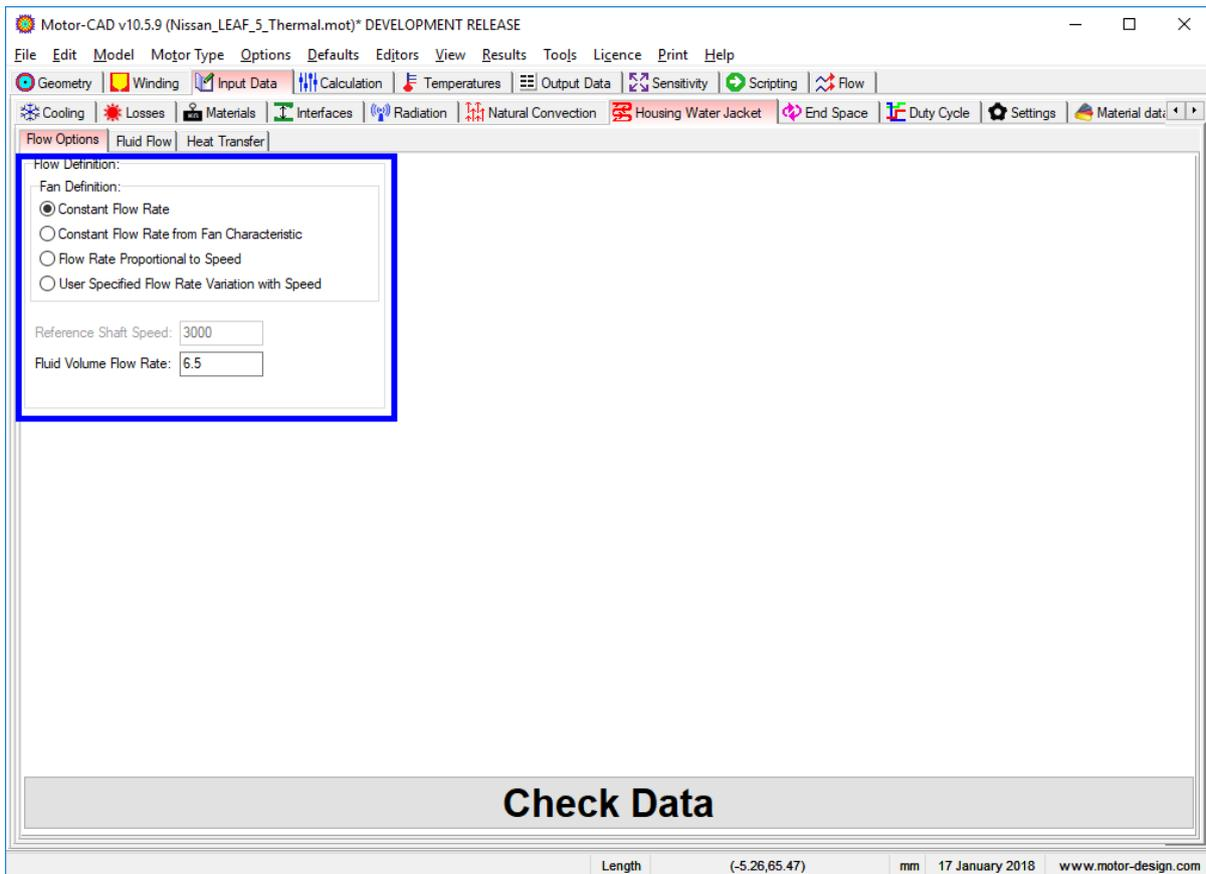
Under **Input Data -> Housing Water Jacket -> Fluid Flow**, we define the fluid properties and other details of the flow through the water jacket:
