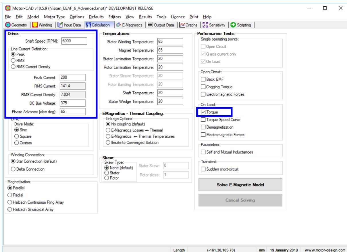
The screenshot shows the Motor-CAD v10.5.9 software interface. The 'Calculation' tab is active, and the 'Torque' option under 'Performance Tests' is checked. The 'Drive' section is highlighted with a blue box, showing the following parameters:
