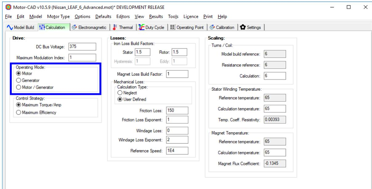
Under the **Electromagnetic** tab, we check the settings and click **Calculate Emagnetic Performance** to generate the efficiency map.
