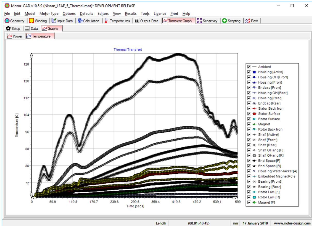
We are particularly interested in the stator winding and magnet temperatures. Under **Transient Graph -> Setup -> Temperature Graph Setup**, customise the transient graph to show only the **Ambient, Magnet, Winding (Average)** and **Winding (Hotspot)** nodes (the **Select/Deselect all nodes** checkbox can be useful here). Deselect the **Draw Points** option.
