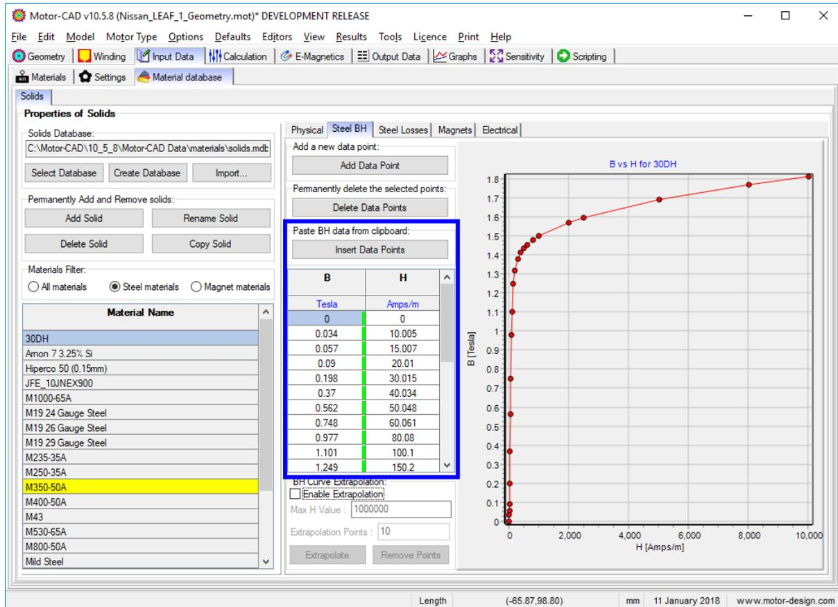
In addition to the manufacturer’s data, Motor-CAD can estimate further BH points beyond the maximum values of the experimental data typically available. Select the **Enable Extrapolation** option to enable this functionality. Enter a maximum H value which will give a good safety margin for the expected flux density values in the simulation, and select the number of points to provide a good set of data. In this case, the following values are appropriate:
