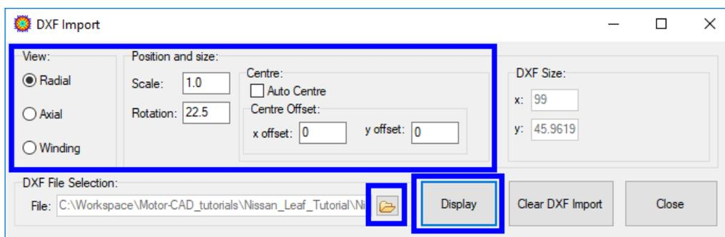
Click **Display** to show the DXF outline on the **Geometry -> Radial** cross-section, and then close the dialog.
