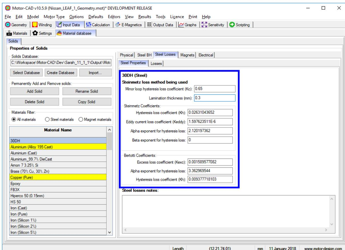
This completes the process of adding the new steel to the materials database. When saving the .mot file, all data relating to the materials used in the model will be contained in the file. In addition, the materials database file can be shared to allow organisations to work from a standard set of materials.
