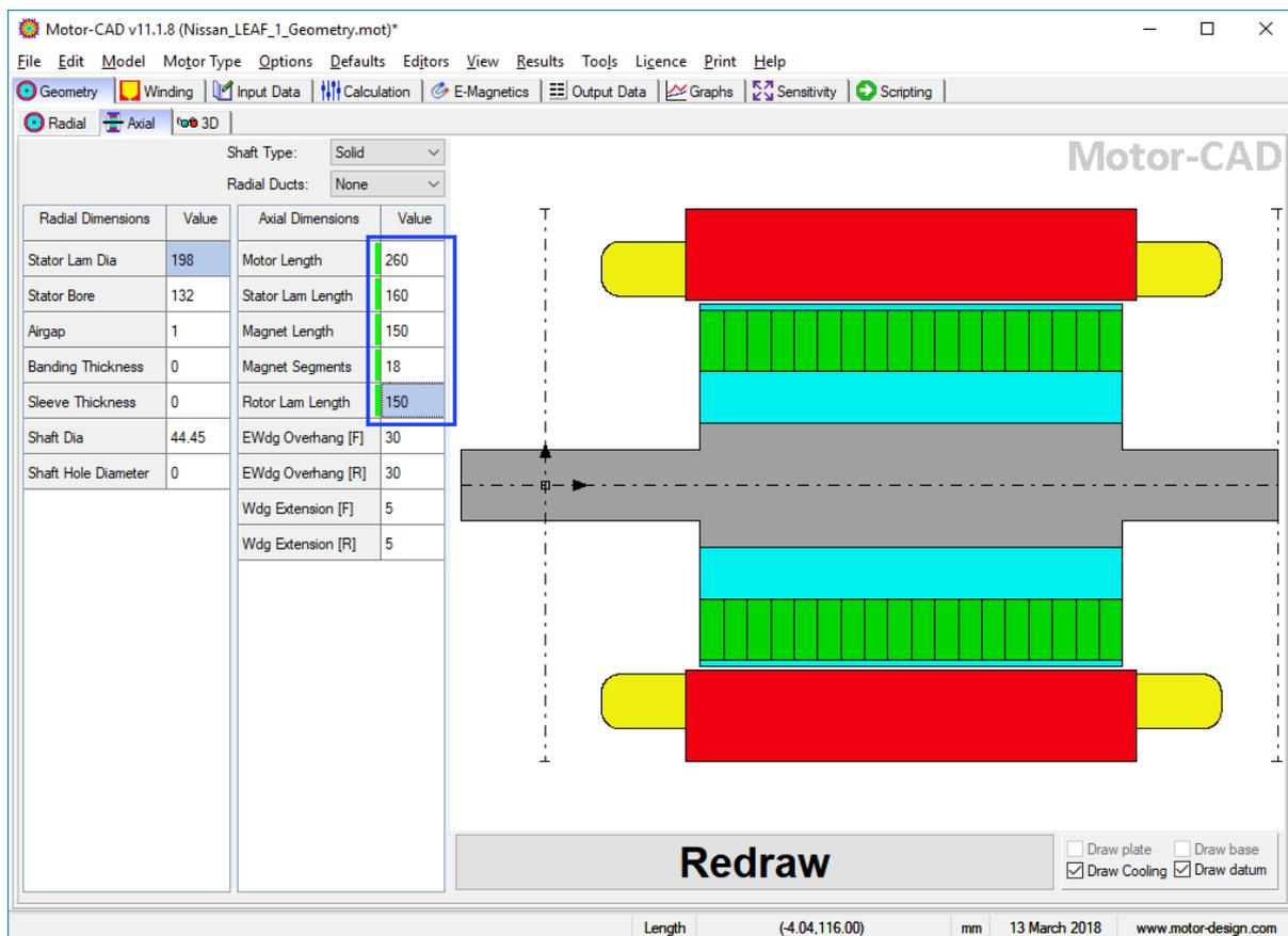
The screenshot shows the Motor-CAD v11.1.8 interface with the **Axial** tab selected. The **Axial Dimensions** table is highlighted with a blue border, showing the following values:
