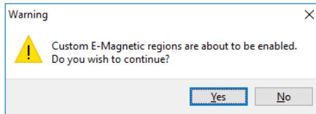
This is warning that we are about to start using custom regions for the FEA simulation instead of the default regions generated by Motor-CAD. We click **Yes** to continue with the region editing and notice that the **Use Custom E-Magnetic Regions** checkbox has been automatically enabled.
