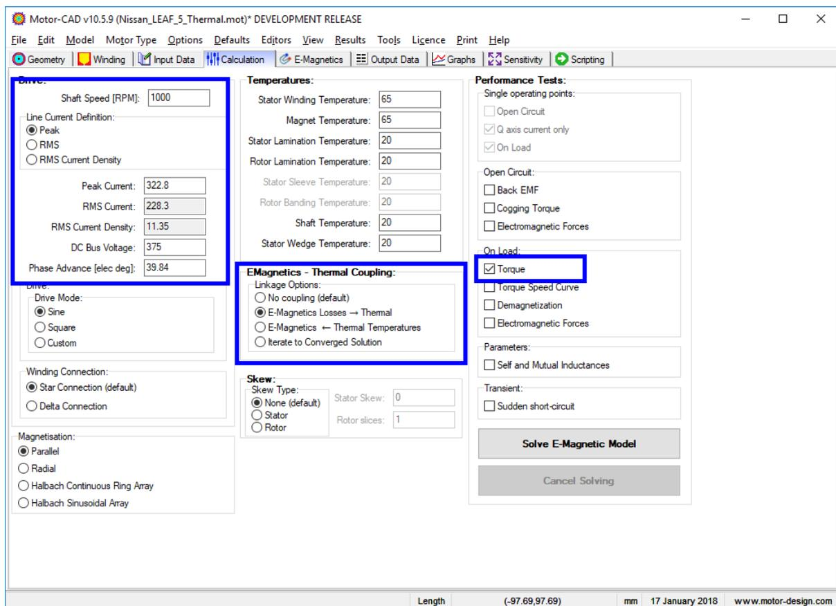
Now **Solve** the model. Once solving is completed, check the loss values under **Output Data** -> **Losses**.
