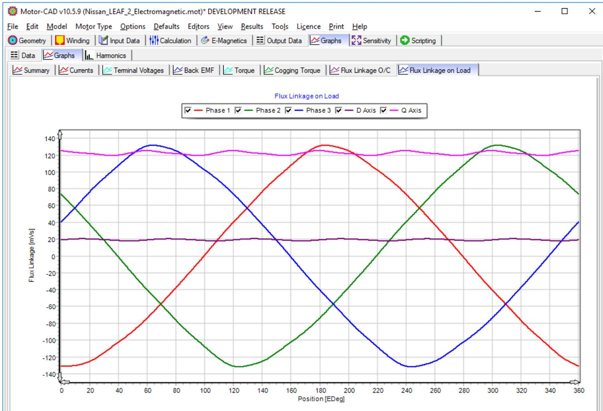
We can also check the harmonic analysis of the waveforms under **Graphs -> Harmonics**. Note the characteristic 6<sup>th</sup> and 12<sup>th</sup> harmonics in the torque waveform.
