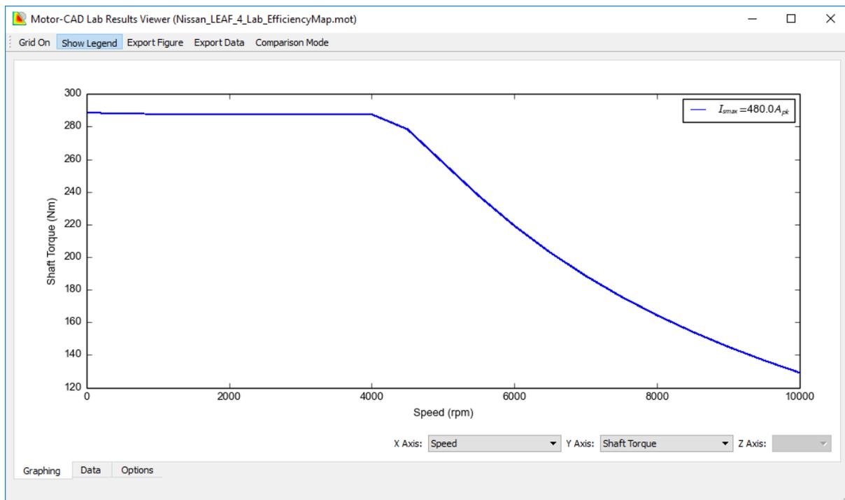
We will now calculate the full efficiency map. Close the viewer and return to the Motor-CAD window. As well as including the copper, iron and magnet losses through FEA-based models, we can also defined the mechanical losses. These are typically comprised of a friction (e.g. bearing losses) and windage loss component.
