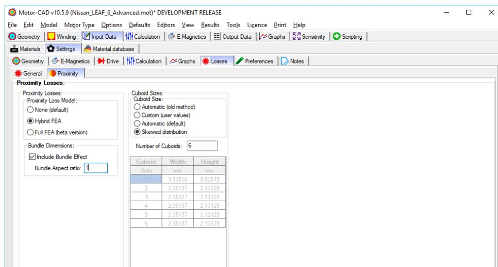
The proximity losses are typically larger towards the slot opening due to the magnetic field generated by the rotor. Selecting the **Skewed distribution** option allows Motor-CAD to increase the number of cuboids around the slot opening, increasing the resolution in this region and hence improving the accuracy of the proximity loss calculation.
