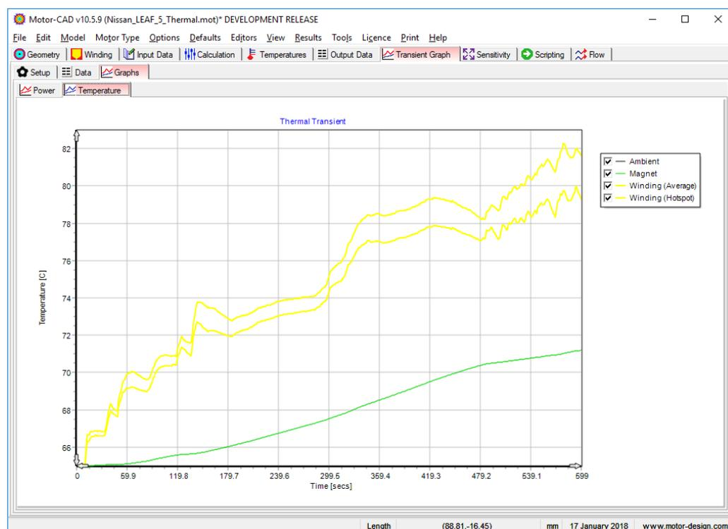
Furthermore, more than one cycle of the duty cycle can be simulated. Change the **Number of Cycles** to **5** under **Input Data -> Duty Cycle -> Settings**, and then run the calculation again from the **Calculation** tab.
