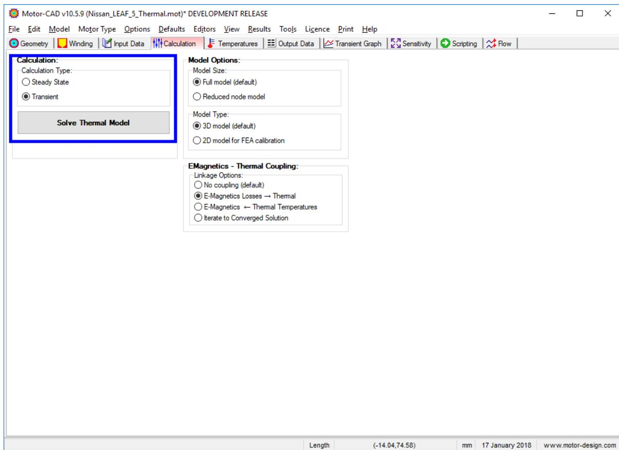
During solving, the transient progress bar shows the progress of the simulation. By default the results are not shown during the solution for speed, but can be displayed using the options here.
