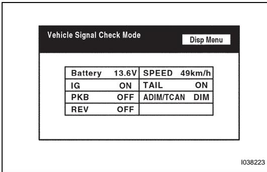
(b) When the "Vehicle Signal Check Mode" screen is displayed, check all the vehicle signal conditions.
