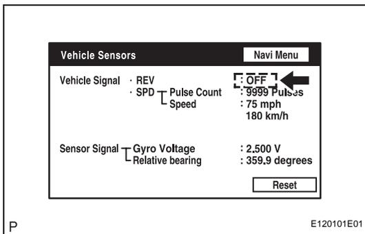
(a) Check that the display changes between ON and OFF according to the shift lever operation (P and R).
