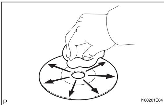
(a) If dirt is on the disc surface, wipe it clean with a soft cloth from the inside to the outside in a radial direction.
