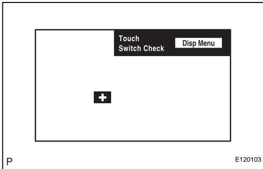
(b) Touch the display anywhere in the open area to perform the check when the "Touch Switch Check" screen is displayed.
