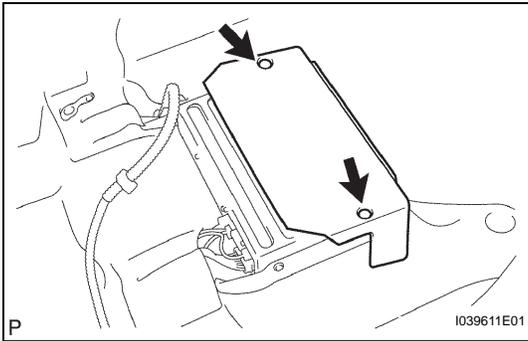
(b) Remove the 3 bolts and navigation ECU with bracket.
