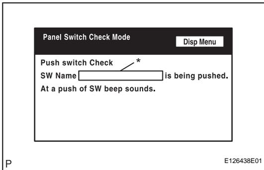
(b) Operate each switch and check that the switch name and condition are correctly displayed.
