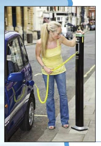
The first electric cars were made in the 19th century. A few are still made today. Instead of a gas tank, they usually have batteries, which store electricity. Instead of an internal-combustion engine, they have an electric motor. The motor uses electricity from the batteries to produce a turning action. This action is used to turn the car's wheels.
