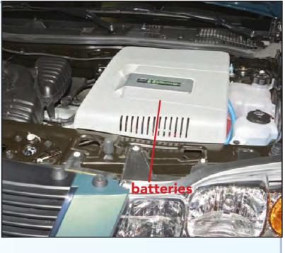
Car makers are trying to make the batteries in hybrids smaller and lighter. This model has smaller-than-usual batteries.
