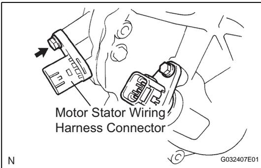
**14. REMOVE MOTOR STATOR WIRING HARNESS CONNECTOR**
