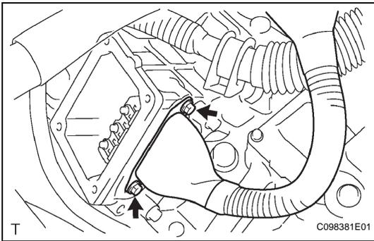
(2) Remove the 2 bolts from the generator cable.
