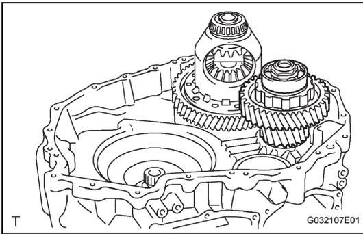
**6. INSTALL DIFFERENTIAL DRIVE PINION**
