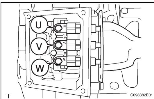
(b) Connect the generator cable as shown in the illustration.
