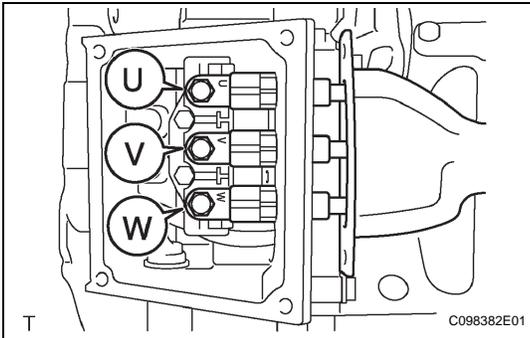
(3) Inspect the voltage between each of the 3 phase AC terminals (U to V, V to W, U to W) and body ground using the Toyota electrical tester.
