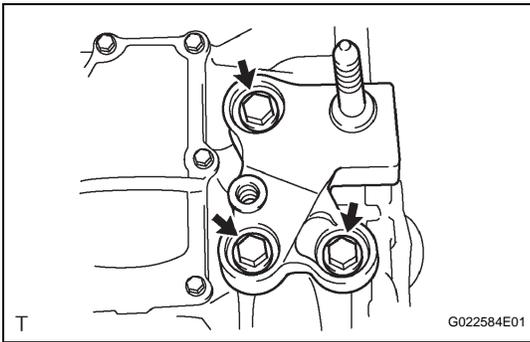
**12. REMOVE NO. 3 ENGINE MOUNTING BRACKET**
