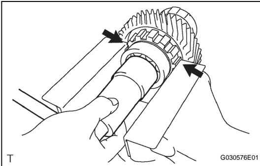
(c) Using SST and a press, press out the bearing from the differential driver pinion.
