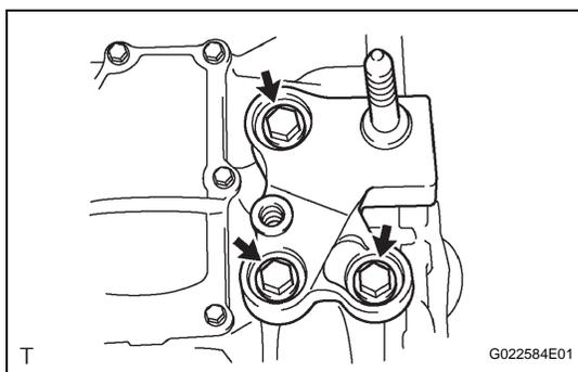
**32. INSTALL HYBRID VEHICLE TRANSAXLE ASSEMBLY**
