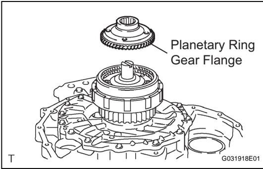
(10) Install the planetary ring gear flange.
