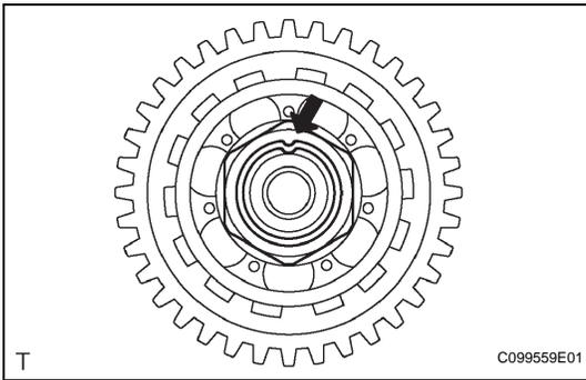
(b) Set the differential drive pinion in a vise and remove the nut using a deep socket wrench.
