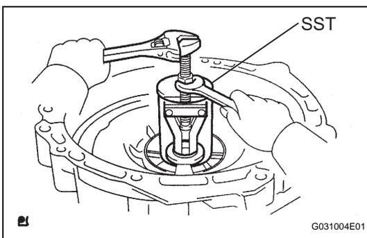
**30. REMOVE HYBRID VEHICLE TRANSAXLE ASSEMBLY TYPE T OIL SEAL**
