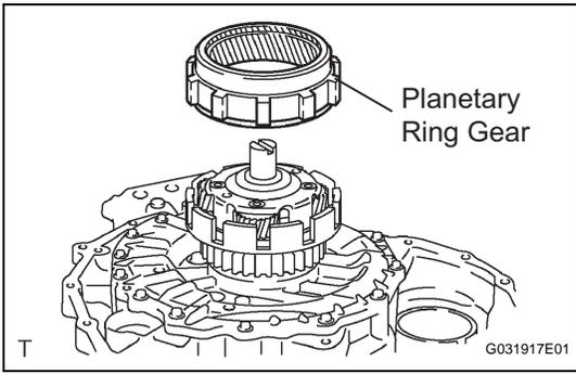
(9) Install the planetary ring gear.
