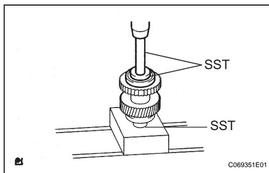
(c) Using SST and a press, press in the bearing to the counter drive gear.
