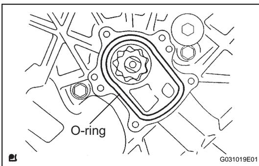
**4. INSTALL TRANSMISSION OIL PUMP COVER SUB-ASSEMBLY**
