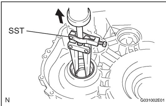
**22. REMOVE DIFFERENTIAL CASE LH TAPERED ROLLER BEARING RACE**
