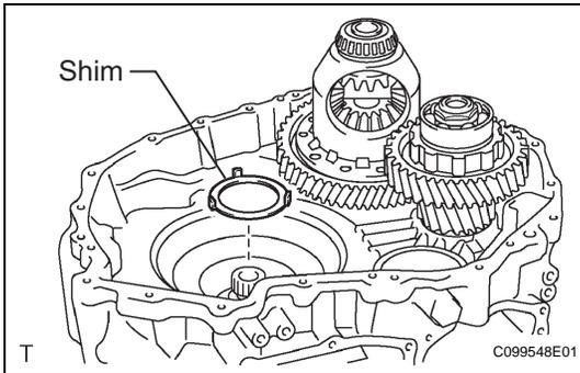
**8. INSTALL INPUT SHAFT ASSEMBLY**
