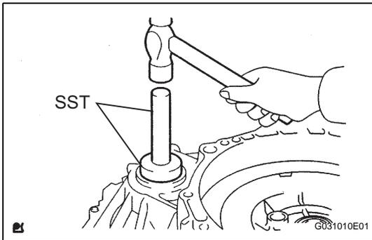
**3. INSTALL HYBRID TRANSAXLE OIL SEAL RH**
