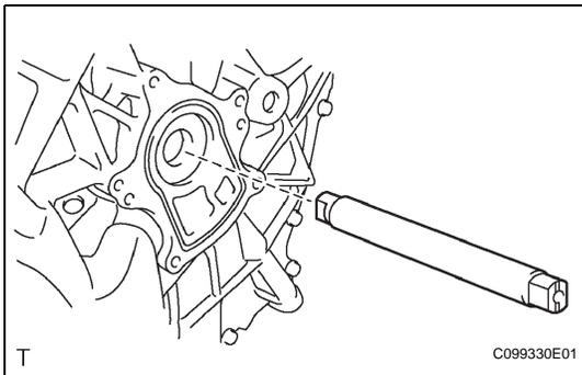
(b) Remove the oil pump drive shaft.
