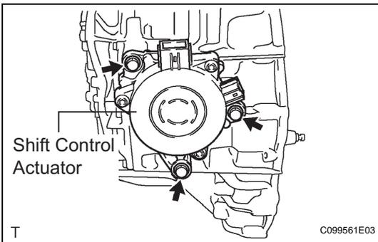
**15. REMOVE SHIFT CONTROL ACTUATOR ASSEMBLY**
