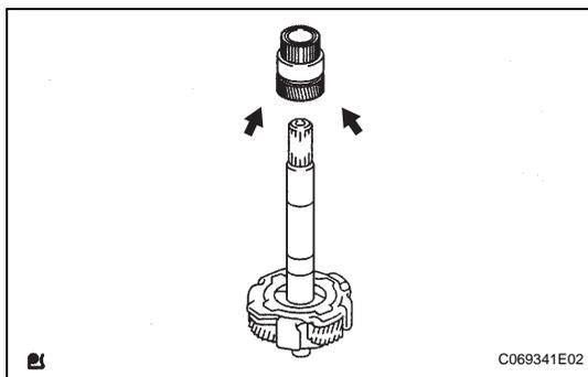
2. **INSTALL PLANETARY SUN GEAR SUB-ASSEMBLY**
