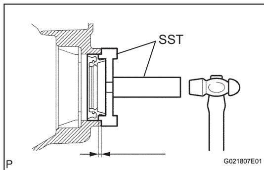
8. INSTALL HYBRID TRANSAXLE OIL SEAL
