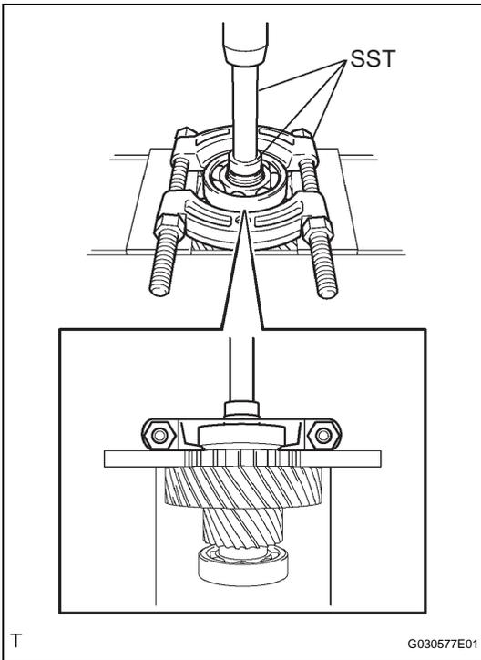
(d) Using SST and a press, press out the bearing from the differential drive pinion.
