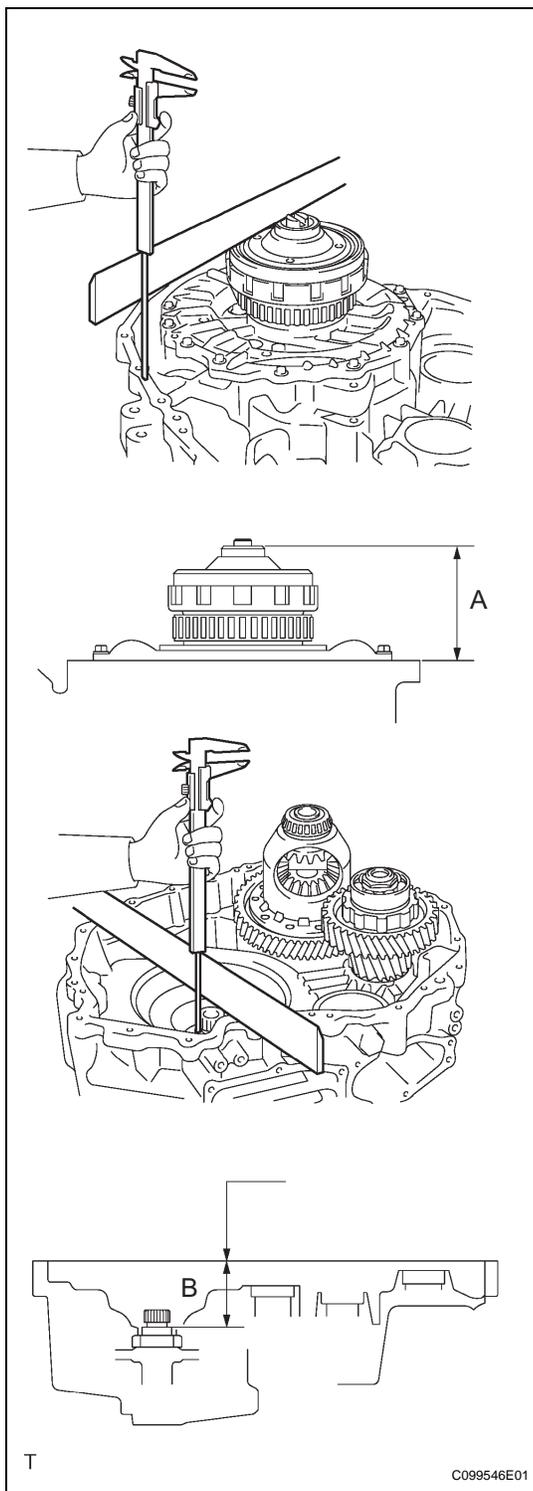
(11) Using a straightedge and vernier caliper, measure dimension A as shown in the illustration.
