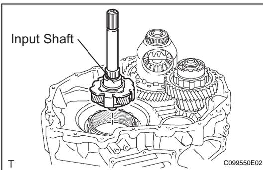
(g) Install the input shaft.
