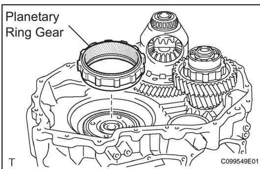
(f) Install the planetary ring gear.
