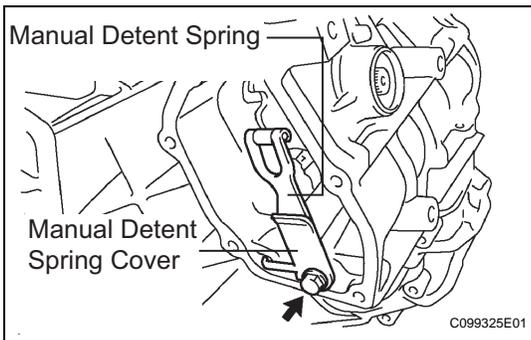
**19. INSTALL MANUAL DETENT SPRING SUB-ASSEMBLY**
