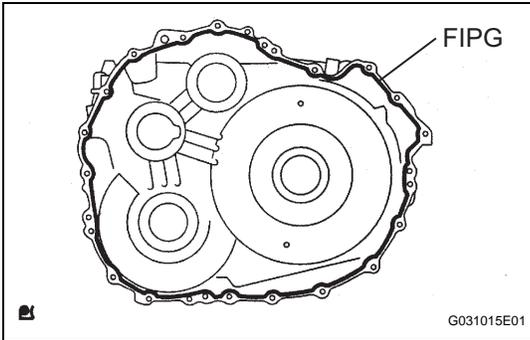
**13. INSTALL HYBRID VEHICLE GENERATOR ASSEMBLY**
