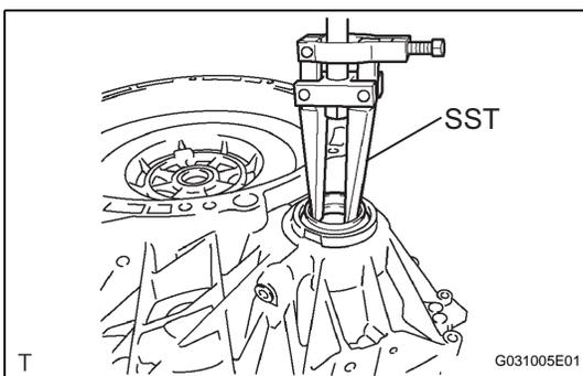
**31. REMOVE HYBRID TRANSAXLE OIL SEAL RH**
