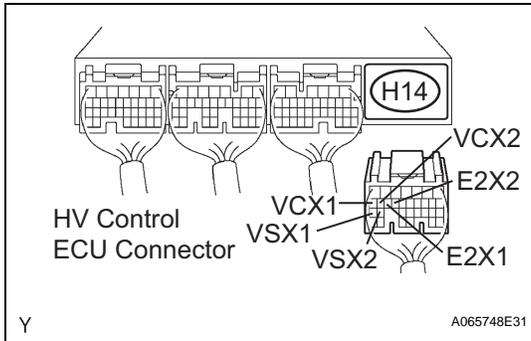
(a) Disconnect the H14 HV control ECU connector.
