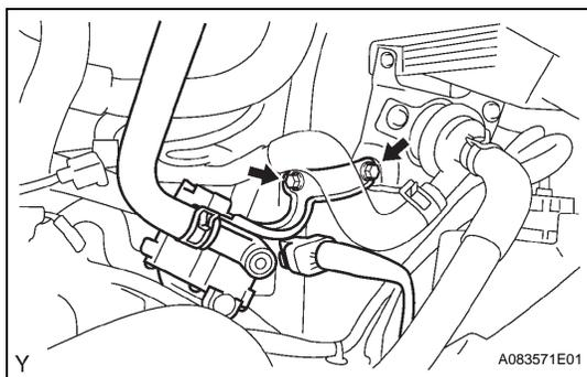
2. **INSTALL WATER VALVE WITH BRACKET ASSEMBLY**
