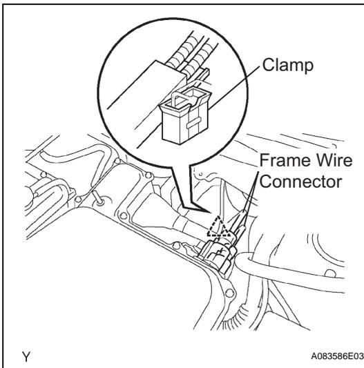
**10. INSTALL FRAME WIRE****CAUTION:****Wear insulating gloves.**
