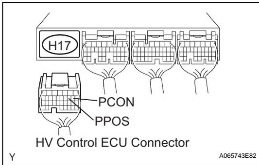
(a) Disconnect the H17 HV control ECU connector.
