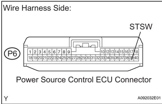
(b) Disconnect the P6 power source control ECU connector.
