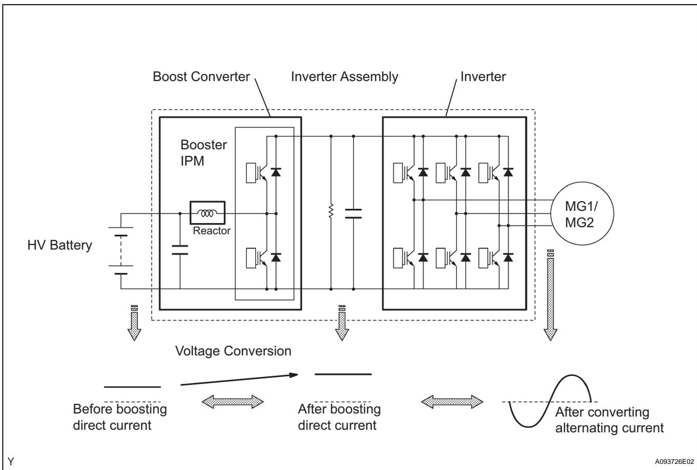
The HV control ECU uses a voltage sensor that is built into the boost converter to detect the high voltage (VL) before it is boosted. Also, it uses a voltage sensor that is built into the inverter to detect the high voltage (VH) after it has been boosted.
