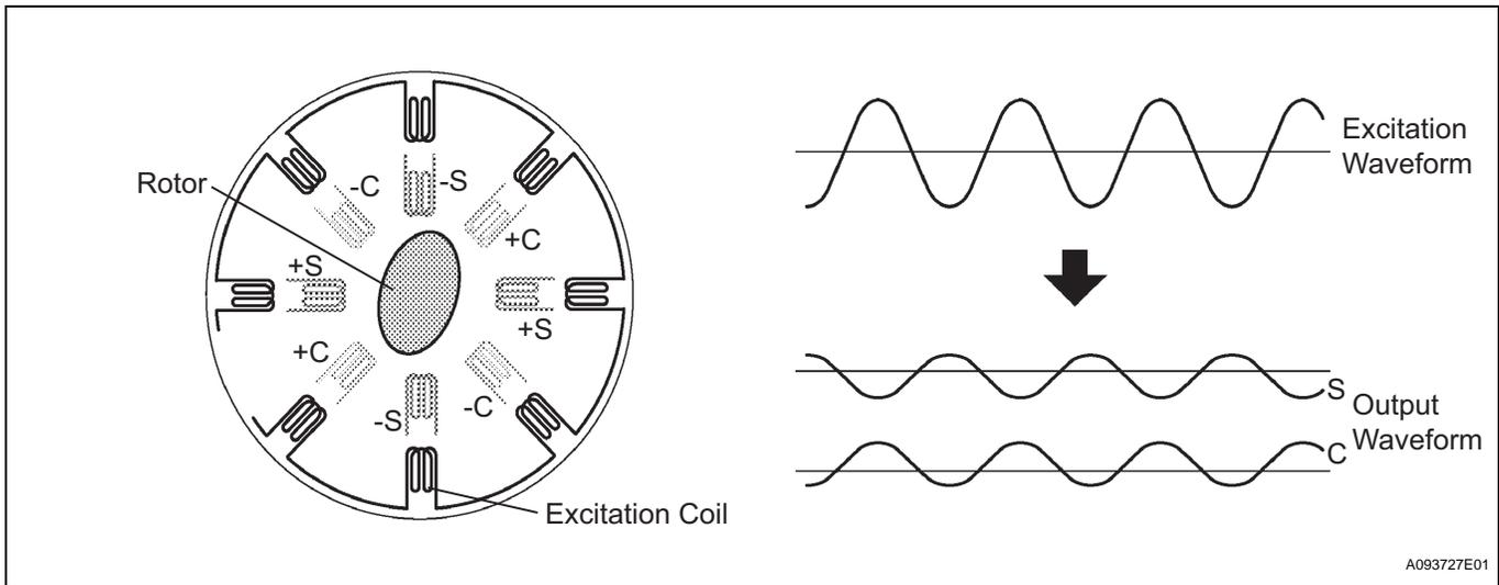
The HV control ECU monitors the output signals of the motor resolver and detects a malfunction.
