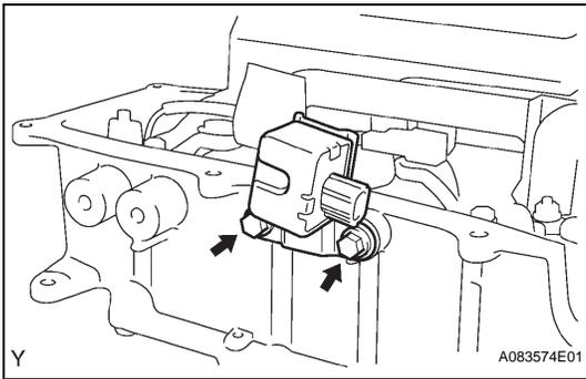
**29. REMOVE NO. 1 CIRCUIT BREAKER SENSOR**
