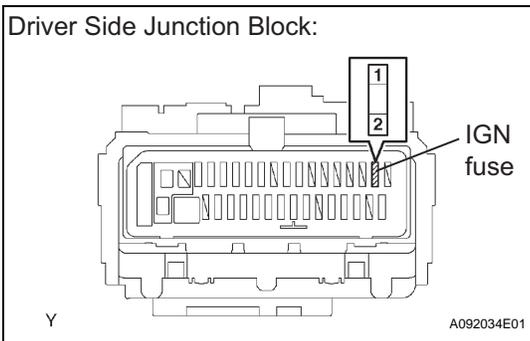
(b) Remove the IGN fuse from the driver side junction block.
