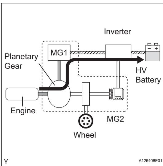
(3) MG1 is rotated by the engine via the planetary gear, in order to charge the HV battery.
