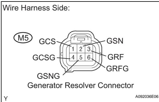
(b) Disconnect the M5 generator resolver connector.
