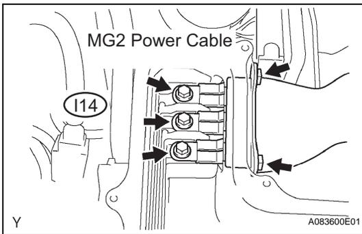
(e) Remove the 5 bolts to disconnect the MG2 power cable.
