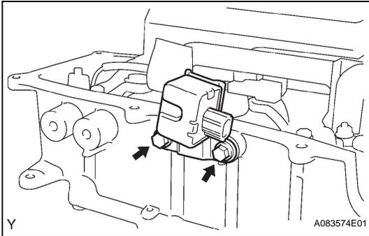
**INSTALLATION****1. INSTALL NO. 1 CIRCUIT BREAKER SENSOR**
