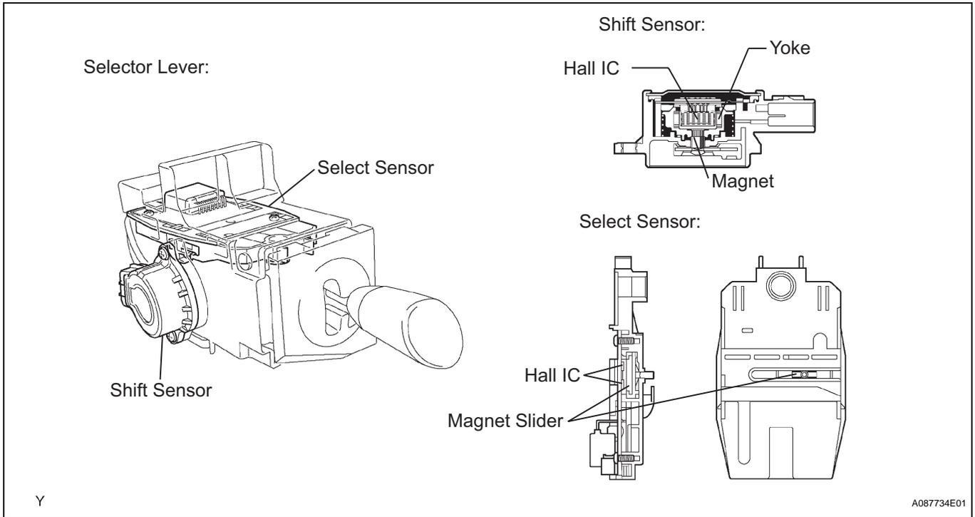
The shift sensor outputs voltage, which varies between 0 and 5 V in accordance with the vertical movement of the selector lever, to the HV control ECU. The HV control ECU interprets low level voltage as the D or B position, middle level voltage as the home or N position, and high level voltage as the R position.
