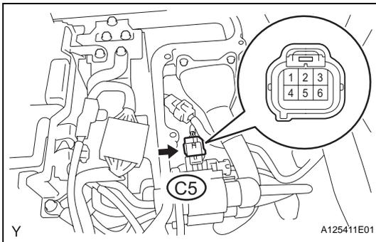
(g) Check the connection condition of the C5 connector.
