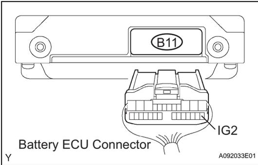
(a) Disconnect the B11 battery ECU connector.
