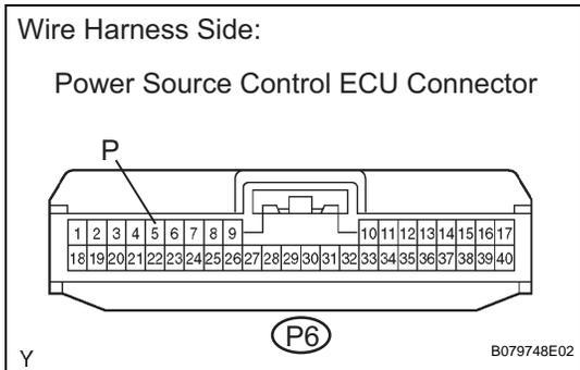
(c) Disconnect the P6 power source control ECU connector.
