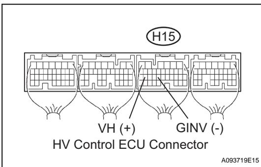
(b) Measure the voltage between the terminals of the H15 HV control ECU connector.
