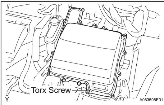
20. VERIFY THAT VOLTAGE OF INVERTER WITH CONVERTER IS 0 V
