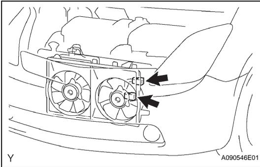
(a) Check the connection condition of the fan connectors.
