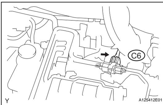
(a) Check that the C6 connector is connected securely.
