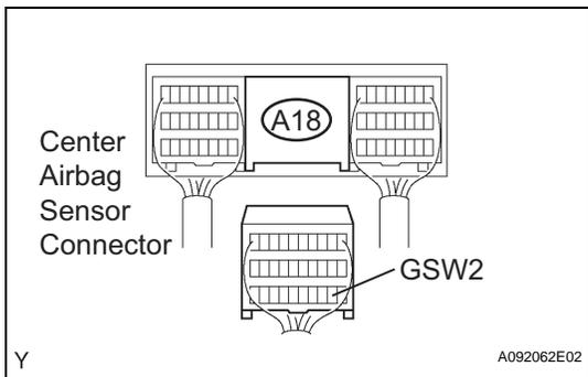
(b) Disconnect the A18 center airbag sensor connector.
