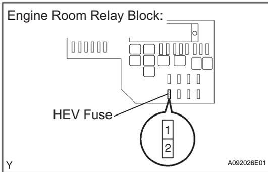
(b) Remove the HEV fuse from the engine room relay block.
