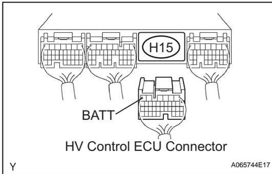
(a) Disconnect the H15 HV control ECU connector.
