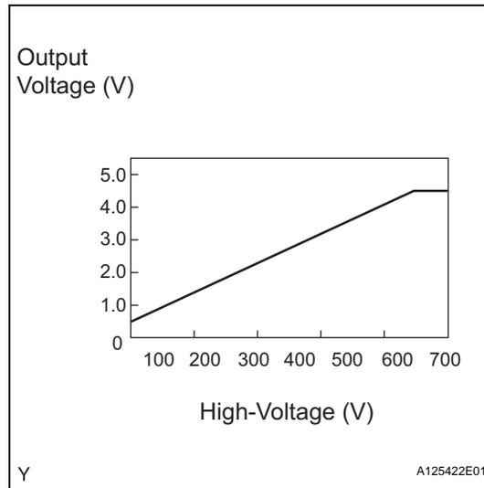
The inverter voltage sensor outputs a voltage that varies between 0 and 5 V in accordance with the changes in the high voltage. The higher the high voltage, the higher the output voltage, and the lower the high voltage, the lower the output voltage.
