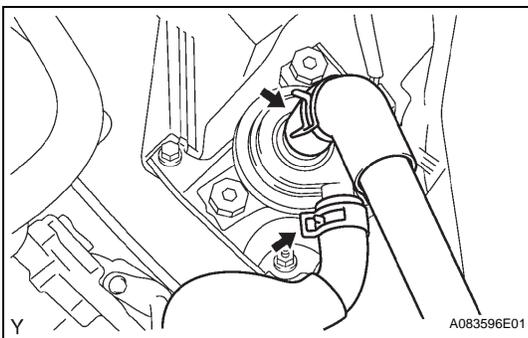
14. REMOVE WATER PUMP WITH MOTOR ASSEMBLY
