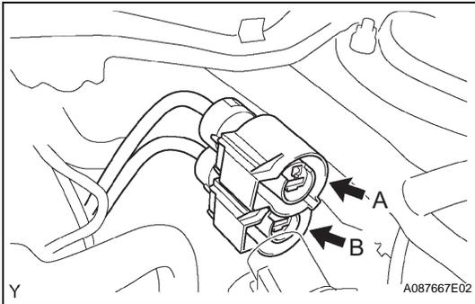
(b) Check that the frame wire has been disconnected from the system main relay.
