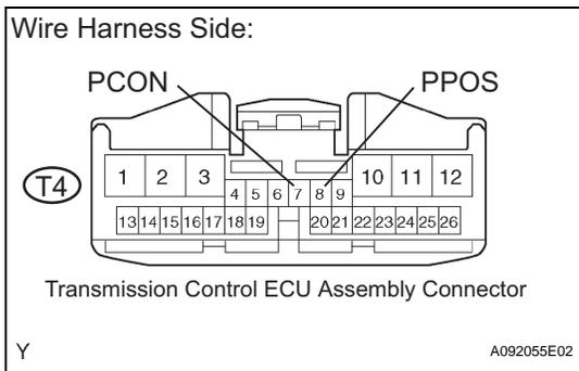
(b) Disconnect the T4 transmission control ECU assembly connector.
