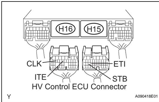
(a) Disconnect the H15 and H16 HV control ECU connectors.
