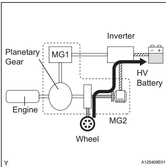
(4) When the vehicle is decelerating, kinetic energy from the wheels is recovered and converted into electrical energy and used to recharge the HV battery by means of MG2.
