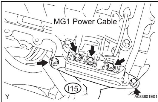
(f) Remove the 5 bolts to disconnect the MG1 power cable.
