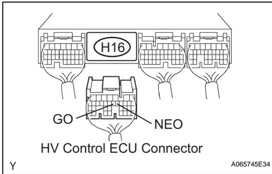
(a) Disconnect the H16 HV control ECU connector.
