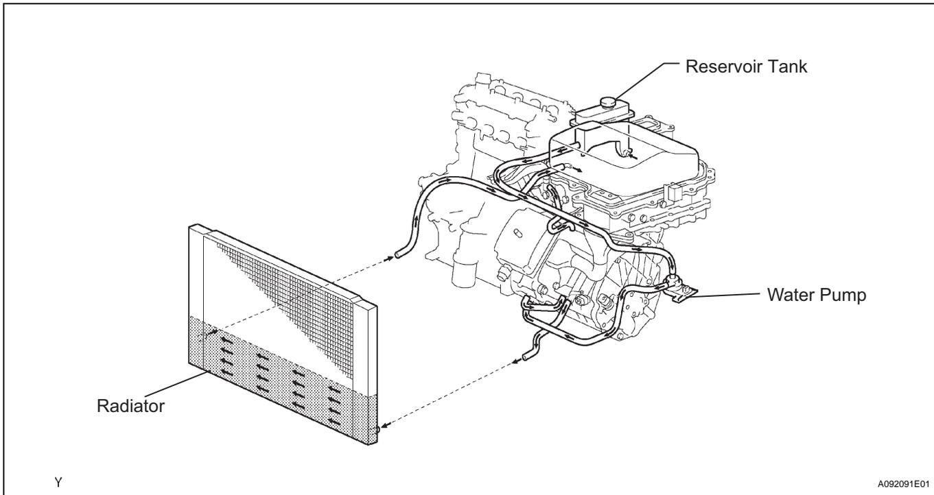
The HV control ECU monitors the electric water pump, cooling fan and cooling system, and detects a malfunction.
