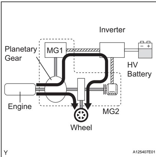
(2) While the wheels are being driven by the engine via the planetary gear, MG1 is rotated by the engine via the planetary gears, in order to supply the generated electricity to MG2.
