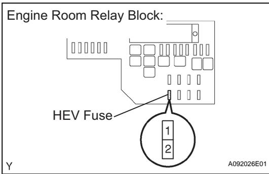
(c) Remove the HEV fuse from the engine room relay block.
