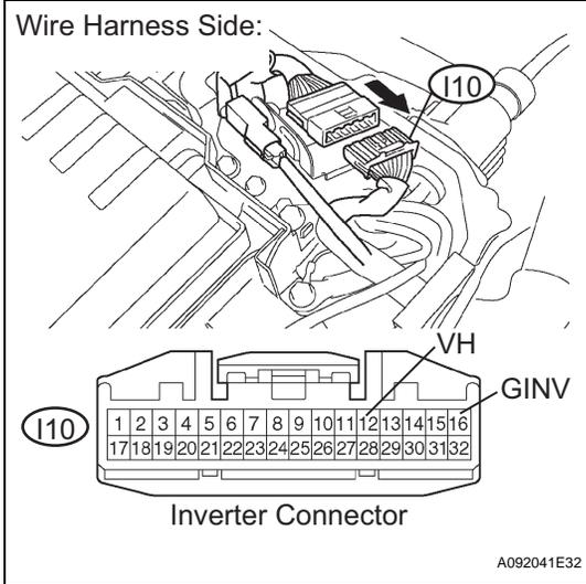
(e) Disconnect the I10 inverter connector.
