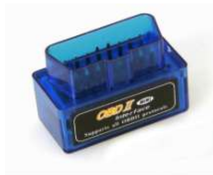
Kit figure 14. OBDII Scanner - Bluetooth comms
