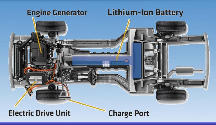
Battery is packaged in tunnel and under rear seat
