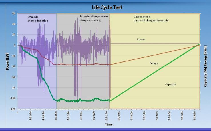
Opel Ampera battery packs are tested in life cycle tests 24/7
