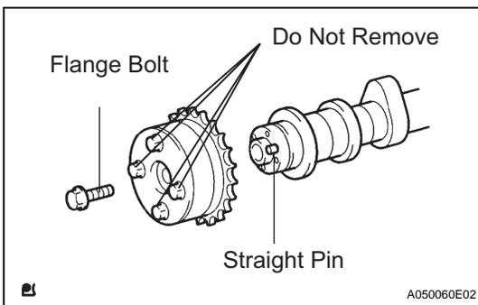
**26. REMOVE CAMSHAFT TIMING GEAR**
