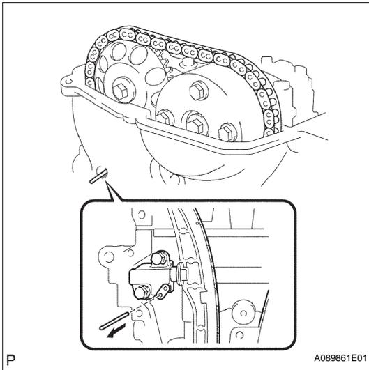
(ad) Remove the bar from the timing chain tensioner.
