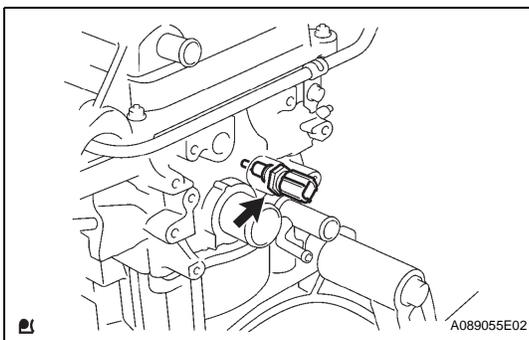
**INSTALLATION****1. INSTALL ENGINE COOLANT TEMPERATURE SENSOR**
