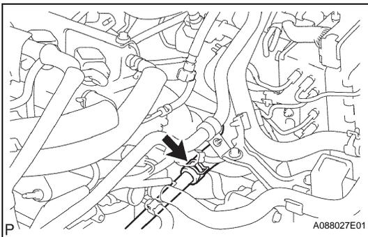
**29. DISCONNECT HEATER WATER HOSE**
