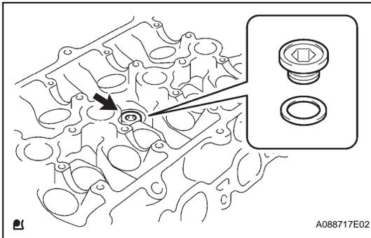
**2. REMOVE OIL CONTROL VALVE FILTER**
