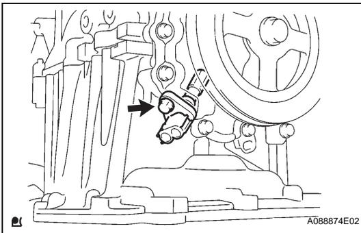
**38. INSTALL CRANKSHAFT POSITION SENSOR**
