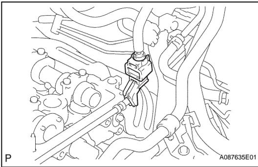
(b) Install the fuel pipe clamp.
