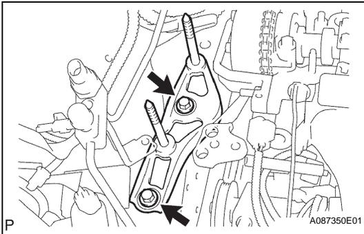
**30. REMOVE ENGINE MOUNTING SPACER**
