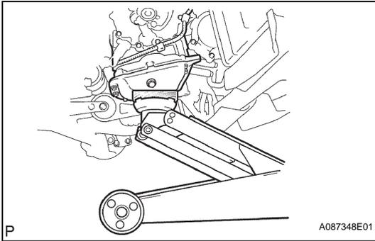
**29. REMOVE ENGINE MOUNTING INSULATOR RH**
