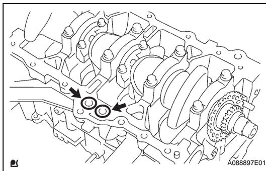
(c) Install 2 new O-rings onto the cylinder block.
