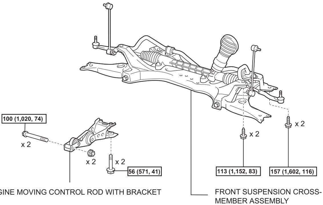
ENGINE MOVING CONTROL ROD WITH BRACKET
