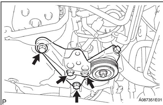
**31. REMOVE ENGINE MOUNTING BRACKET**
