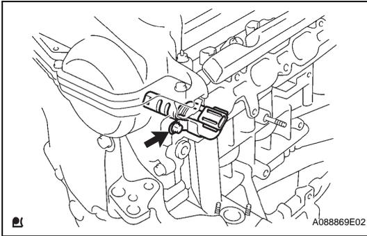
**40. INSTALL CAMSHAFT TIMING OIL CONTROL VALVE ASSEMBLY**
