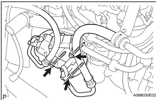
**30. CONNECT COOLER COMPRESSOR WITH MOTOR ASSEMBLY**
