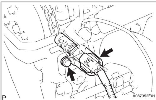
**32. REMOVE CAMSHAFT TIMING OIL CONTROL VALVE ASSEMBLY**
