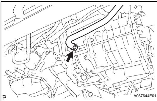
**39. CONNECT NO. 3 INVERTER COOLING HOSE****40. INSTALL NO. 2 RADIATOR ASSEMBLY**
