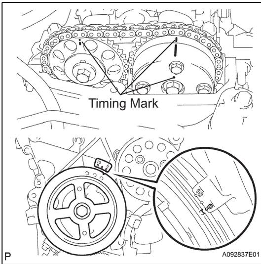
(ae) Turn the crankshaft pulley until its timing notch and timing mark 0 of the chain cover are aligned.
