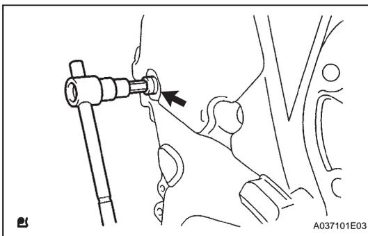
(ah) Using an 8 mm hexagon wrench, install the screw plug.
