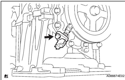
**8. REMOVE CRANKSHAFT POSITION SENSOR**
