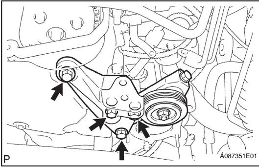
7. **INSTALL ENGINE MOUNTING SPACER**
