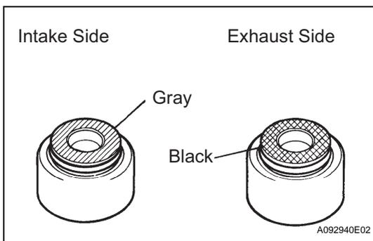
**3. INSTALL VALVE STEM OIL SEAL**
