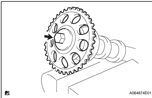
**24. REMOVE CAMSHAFT TIMING SPROCKET**
