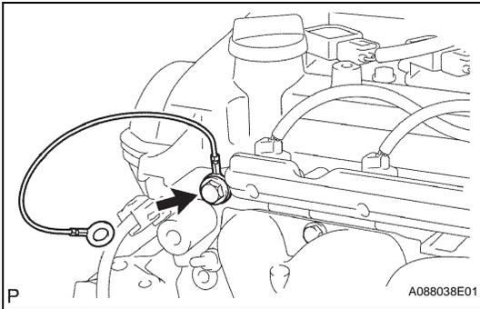
(e) Install the ground cable with the bolt.
