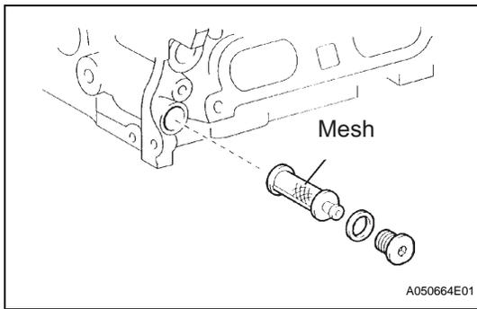
**6. INSTALL OIL CONTROL VALVE FILTER**
