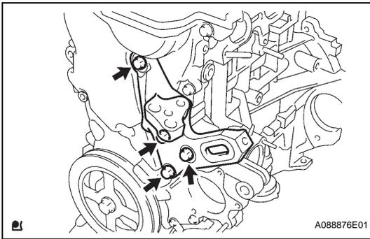
**11. REMOVE ENGINE MOUNTING BRACKET RH**
