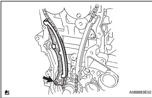
**18. REMOVE CHAIN TENSIONER SLIPPER**
