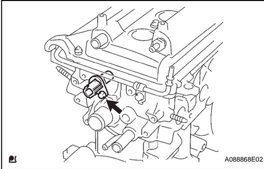
**41. INSTALL CAMSHAFT POSITION SENSOR**
