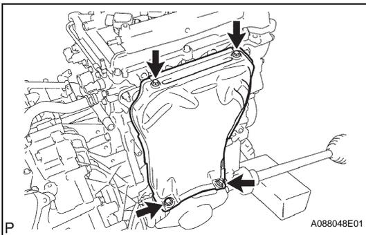
**60. REMOVE EXHAUST MANIFOLD**
