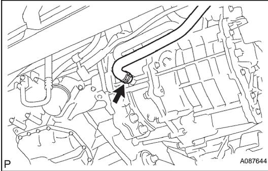
**23. DISCONNECT NO. 3 INVERTER COOLING HOSE**
