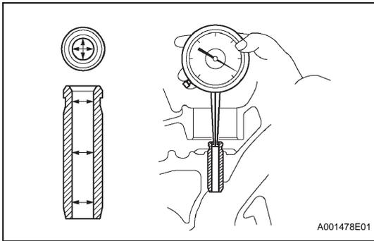
**8. INSPECT VALVE GUIDE BUSH OIL CLEARANCE**
