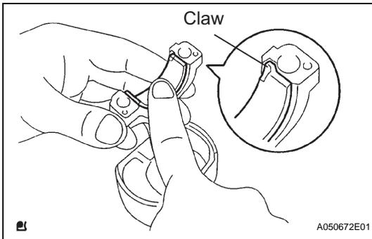
**9. INSTALL CONNECTING ROD BEARING**
