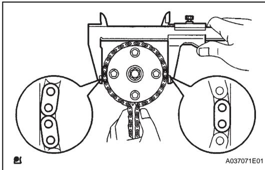
**15. INSPECT CAMSHAFT TIMING GEAR**
