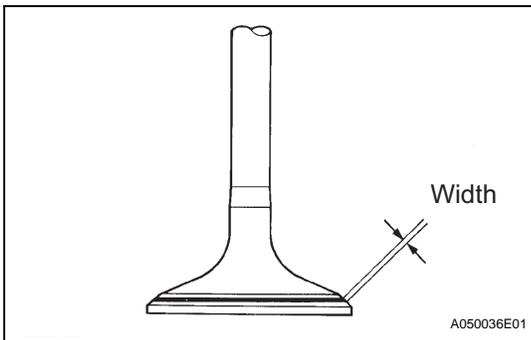
**9. INSPECT INTAKE AND EXHAUST VALVE SEAT**
