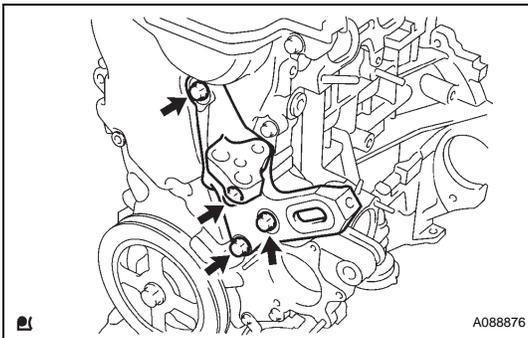
**29. INSTALL ENGINE MOUNTING BRACKET RH**
