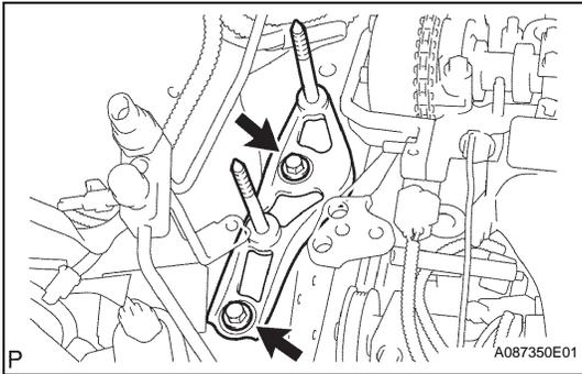
8. **INSTALL ENGINE MOUNTING INSULATOR RH**
