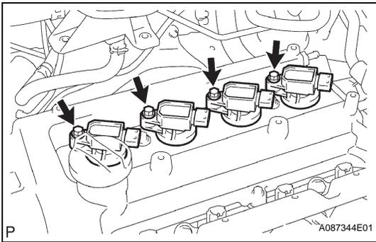
(e) Remove the bolt and ignition coil.
