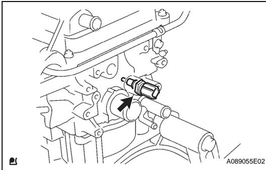
**62. REMOVE ENGINE COOLANT TEMPERATURE SENSOR**
