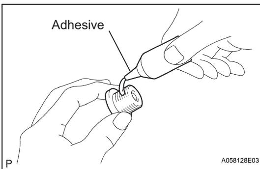
(ag) Apply seal packing to 2 or 3 threads of the screw plug end.
