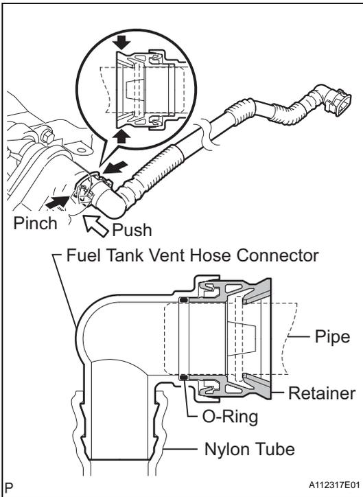
(i) Pinch the retainer and pull out the fuel tank vent connector with the fuel tank vent hose connector pushed to the fuel tank vent hose side to disconnect the fuel tank vent hose from the trap canister with pump module.
