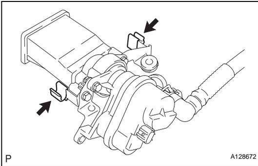
(h) Remove the 2 clamps from the trap canister with pump module.
