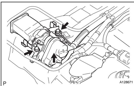
12. REMOVE TRAP CANISTER WITH PUMP MODULE
