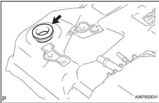
(g) Remove the gasket from the fuel tank.
