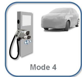
Figure 3d – Mode 4 Charging
