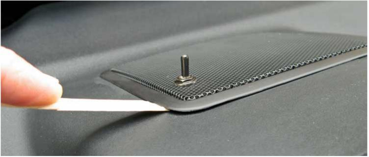
When the edge nearest you is popped up (you can see the front two clips here, there are also two more clips, one on each side) - just pull the whole speaker out and disconnect the white harness. The edge toward the windshield will come out after the front is up - do NOT try to pry the rear edge out, as those clips are different.
