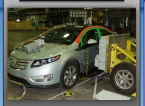
50 kph IIHS Side Impact Deformable Barrier
