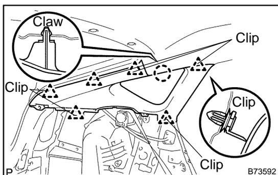
**38. REMOVE ROOF SIDE GARNISH ASSY INNER LH**
