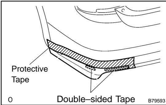
(c) Put protective tape under the rear bumper.
