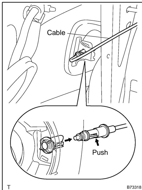
(b) Disengage the claw and remove the cable.
