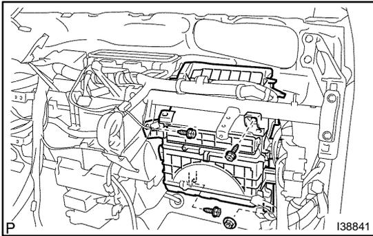
(c) Remove the 3 screws the nut and then the blower assy.
