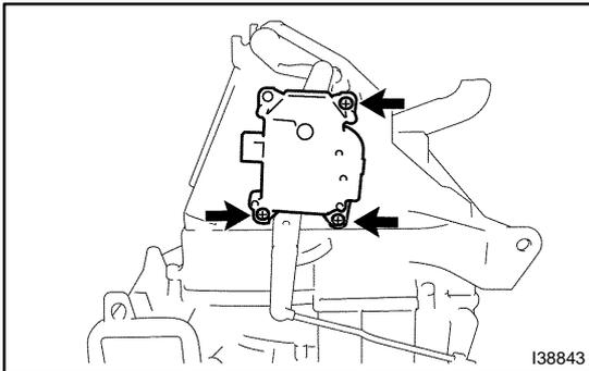
**9. REMOVE AIR INLET SERVOMOTER**
