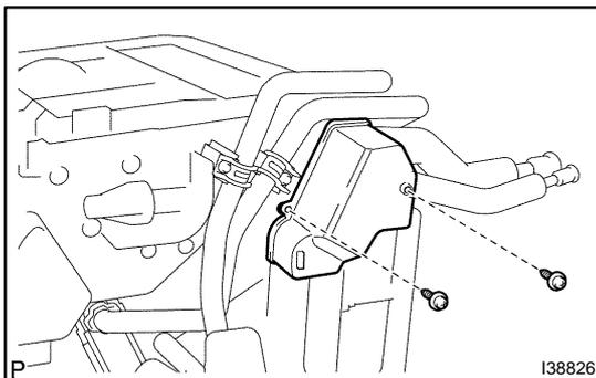
**25. REMOVE AIR CONDITIONING TUBE & ACCESSORY ASSY**
