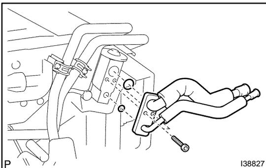
**34. INSTALL AIR CONDITIONING TUBE & ACCESSORY ASSY**
