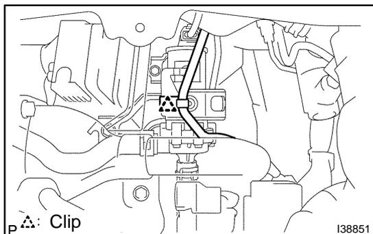
1. **DISCONNECT HEATER WATER HOSE C**
