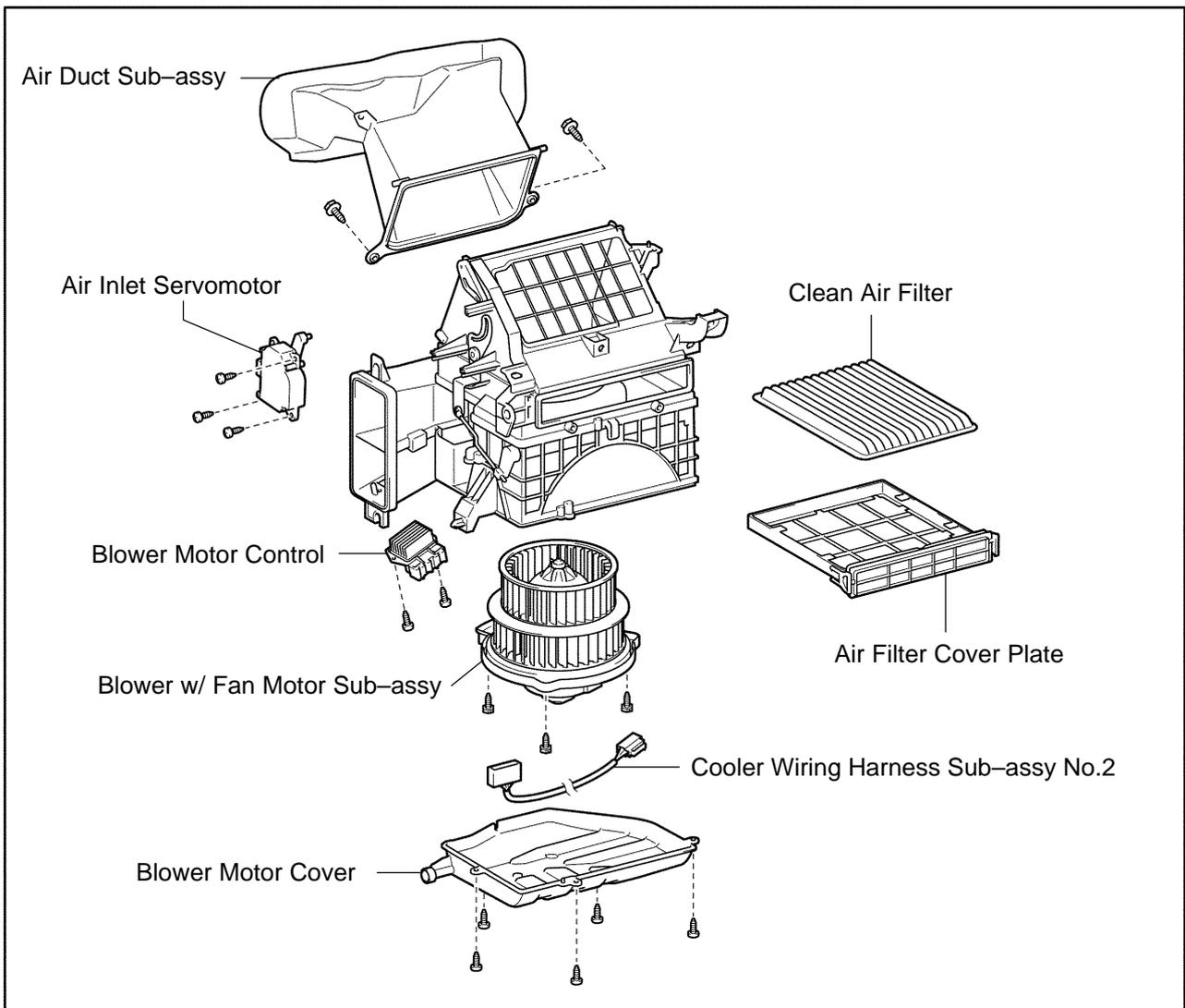
★ : Use repair screw (parts No.90159-70003) if the screw removed before cannot be tightened.
