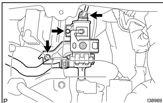
2. **REMOVE HEATER WATER PUMP ASSY**
