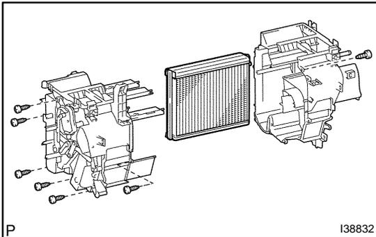
**30. REMOVE COOLER EVAPORATOR SUB-ASSY NO.1**
