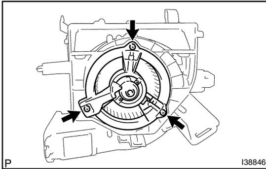
**12. REMOVE BLOWER W/FAN MOTOR SUB-ASSY**
