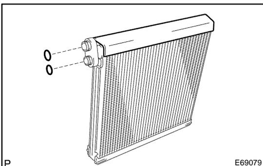
**32. INSTALL COOLER EVAPORATOR SUB-ASSY NO.1**
