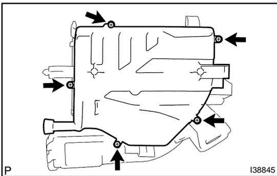
**11. REMOVE COOLER WIRING HARNESS SUB-ASSY NO.2**
