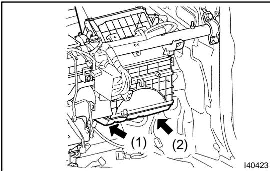
**38. FULLY TIGHTEN AIR CONDITIONER UNIT ASSY**
