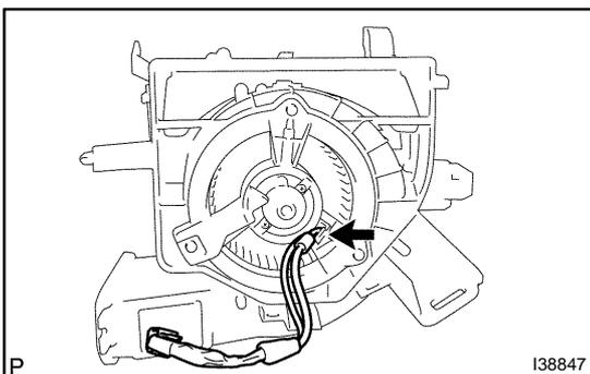
(b) Remove the cooler wiring harness sub-assy No.2 from the blower w/fan motor sub-assy.
