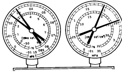
NOTE : These gauge indications occur when the refrigeration system opens and the refrigerant is charged without vacuum purging.
