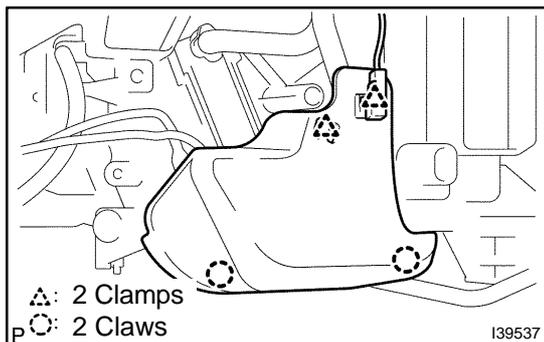
**27. REMOVE HEATER RADIATOR UNIT SUB-ASSY**
