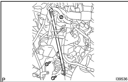
**37. INSTALL INSTRUMENT PANEL BRACE SUB-ASSY NO.1**
