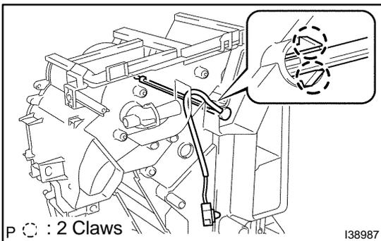
**31. REMOVE EVAPORATOR TEMPERAURE SENSOR**
