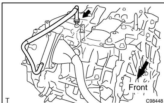
**27. INSTALL INVERTER COOLING HOSE NO.6**
