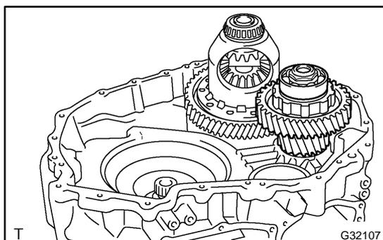
**40. INSTALL DIFFERENTIAL DRIVE PINION**
