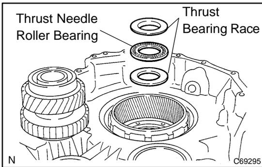
**7. REMOVE PLANETARY RING GEAR**
