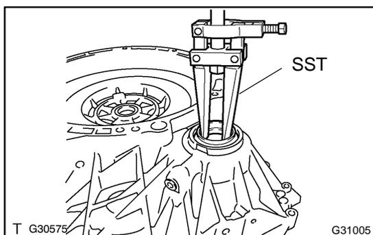
**31. REMOVE HYBRID VEHICLE TRANSAXLE ASSY TYPE T OIL SEAL**
