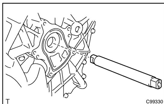
(b) Remove the oil pump drive shaft.
