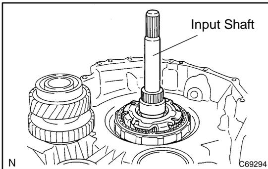
**6. REMOVE INPUT SHAFT ASSY**
