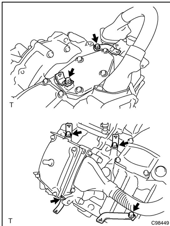
**26. INSTALL ENGINE MOUNTING BRACKET NO.3**
