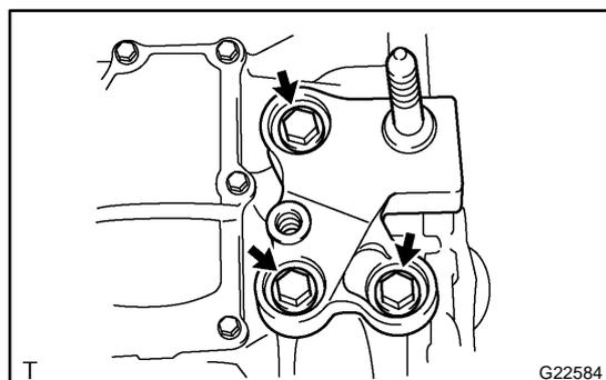
**65. INSTALL ENGINE MOUNTING BRACKET NO.3**
