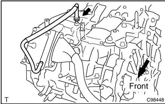
**24. REMOVE INVERTER COOLING HOSE NO.6**
