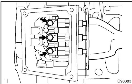
(c) Install the generator cable (terminals) with the 3 bolts.
