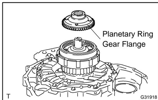
(10) Install the planetary ring gear flange.
