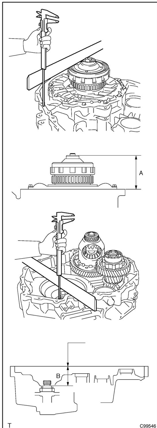
(11) Using a straight edge and vernier calipers, measure dimension A as shown in the illustration.
