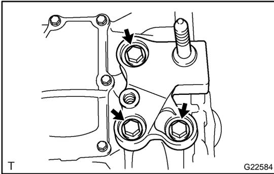
**12. REMOVE ENGINE MOUNTING BRACKET NO.3**
