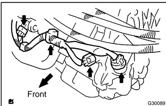
(f) Connect the clamp and the 3 connectors shown in the illustration.
