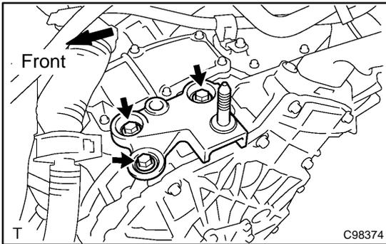
**25. REMOVE ENGINE MOUNTING BRACKET NO.3**
