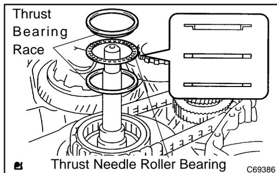
**45. INSTALL THRUST BEARING RACE NO.2**
