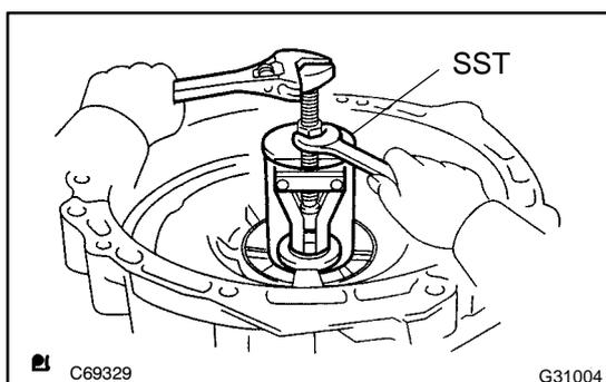
**30. REMOVE HYBRID VEHICLE TRANSAXLE ASSY TYPE T OIL SEAL**
