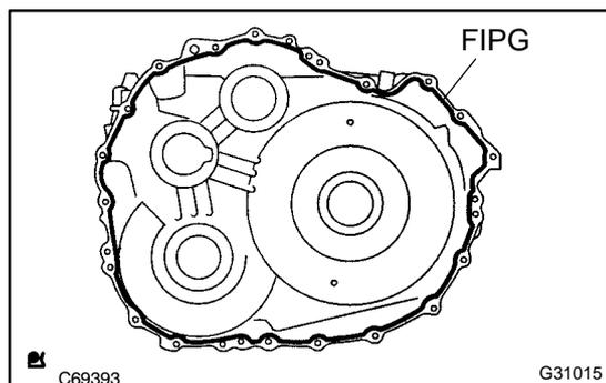
**47. INSTALL HYBRID VEHICLE GENERATOR ASSY**
