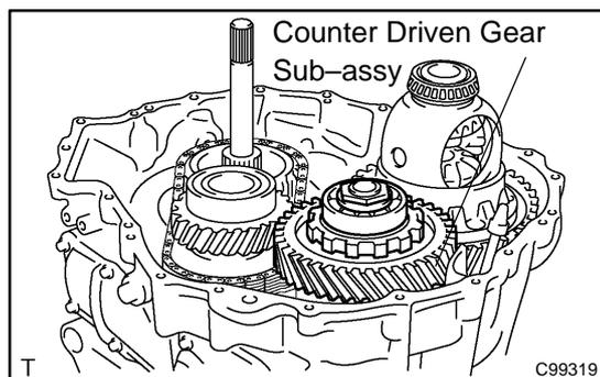
**3. REMOVE DIFFERENTIAL DRIVE PINION**
