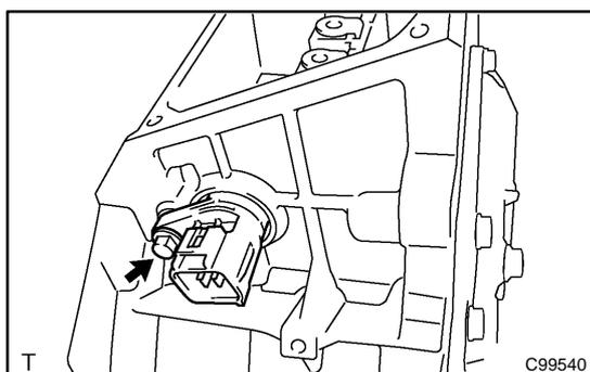
**28. REMOVE GENERATOR MOTOR REVOLUTION SENSOR WIRING HARNESS CONNECTOR**
