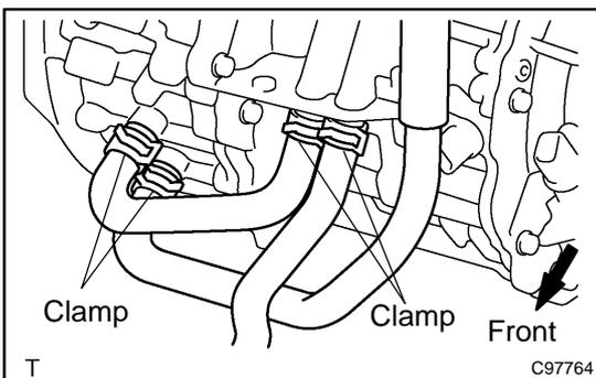
**15. SEPARATE INVERTER COOLING HOSE NO.4**
