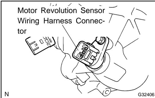
**13. REMOVE MOTOR REVOLUTION SENSOR WIRING HARNESS CONNECTOR**
