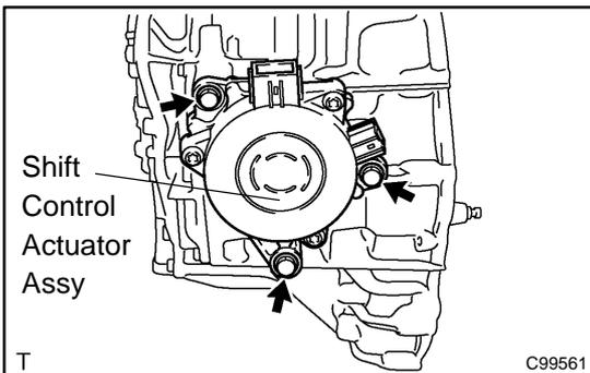
**15. REMOVE SHIFT CONTROL ACTUATOR ASSY**
