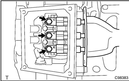
(b) Remove the 3 bolts and generator cable.
