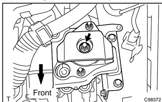
**22. SEPARATE ENGINE MOUNTING BRACKET NO.3**
