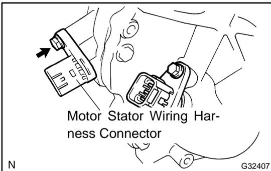
**14. REMOVE MOTOR STATOR WIRING HARNESS CONNECTOR**
