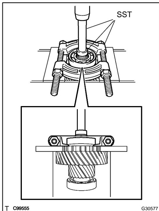
(c) Using SST and a press, remove the bearing from the differential driver pinion.
