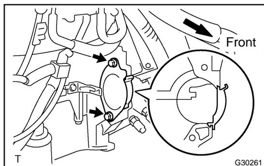
**23. REMOVE HYBRID VEHICLE TRANSAXLE ASSY**
