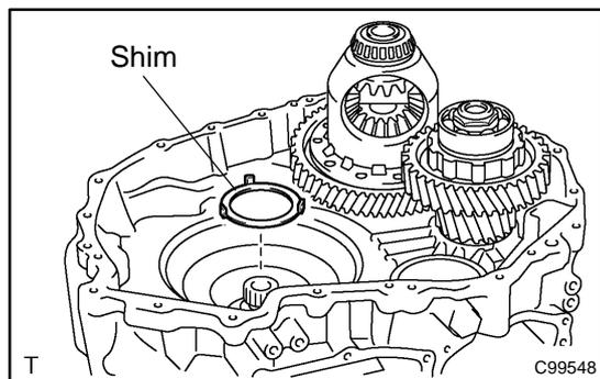
**42. INSTALL INPUT SHAFT ASSY**
