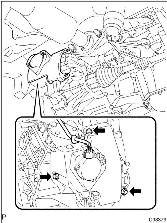
(c) Install the transmission case cover to the hybrid vehicle transaxle using the 3 bolts.
