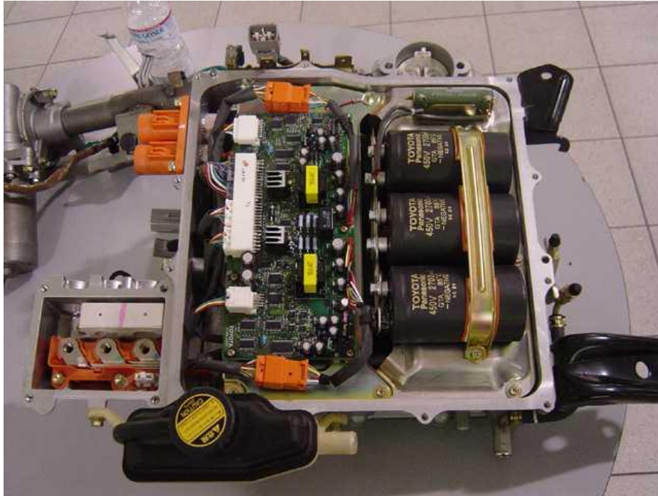
High voltage unit of the HSD
