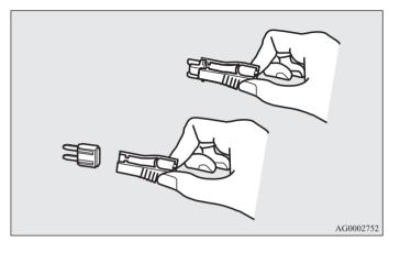
4. Use the fuse location diagrams and their corresponding tables, to check the fuse that is related to the problem. If the fuse is not blown, something else must be causing the problem.
