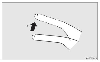
1- Pull the lever up without pushing the button at the end of hand grip.
