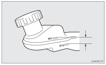
The brake fluid level falls slightly with wear of the brake pads, but this does not indicate any abnormality.
