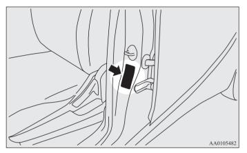
This placard shows the maximum number of occupants permitted to ride in your vehicle as well as "the combined weight of occupants and cargo" (C), which is called the vehicle capacity weight. This placard also tells you the size and recommended inflation pressure for the original equipment tires on your vehicle. For more information, refer to "Tires" on page 7-18.
