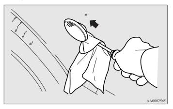
2. Remove the socket and bulb assembly together by turning it counterclockwise.
