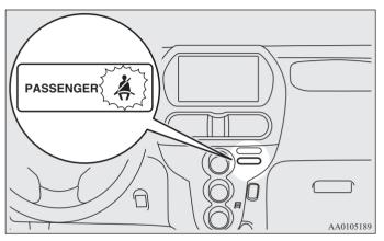
When the electric motor switch is turned to the "ON" position, this indicator normally comes on and goes off a few seconds later.
