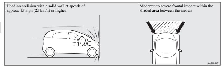
The front airbags are designed to deploy when the vehicle suffers a moderate to severe frontal impact. A typical condition is shown in the illustration to the left.
