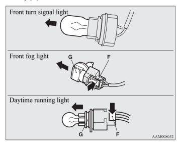
5. To install the bulb, perform the removal steps in reverse.
