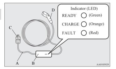
Ready (green), Charge (orange) and Fault (red) indicators are on the control box and they will illuminate/blink in response to the following conditions:
