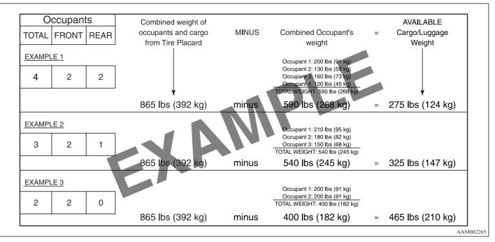
• Under a maximum loaded vehicle condition, gross axle weight ratings (GAWR's) for the front and rear axles must not be exceeded. For further information on GAWR's, vehicle loading, see the "Specifications" section of this manual.
