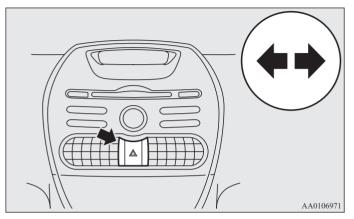
If you press the flasher switch, the front and rear turn signals will flash intermittently, and so will the hazard warning lights. This is an emergency warning system and should not be used when the vehicle is in motion, except for emergencies. If you need to leave your vehicle, the flashers will keep work-
