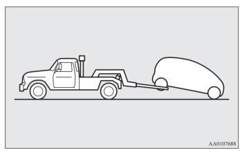
Place the selector lever in the "N" (NEUTRAL) position. Turn the electric motor switch to the "ACC" position and secure the steering wheel in a straight-ahead position with a rope or tiedown strap. Never place the electric motor switch in the "LOCK" or "ON" position when towing.
