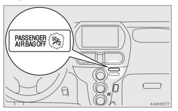
The indicator normally comes on when the electric motor switch is turned to the "ON" position and goes out a few seconds later.
