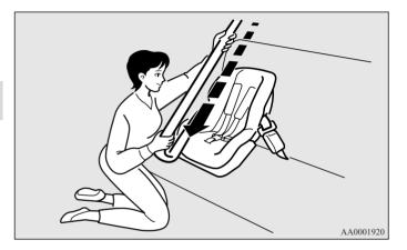
4. After the belt has retracted, tug on it. If the belt is in the ALR function, you will not be able to pull it out. If the webbing can be pulled out from retractor, the ALR function has not been activated and you will need to repeat steps 3 and 4.
