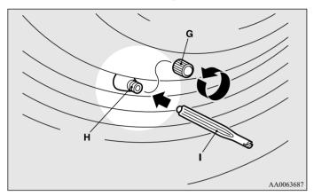
9. Remove the valve insert (J) by turning it counterclockwise using the valve remover (I). Put the removed valve insert in a clean place so it does not get dirty.
