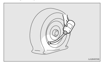
12. After injecting the sealant, pull the hose off the valve, remove any residual sealant from the valve, rim and/or tire.
