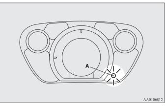
3. The system has entered the armed stage after about 20 seconds, when the theft-alarm indicator flashing becomes slower.
