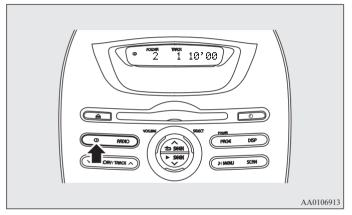
Push the CD button if a disc is already in the CD player. The display shows "READING", then playback begins. The folder number, the track number and the playing time will appear on the display. NOTE
