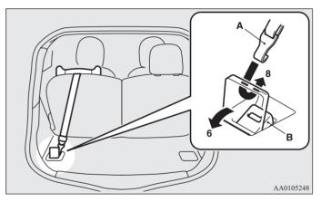
• Child restraint system tether anchors are designed only to withstand loads from correctly fitted child restraint systems. Under no circumstances are they to be used for adult seat belts, harnesses, for attaching other items, or equipment to the vehicle.
