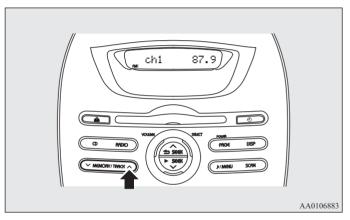
3. To recall a frequency that has been saved in memory, press the MEMORY button briefly for no longer than about 1 second.
