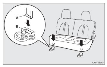
5. After installing the seat cushion, shake it lightly to confirm that it is properly fixed in position.
