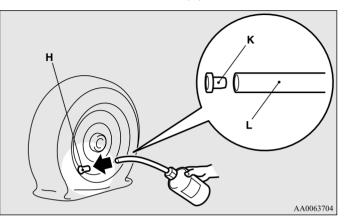
11. Holding the sealant bottle upside-down, squeeze it again and again to inject all of the sealant into the tire.
