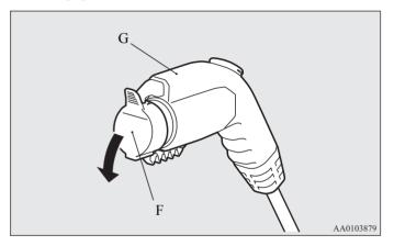
8. Connect the regular charge connector until a click is heard without pressing the button (H).
