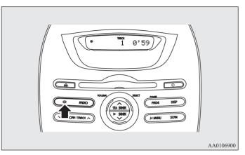
Push the CD button if a disc is already in the CD player. The audio system will enter CD mode and start playback. The track number and the playing time will appear on the display. The tracks in the disc will be played consecutively and continuously.
