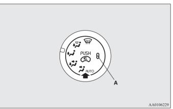
If high cooling performance is desired, or, if the outside air is dusty or contaminated in some way, use the recirculation position. Switch to the outside air position every now and then to keep the windows from fogging up.
