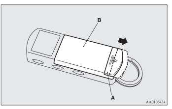
3. By moving the battery cover (B) in the arrow direction, tabs (C) on the battery cover will come out and the battery cover can be removed.
