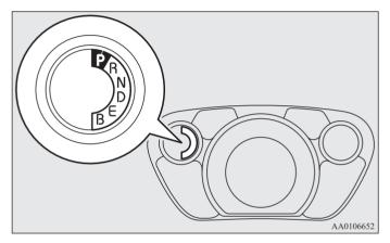
When the selector lever position indicator flashes while you are driving, there could be a malfunction in the transmission.
