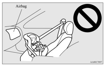
• FRONT-FACING CHILD RESTRAINT SYS-TEMS should be used in the rear seat whenever possible. If they must be used in the front passenger seat, move the seat to the most rearward position and make sure the child stays in the child restraint system, properly restrained. Failure to follow these instructions could result in serious injury or death to the child.
