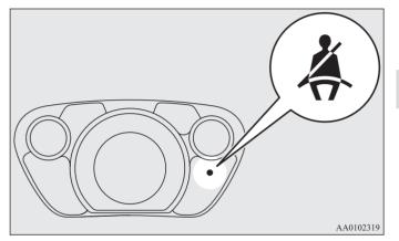
If the electric motor switch is turned to the "ON" position without the driver's seat belt being fastened, a warning light will come on, and a tone will sound for approximately 6 seconds to remind you to fasten your seat belt.
