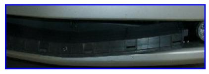
Rotate the grille face down to pull it out.
