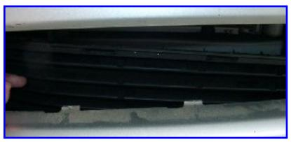
Once all the tabs are free, push the grille into the opening. You might have to move it around a bit to get it past the edge of the nose opening.
