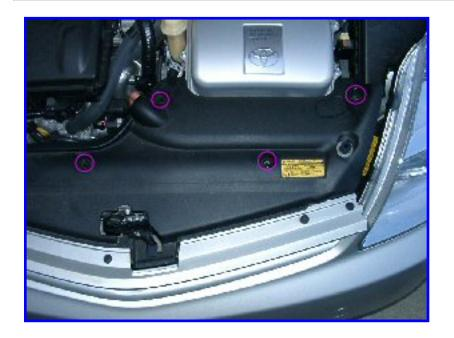
Start by removing the fastening pins circled here...
