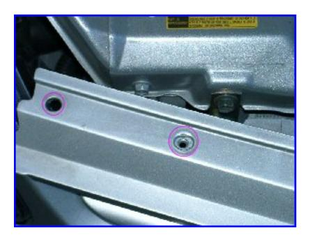
You only need to remove 2 fasteners in front of the horn to make it very easy to access it. The circle on the left is for a push-pin style, simply lever the center of the pin up with a flatblade screwdriver, and pull the pin out. The circle on the right is for a hood bumper, just use a Philips screwdriver to remove it.
