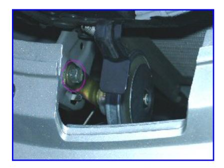
Once all the pins are out, simply lift the black trim panel up and set it aside. Directly under the hood latch, you will see the easiest horn to replace (aftermarket horn already installed). Simply remove the circled bolt, while holding on to the horn, and lift it up through the latch opening, then disconnect the single wire attached to it.
