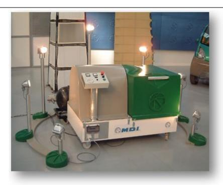
The MDI technology is applicable to a wide range of **Generator** powered by compressed air or dual energy engines. Various kinds of generator can be implemented:
