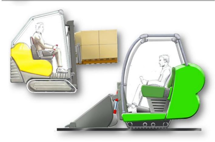
A range of tow tractors and forklift tractors is part of the MDI licensed products. A prototype tractor capable to pull 5 tons was produced and tested. The development of these types of products will be scheduled as opportunities arise.
