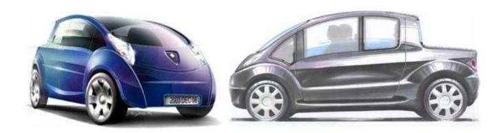
It will come in numerous versions, thanks to a modular concept that allows producing multiple models using an identical body-molding base: pick-up — monospace — multi volume saloon — station wagon — small van — taxi...
