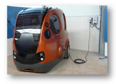
Two modes of filling the Compressed Air are available on the vehicle. A total of the Air tank can be achieved within 2 minutes on an Air station or within 3h30 to 4 hours on an electric plug. The electrical connector is concealed behind the 'AIR' Logo plate on the left flank and the connection to the Air Supply (from an 'Air Station') is concealed behind the 'AIR' Logo plate on the right.
