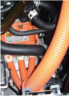
*High-Voltage Cable Connection to Motor*
