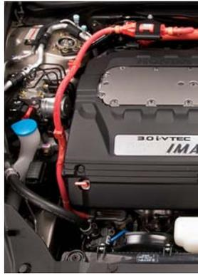
*High-Voltage Cable to Accord AC Compressor*
