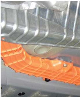
*Electrical shield bolted to undercarriage*
