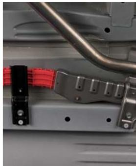
*Thermal shield near hot exhaust*
