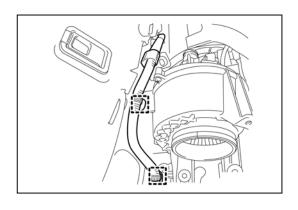
(3) Remove the 2 bolts, nut and battery cooling blower assembly.
