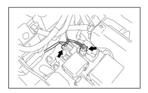
(3) Remove the 3 nuts and hybrid battery junction block.
