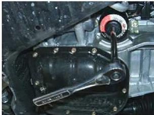
**Center the drainpan under the filter.** Press the wrench onto the end of the filter, break it loose, then wiggle the wrench off of the filter. Then unscrew the filter by hand. Some oil will spill out just as the filter gasket clears the filter block, so be ready for it. Once the filter is off, be careful to keep the filter upright, as it is full of dirty oil. Place it over your drainpan and turn it over to drain.
