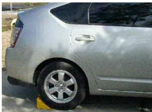
Step 1 if using a jack - place the wheel chocks behind the rear wheels and **set the Parking Brake**. If using ramps, drive up onto the ramps, **set the Parking Brake**, then place the wheel chocks.
