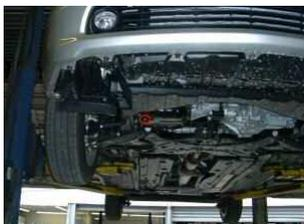
To help locate the oilpan/filter, here's a view up on a lift, showing the location of the oil drainplug.
