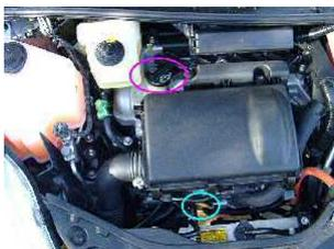
Find the oil cap, shown here circled in pink (the dipstick handle is circled in blue). Here's a [closeup](#).
