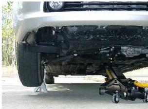
If you are more experienced with cars, are using jackstands, and will be using the [#2 method of leveling the car to check the oil level](#), crack the lugnuts loose for both front wheels before jacking the car up (to make rotating the tires much easier).
