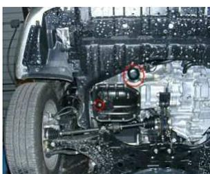
Here's a view directly under the car, the drainplug and oil filter are circled. If you need further pics, try the [diagonal underside view](#) and the [driver's side view](#).
