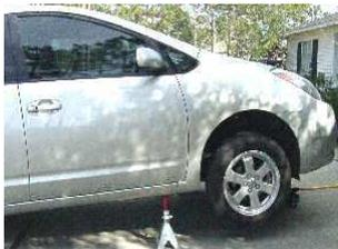
My jackstand placement. If you are using a jack/jackstands, **DO NOT get under the car before putting the jackstands into place and lowering the jack until the jackstands are taking the full weight of the car without shifting**. Use some cardboard between the jackstands and body to protect the body.
