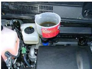
**Use a funnel to fill the car** - the oil cap is somewhat buried, and if you just try pouring the oil into it, you risk pouring oil all over the valvecover. The funnel shown was bought at Walmart for about \$3, includes a long clear hose for the end, and the blue end you see sticking into the valvecover is an on/off switch.
