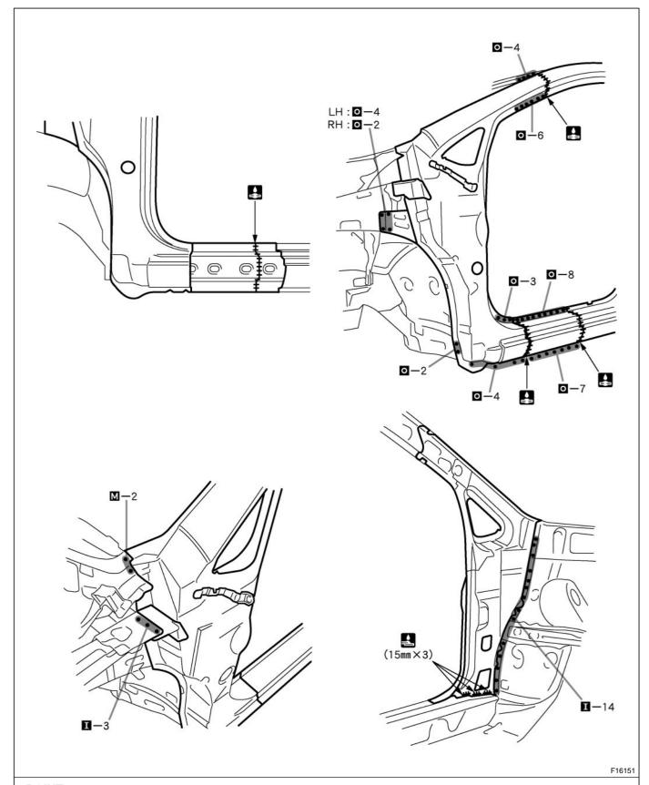
1 Inspect the fitting of the front door, front fender and windshield glass, etc., before welding, since this affects the appearance of the finish.
