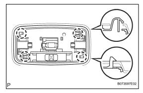
(b) Using a screwdriver, detach the 4 claws and remove the room light.
